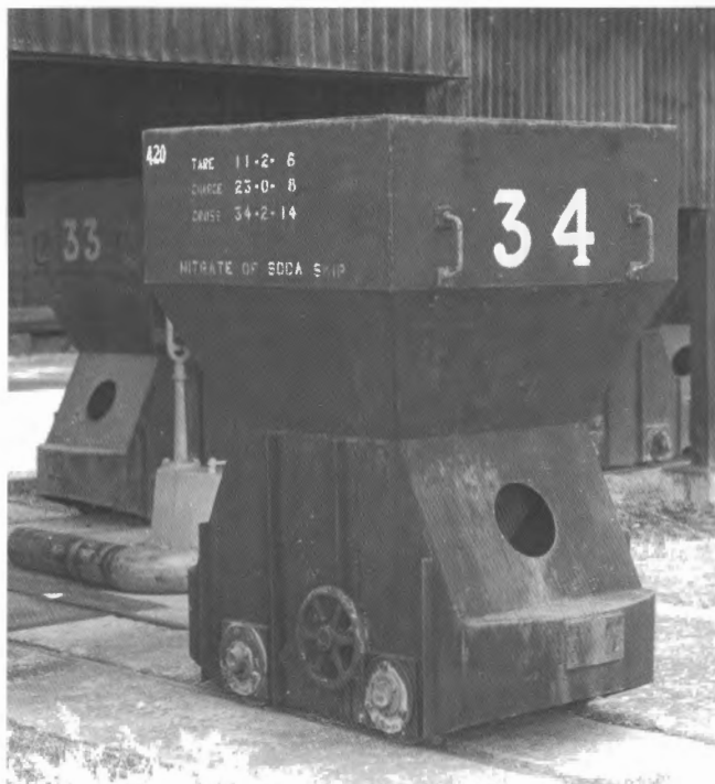
A sodium nitrate skip truck standing outside the skip truck shelter, Acid Section, 1972.
