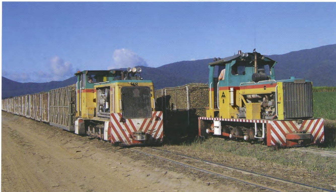
Mulgrave Mill inherited the locomotive fleet of Hambledon Mill and here, on the left, is ex-Hambledon Clyde 0-6-ODH 18 (63-379 of 1963), fitted with a low-level cab for working under the QR bridge at Redlynch. On the right is 0-6-ODH 8 (A1926 of 1958), built for Mulgrave Mill, and consequently fitted with a raised cab. The locomotives are entering the full yard on 21 September 2005, with a 4-wheel 10-tonne bin behind number 18. Photo: John Browning
