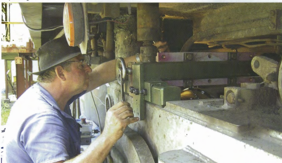
On 29 October 2005, Richmond Vale Railway volunteer John Rodham turns the flanges of ex-BHP Bo-Bo DE centre-cab number 53 on the machine he and fellow volunteers built for the task. Photo: Jeff Muller
