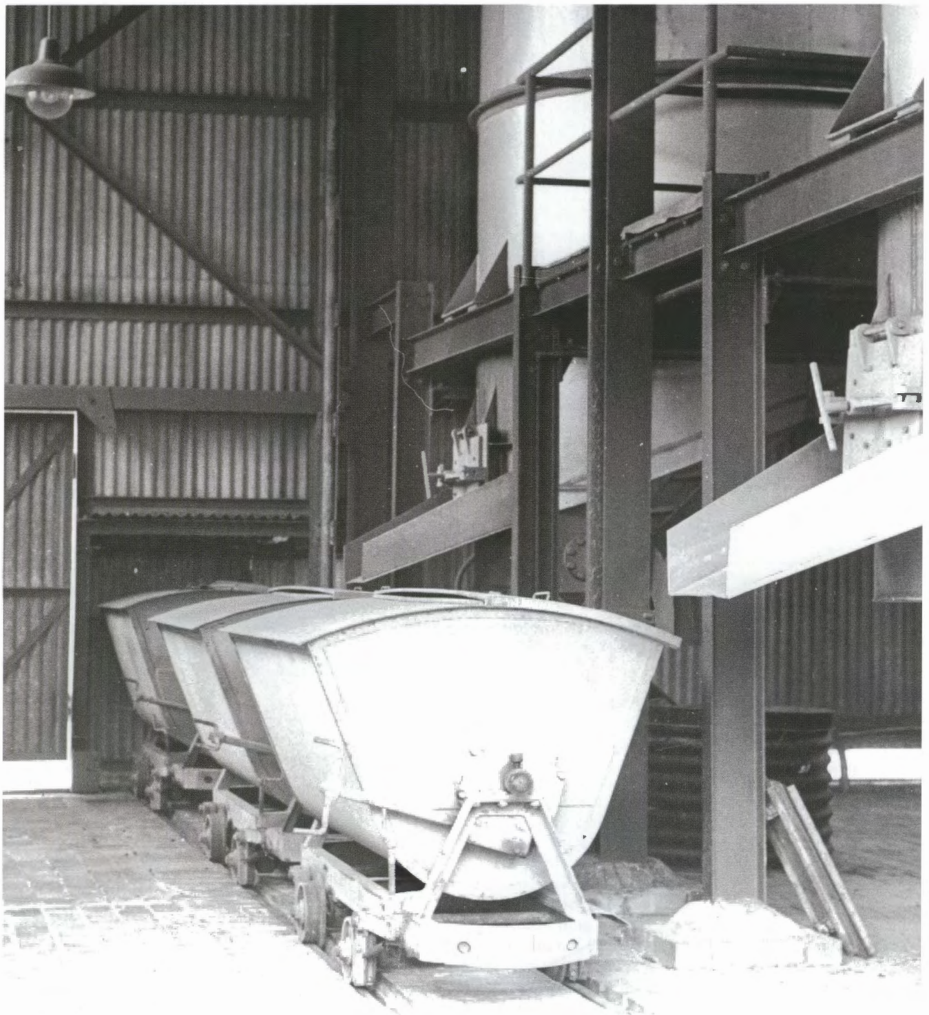
Tipping push trucks, with their water tanks removed, beside the pelleters in the trinitration house, TNT Section, 1972. Photo: Brian Andrews
