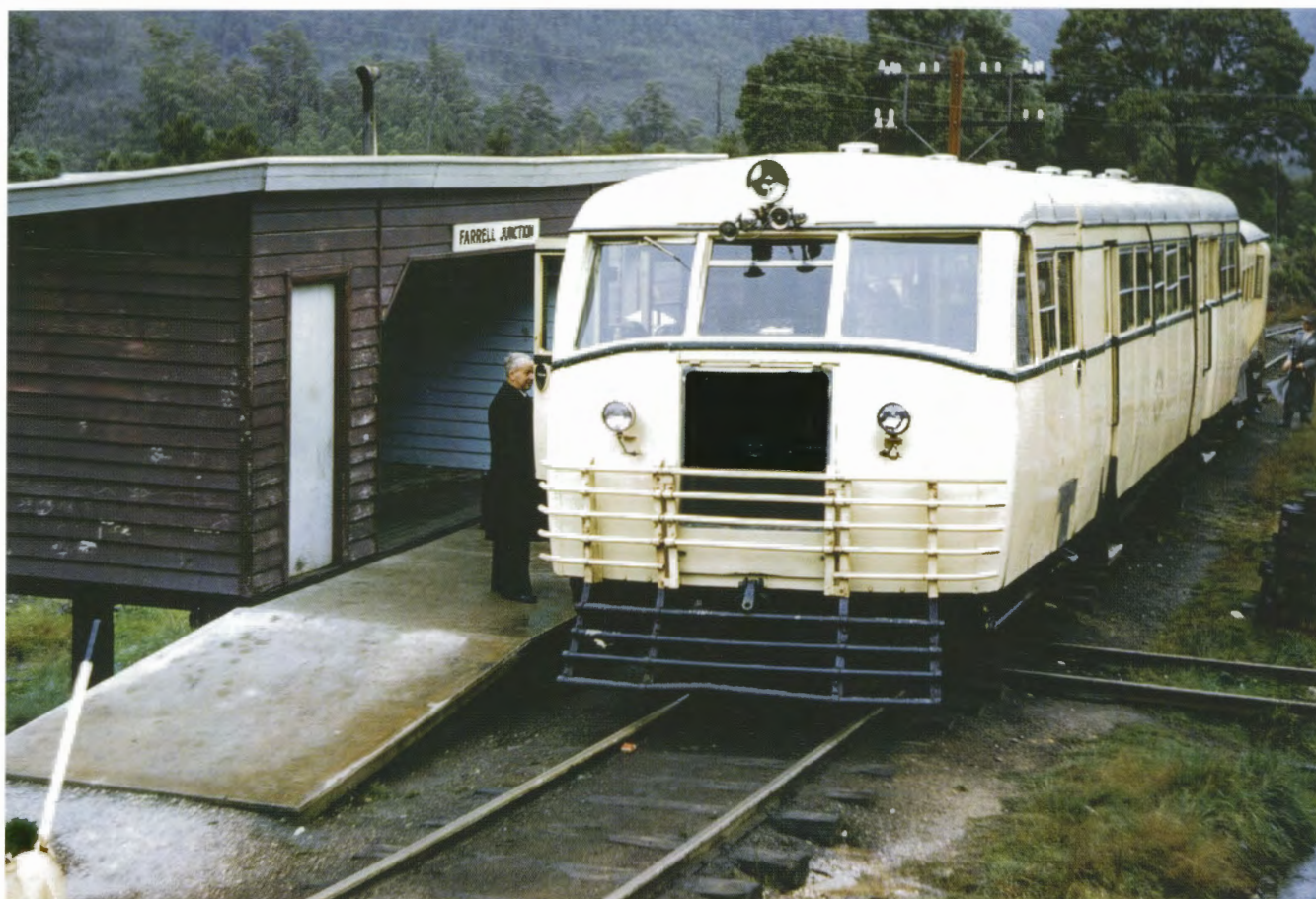
Emu Bay Railway Walker Brothers railmotor WG1, with trailer PT2, at Farrell Junction, where the EBR met the Tullah Tramway. Delivered in April 1940, WG1 was equipped with a 153hp Gardner diesel engine and seated 48 passengers, whilst PT2 could accommodate a further 12.
