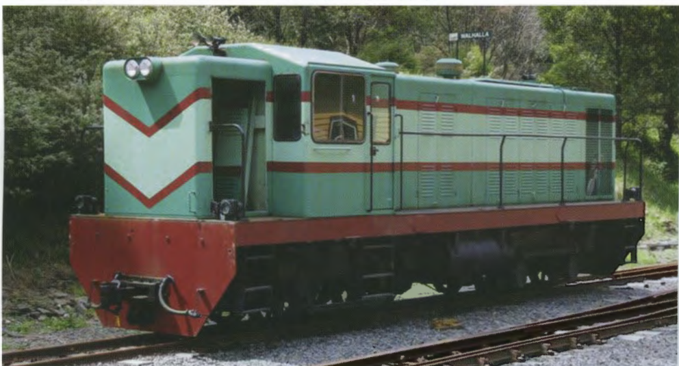
Former Emu Bay Railway B-B DH locomotive No 1001 (Walkers 576 of 1963) pictured in Walhalla yard on the Walhalla Goldfields Railway on 6 November on its new 762mm gauge bogies. Photo: Bill Hanks
