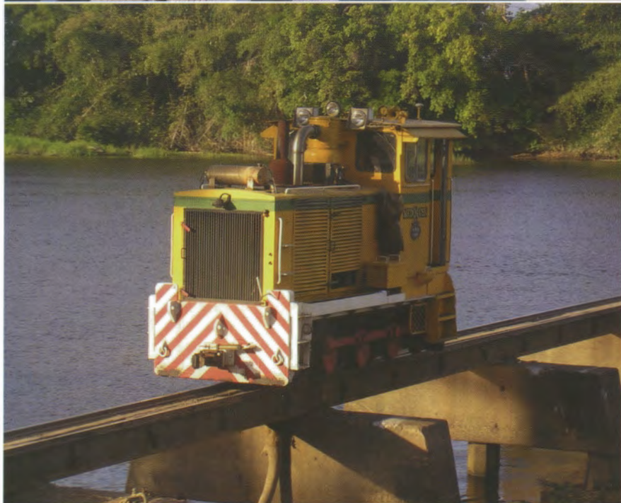
Top: CSR personnel work to install temporary strengthening girders to support the damaged Herbert River bridge at Macknade on 25 November 2006. Photo: Brett Geraghty Above: Driverless EM Baldwin 0-6-0DH 14 (6/2490.1 7.68 of 1968) gingerly crosses the damaged Macknade Herbert River bridge in remote control mode on 25 November 2006. Photo: Brett Geraghty
