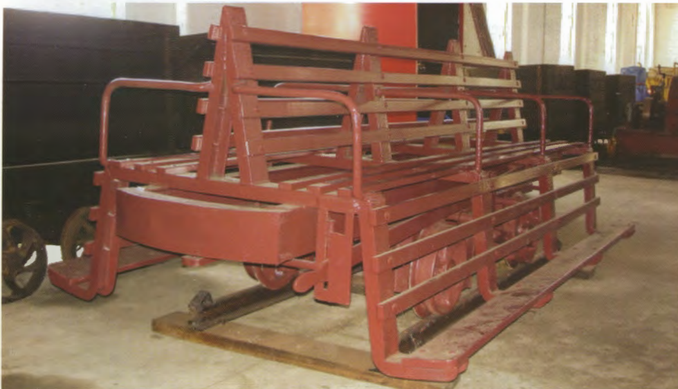
The four-wheel miners' transport car newly restored under a Work for the Dole team supervised by retired coal miners Peter Skinner and Barry Noble. This is one of six recovered from the drift of the Lithgow Valley Colliery in 1996. They were drawn by the endless rope system and had been abandoned in the mine when it closed in 1978. The State Mine Blacksmith Phil Spark made new axle blocks for the restored vehicle. Photo: Ray Christison
