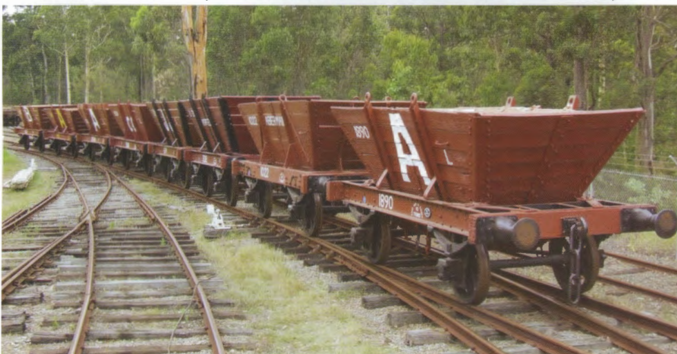
With the restoration of non-air coal hopper wagon B1123, the Richmond Vale Railway reached the halfway mark in its program to restore 16 of these wagons to pristine condition. Graham Black photographed the eight restored wagons in December 2006.
