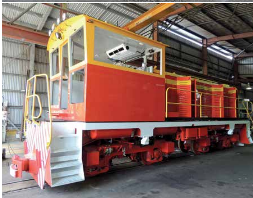
Top: Mulgrave Mill's newly refurbished Com-Eng 0-6-0DH 17 DEERAL (AD1453 of 1962) with its new cab providing enhanced visibility for loco crew, 31 August 2013. Photo: Luke Horniblow
