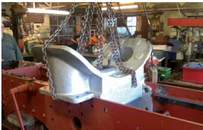
Hunslet 1215 of 1916 has its smokebox saddle casting refitted after repairs. After serving in WW1, 1215 operated at Queensland's Bingera and Invicta mills before being shipped back to England in 2005 for restoration.
