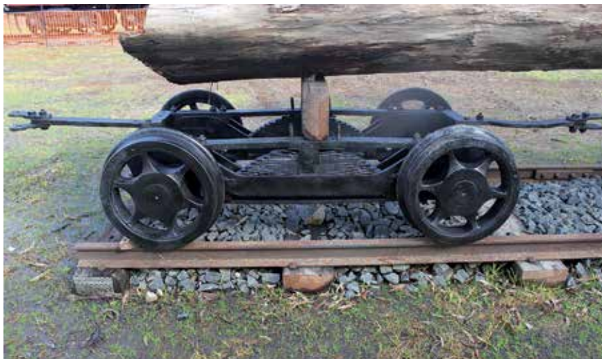
Not instantly recognisable as timber tramway equipment, this 1067mm gauge log bogie forms part of the Noojee & District Historical Societies display at the former VR Noojee railway station site.
