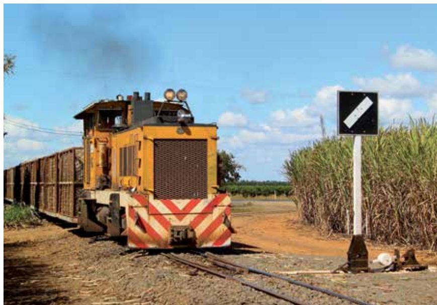
Millaquin Mill's loco E.M. Baldwin B-B DH FAIRYDALE (10048.1 6.82 of 1982) powers a rake of full bins from the Clayon/Alloway area 'over the QR' through the points at South Kalkie Junction (Jimmy Sheehan's) on 25 August. The trailable points at this junction were installed as a part of the flashing light upgrade for Lovers Walk road crossing. Photo: Lincoln Driver
