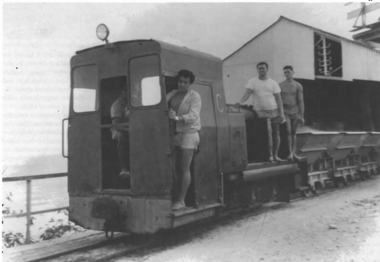
A phosphate train being discharged at the top of the cliff, in 1966. The product is processed as it falls down through the building to the narrow coastal plain. The wagons are 4-wheeled side-tippers built by Decauville. Photo: P Knoepflin
