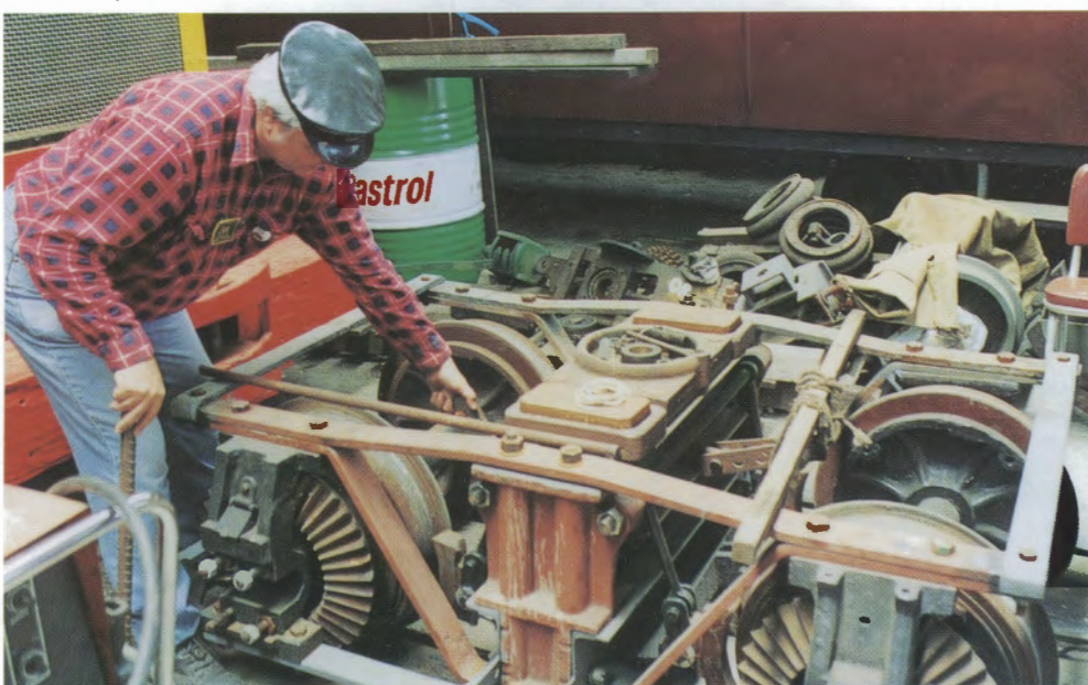
John Garaty points out features of the new Shay bogie during the workshop tour of the ILRMS at Albion Park.
