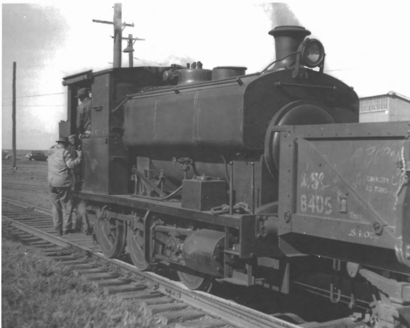
When ER&S required an additional locomotive in 1948, Andrew Barclay supplied another 0-6-0 saddle tank, builder's number 2256, generally similar to No.1. More conventional driving wheels were used, larger diameter cylinders were fitted and it became the second loco to carry No.2. In 1957, the shunter prepares to throw a set of points as No.2 heads into Port Kembla yard sidings. Photo: Ron Preston
