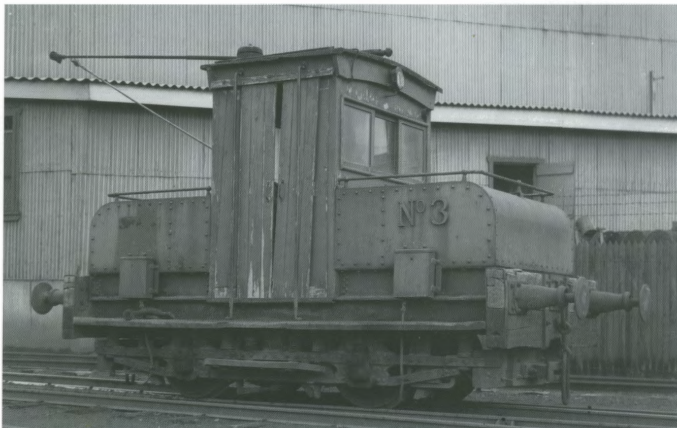
In the transformation that turned the former D class tram to ER&S No.3, only the Peckham four-wheel truck and the trolley pole were visible evidence of its previous existence. Fitted with two types of draugear on its buffer beams, riveted "bull-nose" ends and a tall timber cab, the little electric locomotive was used to move vehicles around the sensitive areas of the smelting plant
