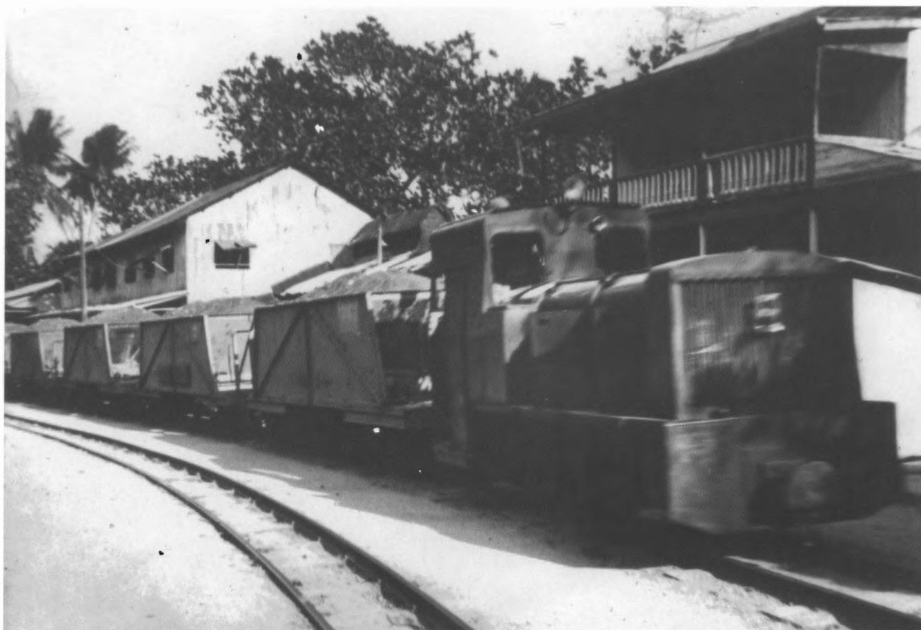
A diesel hauled phosphate train at a similar location in 1966. The locomotive, number B, is an 0-6-0DM built by Billard & Cie. in 1946. Photo: P Knoepflin
