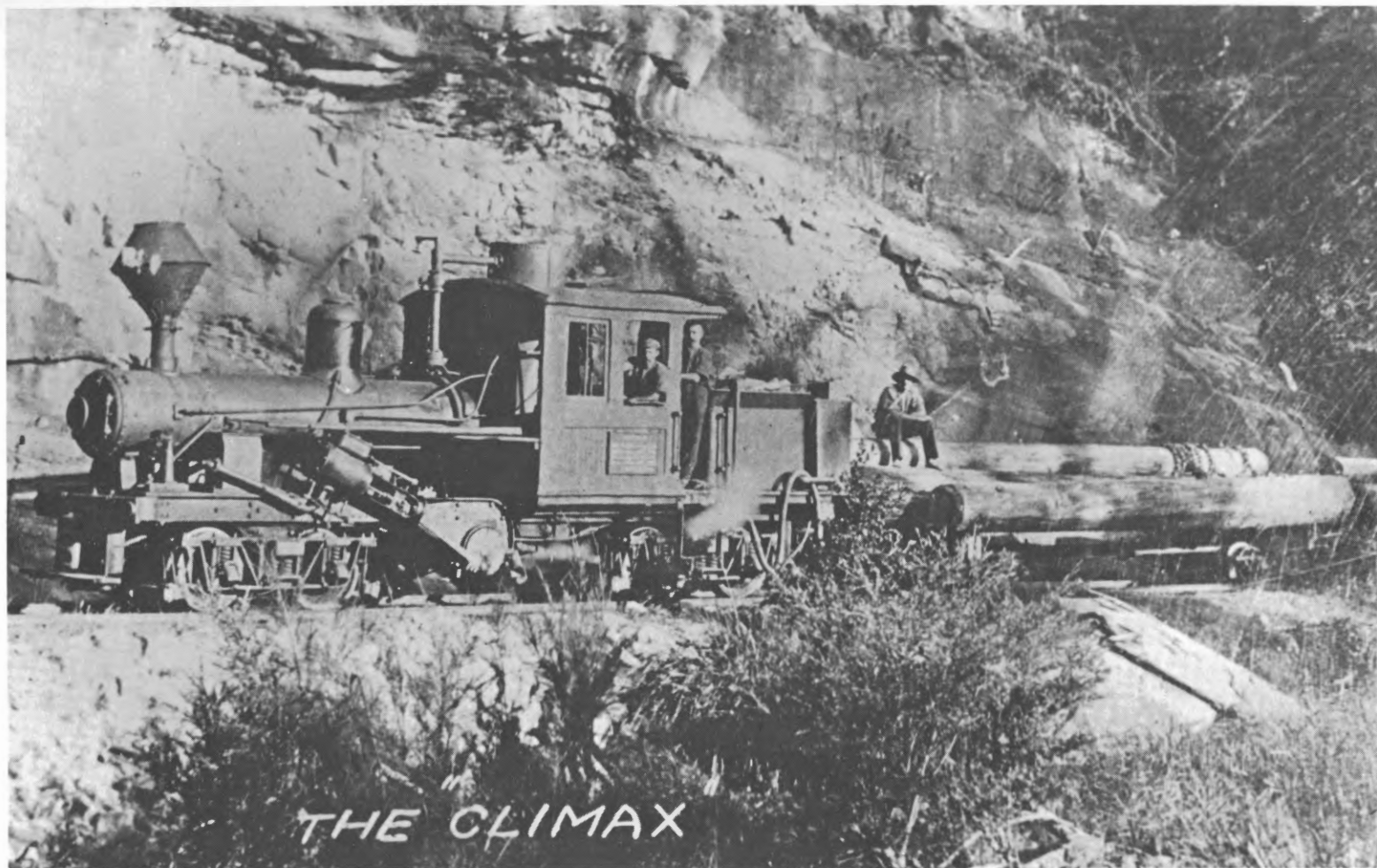
Lahey's Climax locomotive, as rebuilt with extended smokebox, just north of the tunnel. For reproduction, please contact the Society
