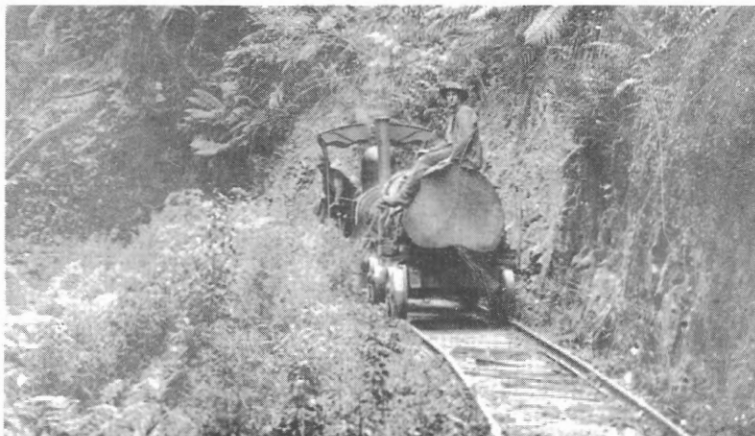
The Beyer Peacock loco bringing in a log to the No. 1 mill. The loco is trailing the load and pushing/coasting down the slight grade. The river is to the left. Photo: Courtesy Don McLaws.
