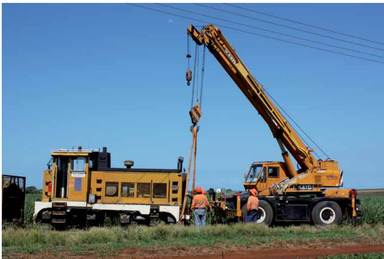
Amid the red soil of the old Qunaba Mill area, Millaquin Mill's EM Baldwin B-B DH CALAVOS (4983.1 1.73 of 1973) came a cropper on 22 November 2012 at Farquhars Road, on what is now known as the Qunaba Line, when a fishplate failed. Help arrived in the shape of a mobile crane and here the early model bogie Baldwin is being rerailed, with ten loaded bins to follow.
