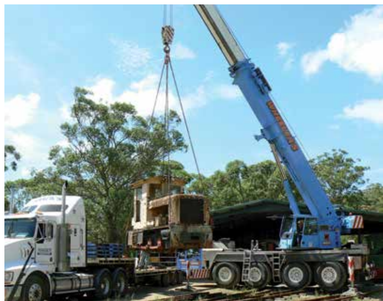
A very large road crane was called in when the loco arrived at Lake Macquarie Light Rail in February 2010. The crane crew certainly knew their job and the impressive capabilities of their computer-controlled crane. Within 30 minutes they had the diesel loco off the semi-trailer and onto a piece of temporary track. Photo: Ian McNeil
