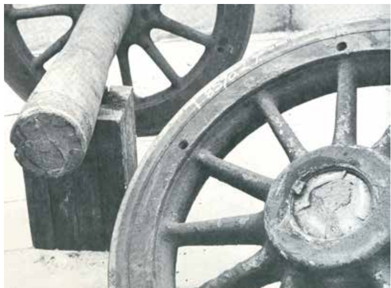
"Snapped in Twain". As stated, axle fractures were rare, but they did occur. Photo: Author's Collection
