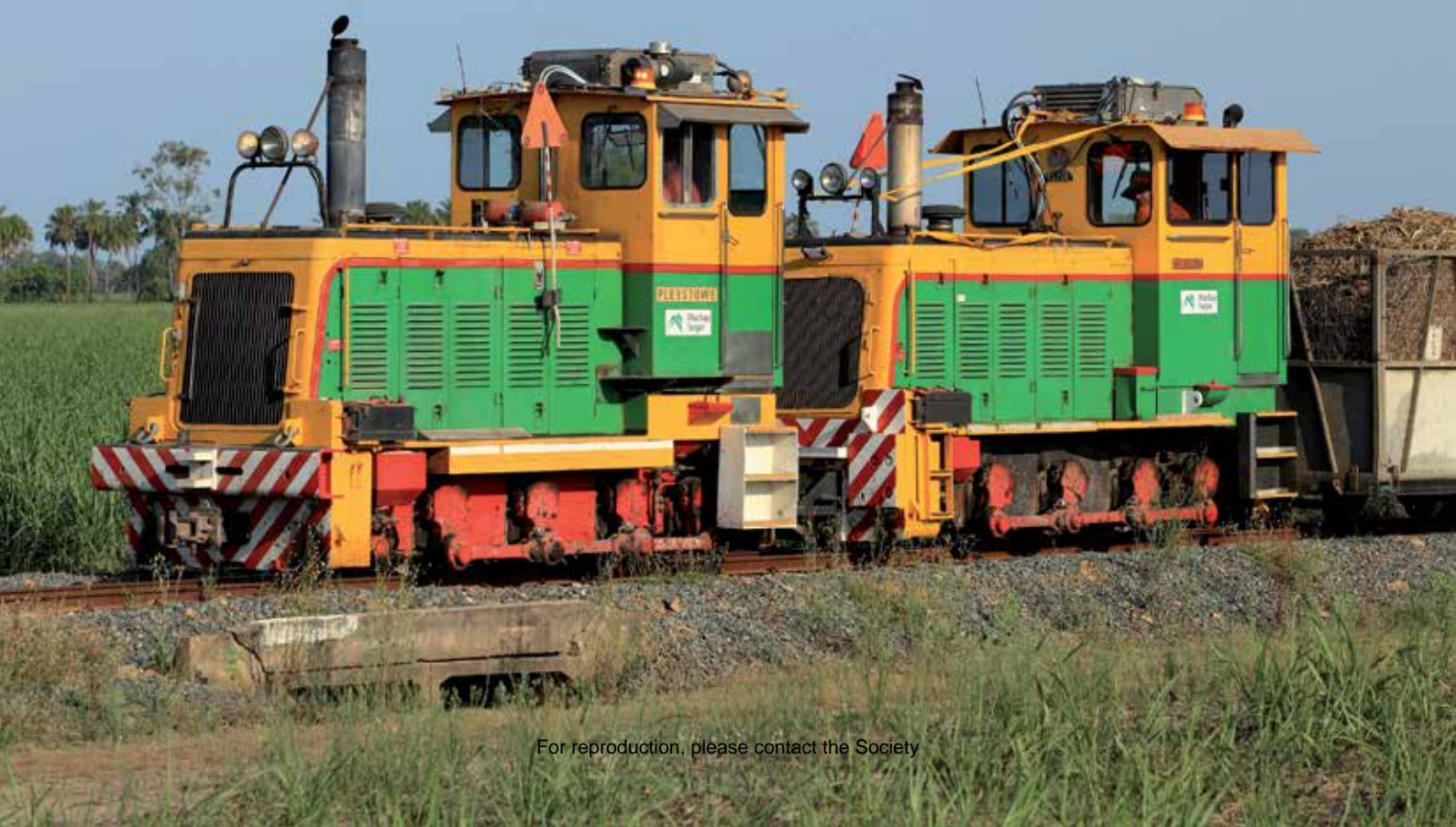
Below: With the normal multi-unit out of action, Clyde 0-6-0DH locomotives PLEYSTOWE (64-321 of 1964) and ST.HELENS (61-234 of 1961) were double-heading on Farleigh Mill's Pioneer Line on 6 December 2012. Could the yellow tape on ST.HELENS be intended as seasonal decoration? Photo: Scott Jesser.
