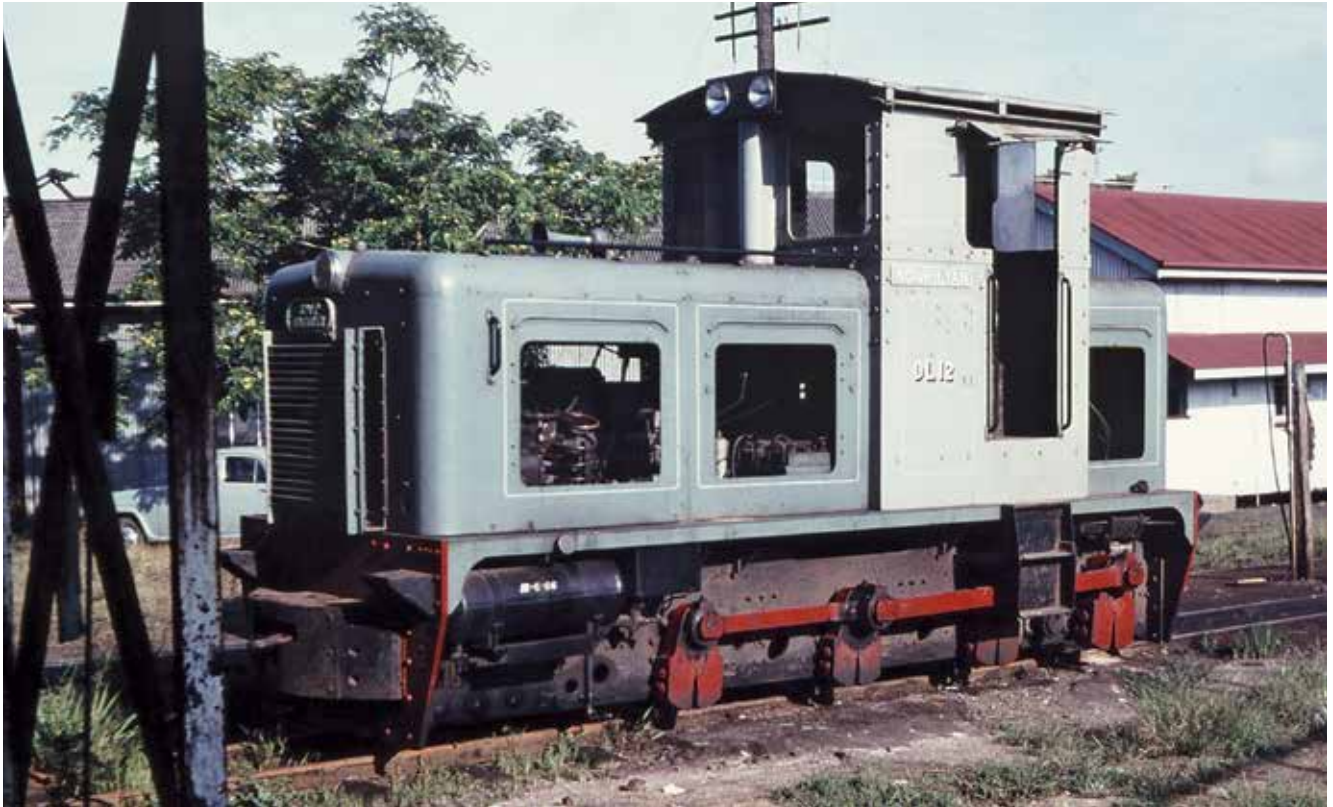
DL12 MOURILYAN at Mourilyan Mill on 15 November 1966. The engine bay door panels have now gone, extra headlights have been added and the tropical Queensland sun has bleached the locomotive's original royal blue paint colour. Photo: Weston Langford
