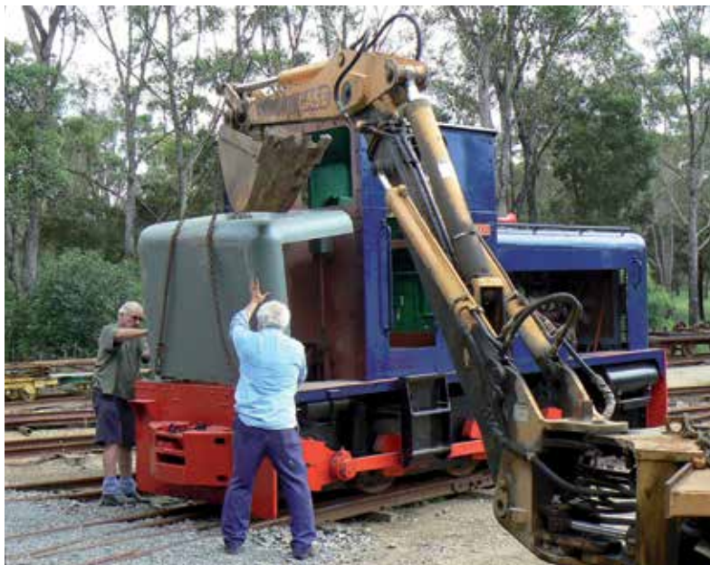
Left: Spray painting the royal blue top coat was undertaken on site. The original colour was able to be recovered from paint preserved under layers of subsequent coats inside the cab. Photo: Ed Boards Right: One of the last components to be reinstalled was an original-profile rear hood fabricated by a Sydney firm specialising in sheet metal bending. This replaced the cut-down hood installed during the latter days of QR ownership in Queensland. Photo: Ian McNeil
