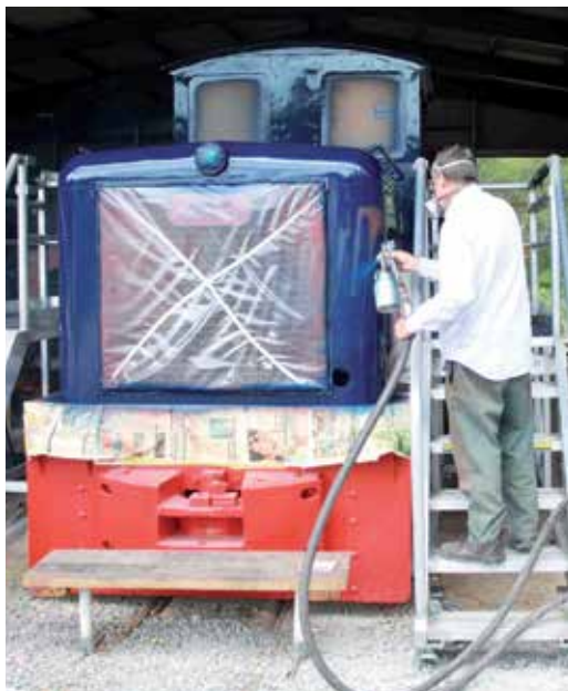
Left: Spray painting the royal blue top coat was undertaken on site. The original colour was able to be recovered from paint preserved under layers of subsequent coats inside the cab. Photo: Ed Boards Right: One of the last components to be reinstalled was an original-profile rear hood fabricated by a Sydney firm specialising in sheet metal bending. This replaced the cut-down hood installed during the latter days of QR ownership in Queensland. Photo: Ian McNeil
