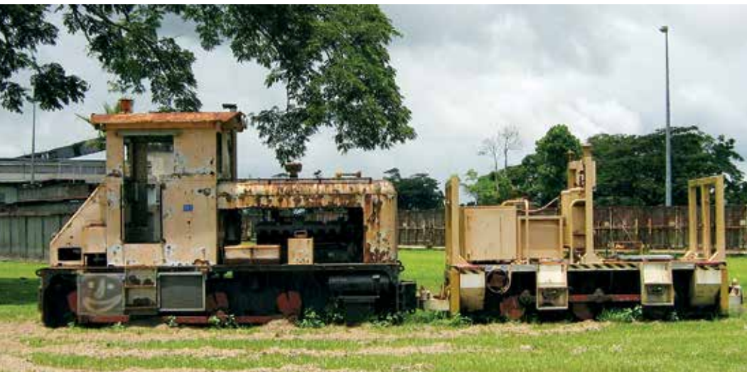
Left: In its final guise, as South Johnstone number 10, the former MOURILYAN sits out of use at the old Mourilyan Mill site on 3 February 2008. The brake wagon alongside began life as a diesel locomotive from the same builder, Drewry 2396 of 1952, ex-South Johnstone Mill number 14. Photo: Chris Hart
