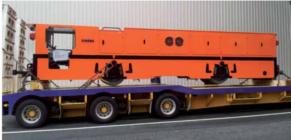
750mm gauge Schöma Model CFL 180 DCL 4wDH locomotive on delivery to the Thiess City East Cable Tunnel site in inner city Surry Hills, Sydney on 28 November 2012. Photo: Robert McFarlane
