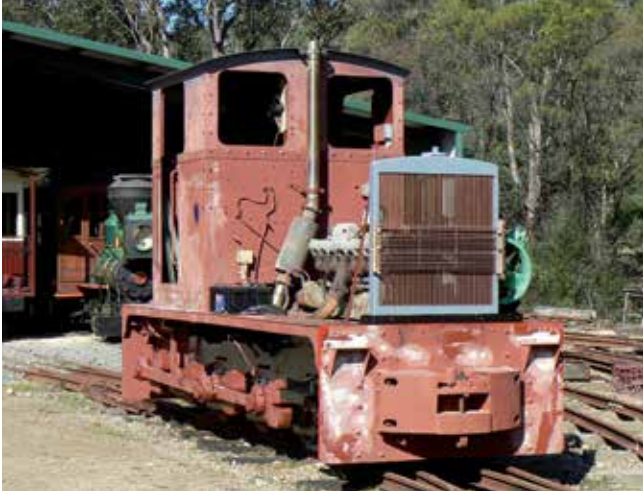
Dismantling and repair began to give way to restoration and reassembly during 2011. Here the chassis and cab components have been repaired, abrasive grit-blasted, primed and reunited. The overhauled radiator and air compressor have been plumbed up, and a pair of heavy-duty batteries installed. Photo: Ian McNeil
