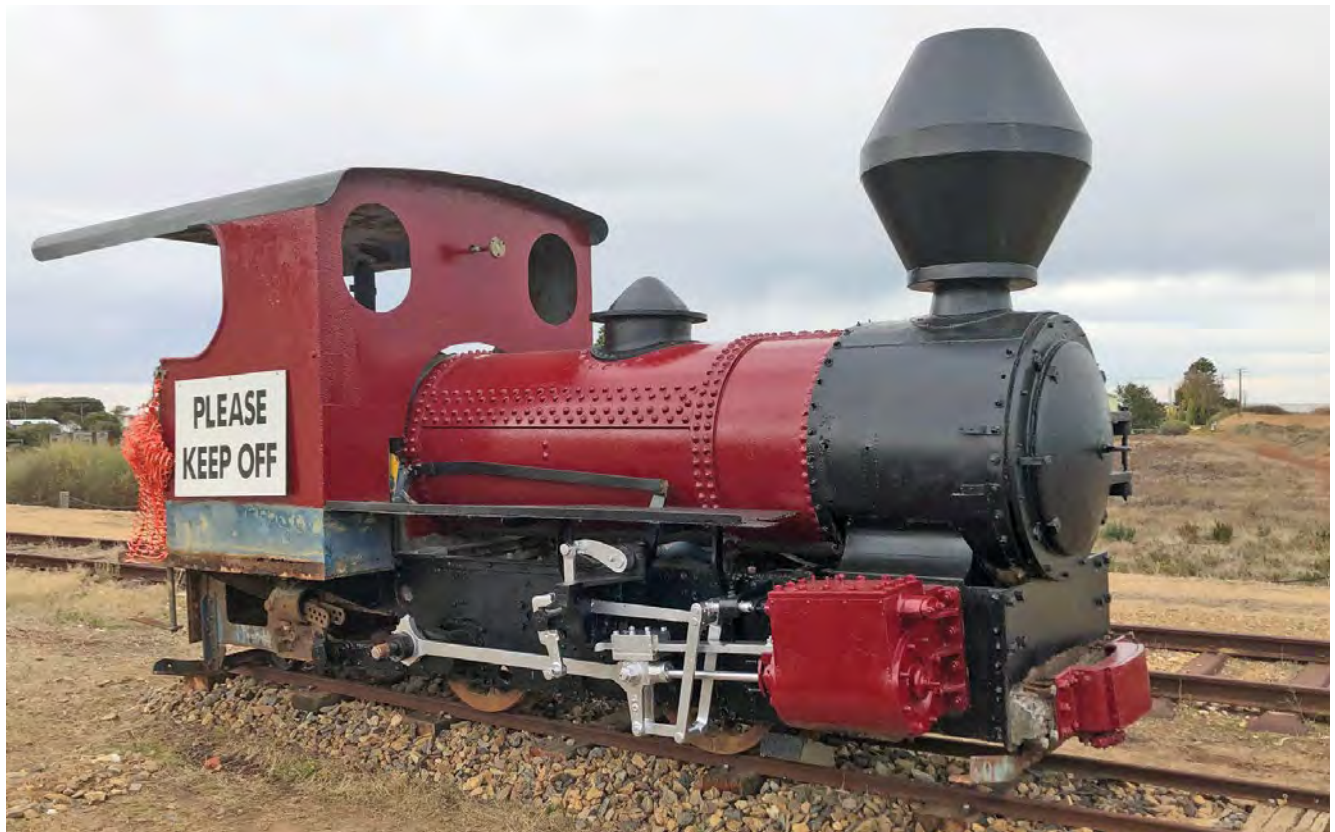
Above: The 1927 Fowler locomotive ex the cane fields near Mackay on its arrival at Milang at the end of May 2021. Below: After arrival at Milang, and during gaps in the bad weather, volunteers have been pushing forward with restoration and this photo shows its current status whilst on display. Photos: Peter Lucas
