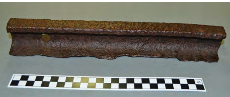
Above: Undated view of the route of the overhead wire electric railway marked by the bright white painted support posts. Photo: Beaconsfield Mine & Heritage Centre collection. Left: Piece of rail recovered from the site of the gold mine battery, so quite possibly from the tramway. The rail measures 1\frac{3}{4} in high x 1 in wide across the head x 2in wide across the bottom flange which would equate to roughly 12-14 lb/yd. The black and white squares measure 10 mm x 10 mm each. Photo: Beaconsfield Mine & Heritage Centre collection. Below: Robert Hudson Ltd V skip and V skip frame on display at the Beaconsfield Mine & Heritage Centre. Photo: Beaconsfield Mine & Heritage Centre collection.
