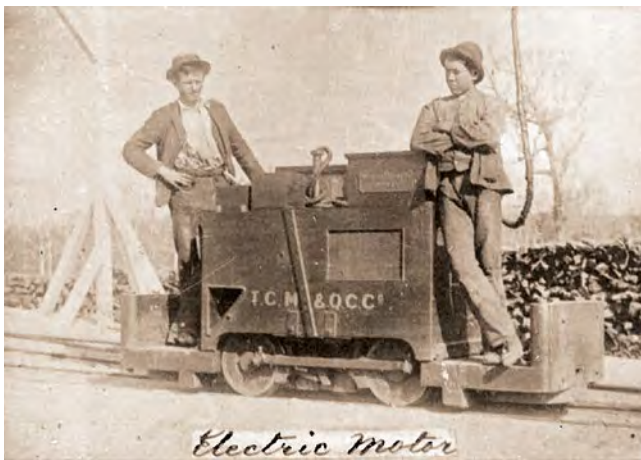
Close up of the overhead wire electric locomotive, described as an 'Electric Motor', and sometimes erroneously in newspapers as an 'electric motor car'. Note the pyramidal timber braces stabilising the OHW support posts. The letters 'TGM&QCC' stood for the Tasmanian Gold Mining and Quartz Crushing Company.
