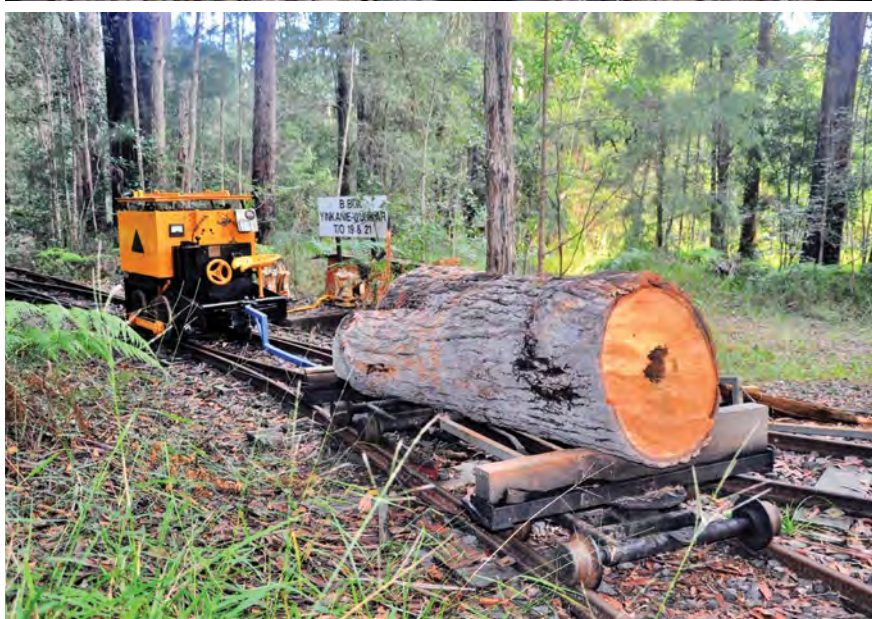
The Wingrove and Rogers battery electric locomotive (Builders number 2216 of 1942) in use at the Tinbeerwah Mountain Railway in July 2021. The locomotive is used for yard shunting and saw mill duties including movement of the former Smithfield wagons around the site. All photos: Russell Savage
