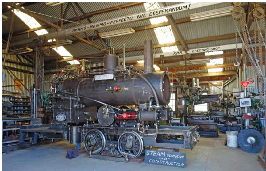
Pictured in the Kerrisdale Mountain Railway Erecting shop on Easter Saturday 2018 is the railway's steam locomotive currently under construction. Designed and built by Andrew Forbes the locomotive features many unique design elements. Construction is progressing well with potential test runs before the end of the year. Photo: Sam Daly
