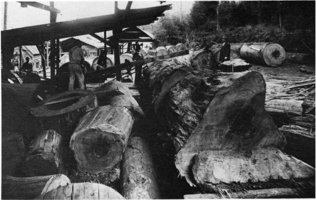
17. *Steam driven drag saw, sawing waste mountain ash into 3ft lengths for splitting into retort wood at No.2 mill. The decayed nature of some of the logs can be seen. Notice the moving bench (on wheels) enabling the logs to pass under the drag saw. Mr. Tom Richards at the drag saw, Mr. Frank Edwards in the log yard.
