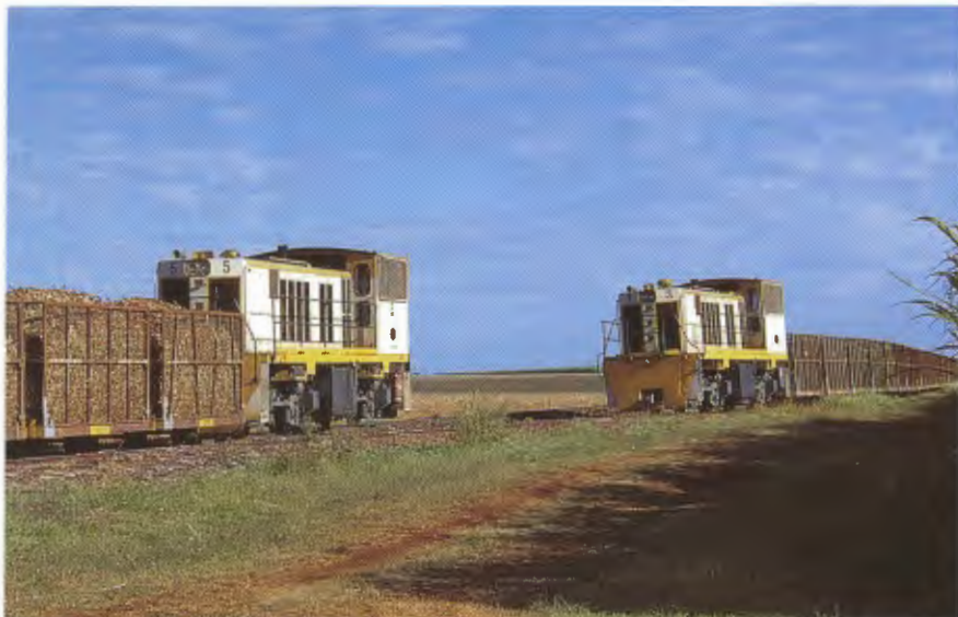
Isis Mill's 610mm gauge Walkers B-B DH 5 (617 of 1969 rebuilt Isis Mill 1998) with fulls from Farnsfield, passes 3 (600 of 1968 rebuilt Walkers 1994) with empties for Goodwood at Kowbi, 2 August 2000 Photo: John Browning
