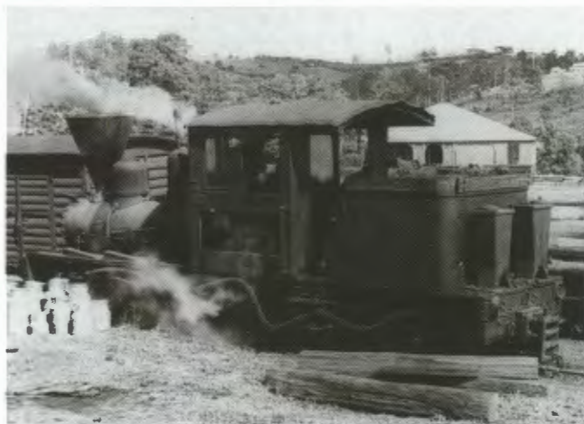
DULONG at Nambour. The ejector water pipe, mentioned in the text, is clearly visible. Photo: Ken Rogers via George Bond
