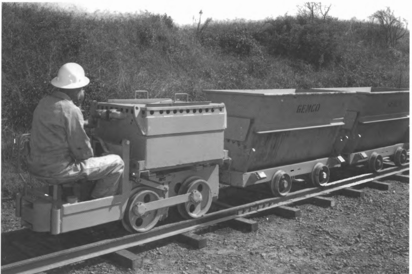
A Gemco Trammer poses with two Gemco side tippers at the Plant Maintenance Depot, Birrong, 1967.
