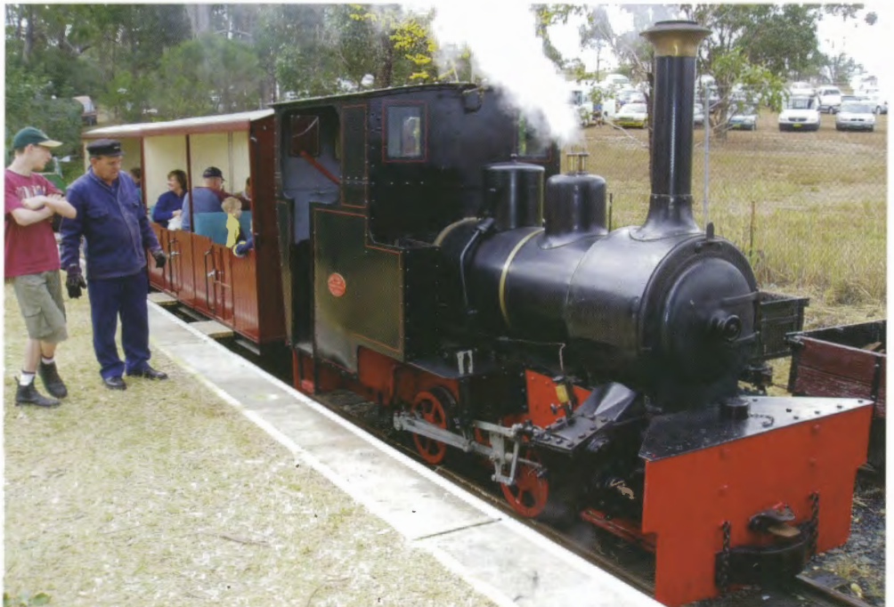
The ex-Corrimal Colliery 0-4-0WT (Robert Hudson 1423/1923) and refurbished carriages await another load of passengers at the Menangle Narrow Gauge Railway station on 14 May 2005. Photo: Bob McKillop
