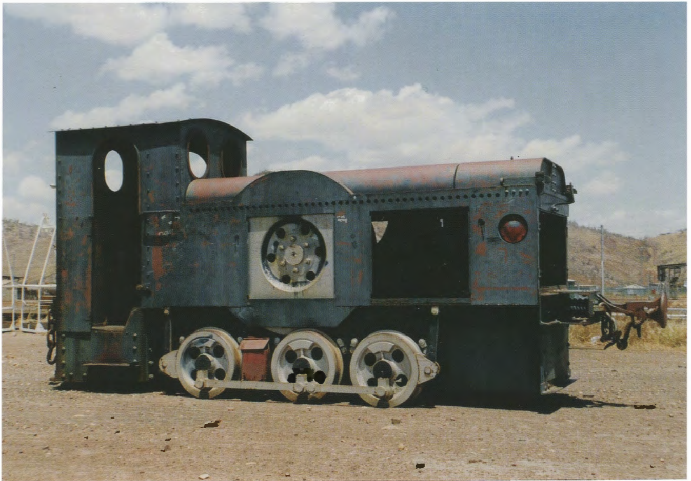
West Australian Public Works Department 0-6-0PM NW 3 "Kaiser" (Ruhrthaler 161 of 1912) at the Department of Transport workshop, Wyndham port on 27 September 1992. Photo: Jeff Austin
