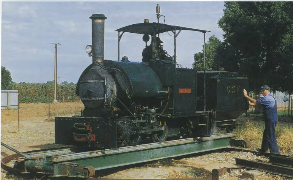
Cobdogla Irrigation Museum: Bagnall 0-4-0ST 1801 of 1907 is turned at Mudges Loop, 24 April 2005. Photo: Ray Graf
