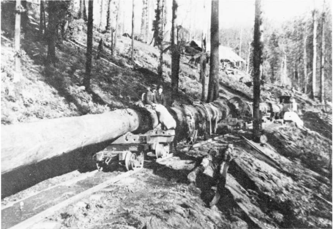
Ezard's locomotive at the rear of a train of logs on the way to the mill. The loco always travelled at the rear of the train on the downgrade to the mill. F.C.V.
