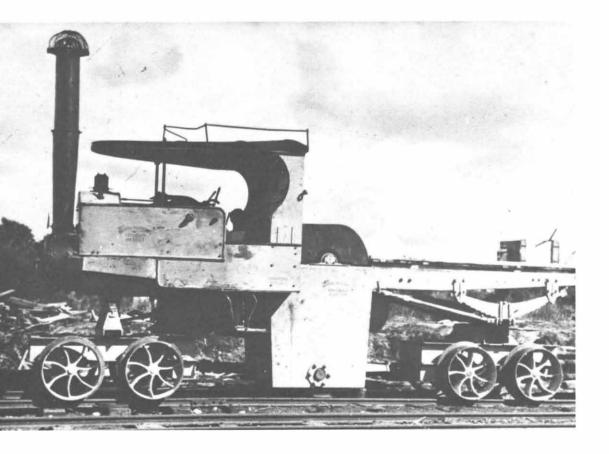
A steam road lorry converted by Russell Allport, Engineers of Hobart, to work on the 3ft 6in gauge Salmon River Tramway in north-west Tasmania. The eight tramway-profile wheels were all driven, by cardan shafts, which can be seen in the photograph.
