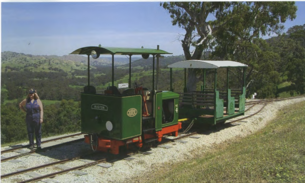
Kerrisdale Mountain Railway's Ruston & Homsby 20DL 4wDM (B/N 285301 of 1949) and four-wheel open carriage at The Summit loop during the Chartered Institute of Transport Australia's visit on 15 November 2003. Photo: Mal Dow
