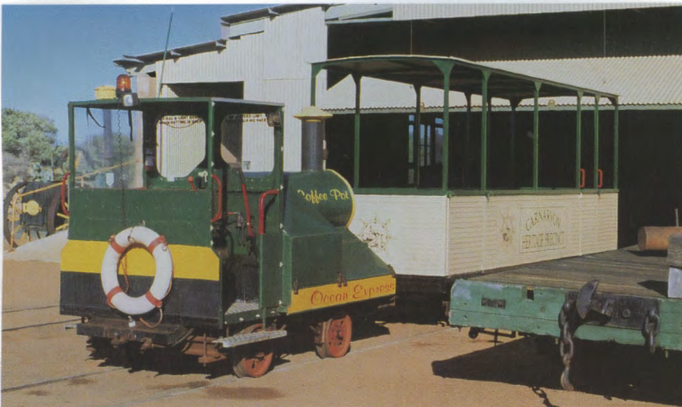
The 4wPM Volkswagen-engined steam outline, locomotive Coffee Pot, standing outside the depot at Carnarvon with the carriage for the jetty tramway. When photographed by Ray Graf in June 2003, operations had been suspended due to insurance problems.
