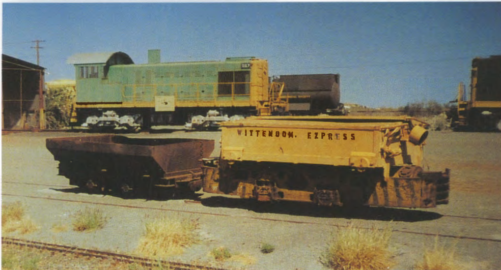
Mancha 4wBE WITTENOOM EXPRESS has been salvaged from the abandoned Wittenoom asbestos mining site and placed on display at the Pilbara Railway Historical Society Museum at Dampier, together with a four-wheel mine car. This locomotive is believed to be one of Mancha 3043 and 3044 of 1949, and 4079 of 1957. Photo: John Smith
