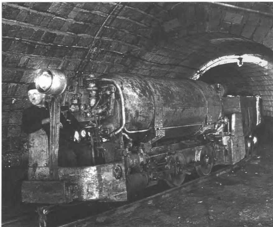
A 40HP 0-4-0 compressed air locomotive built by Demag Engineering of Duisburg, Germany, at work in an underground coal mine. Classified as their Type DL 40/30, it featured a tractive effort of 750kg and driving controls at both ends. Photo: AD Lockyer Collection
