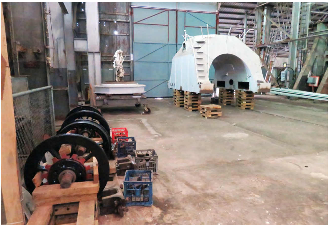
Below: Travelling steam crane No.001 under restoration by volunteers in the Heavy Machine Shop on Cockatoo Island, October 2021. The four wheels are seen in the left foreground, the rotating roller bearing behind them and the main under-carriage mounted on timber blocks. Photo: Author
