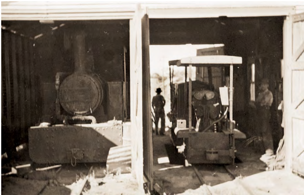
Inside the locomotive shed in March 1951. The Kerr Stuart sits gathering mallee dust in the shed extension added with the arrival of the small Malcolm Moore in 1927. A skillion lean-to had sat here before then. On the right the small Fordson and one of the larger 1000 series Malcolm Moore locomotives, '8-B-245', stand over the pit in the original shed. Photo: Arnold Lockyer
