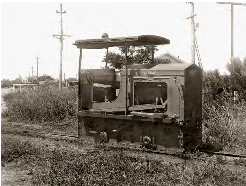
Malcolm Moore b/n 1015 on the northern leg of the 'wye' at the Red Cliffs siding on 30 November 1952. This was the first of the 1000 series locomotives delivered to Red Cliffs and was re-engined with a Hercules DJX diesel in 1948. On the side rack can be seen the wooden sprags used to prevent runaway trucks at the pumping station as well as, to the right, a jack used for rerailing the locomotive and trucks. Photo: RB McMillan
