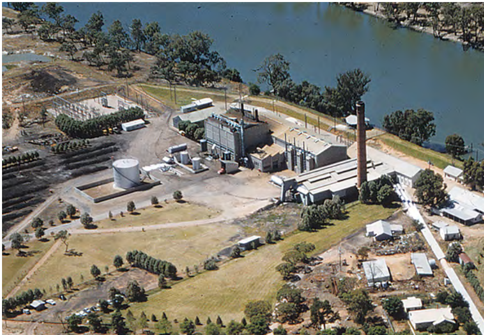
The Red Cliffs pumping station and power station on 6 March 1961. All trace of the tramway to Red Cliffs has gone but visible at the rear of the pumping station boiler house is the ash tramway. It weaves its way around the power station where the siding for the removal of briquette ash from that facility is visible. The Malcolm Moore, Fordson V8 and a line of ash trucks are parked on the siding leading to the SECV powerhouse. At the far left is the ash dump where, by this time, the tramway terminated.
