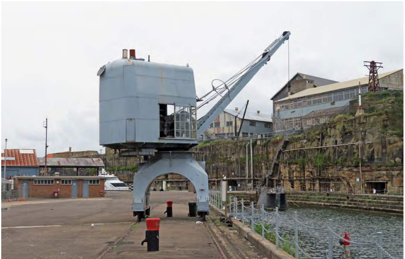
Above: Restored travelling steam crane No.002 pictured on the southern side of the Fitzroy Dock in October 2021 with the high central sandstone plateau in the background and the caisson floating in the end of the dock. Beneath the crane can be seen two of the bollards that are placed around the dock, they are mostly ships cannons cemented in place. Photo: Author
