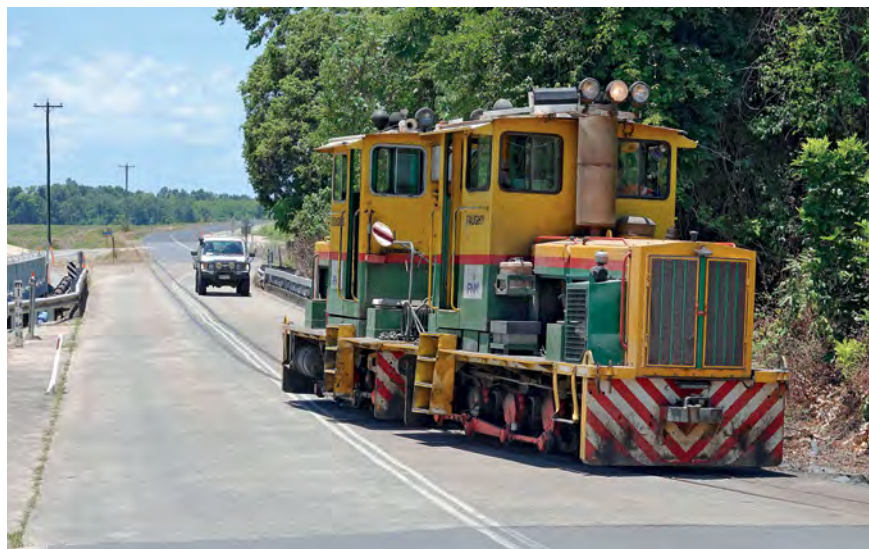
Com-Eng 0-6-0DH multi-unit locos Faughy (AL4190 of 1965) and Douglas (AL2562 of 1963) cross the South Mossman River road and rail bridge as they head back to Mossman Mill after dropping off empties at Valeses siding in the Bonnie Doon area on 24 October. Photo: Gregorio Bortolussi
