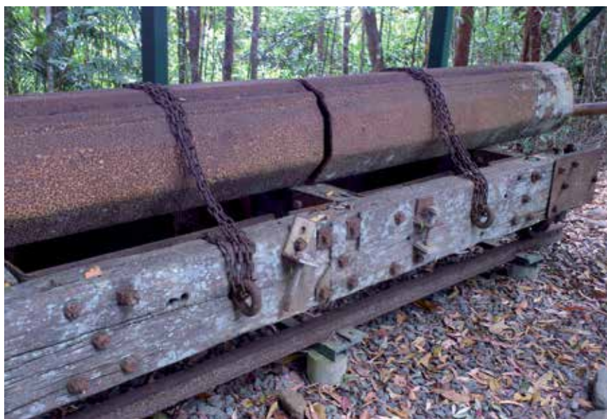
The haulage wagon (complete with sections of iron pipe) that was used in the construction of the Barron Falls power station.
