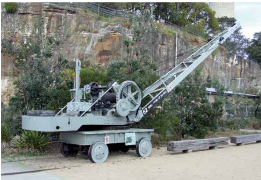
This mobile crane was manufactured by Davis and Primrose, Edinburgh, Scotland in 1912 and was capable of propelling itself around its workplace at Sutherland Dock. Photos: Terry Elliot
