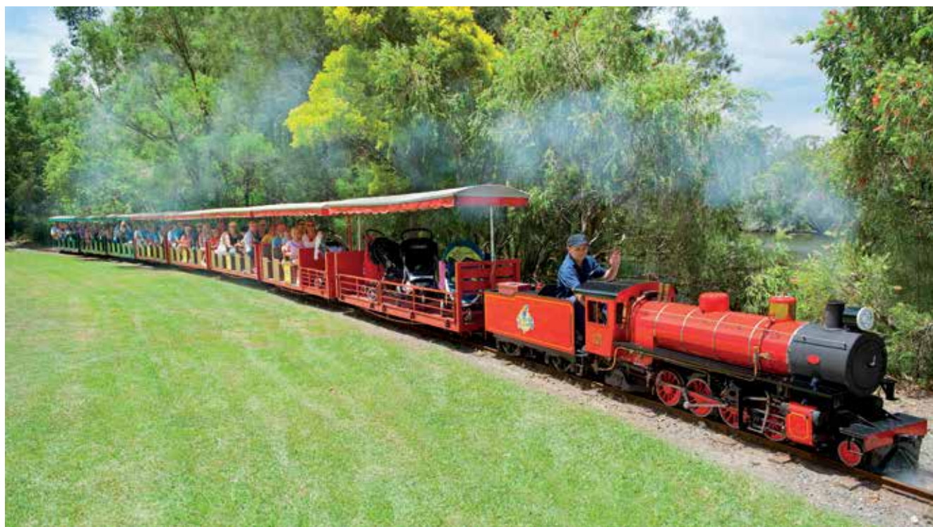
While the locomotive has changed its appearance little after 50 years of operation, the 2011 overhaul saw a new boiler manufactured, braking systems upgraded and the locomotive fully overhauled. It now shares the task of hauling the park's 400,000 annual visitors with three other locomotives. Photo: Currumbin Wildlife Sanctuary
