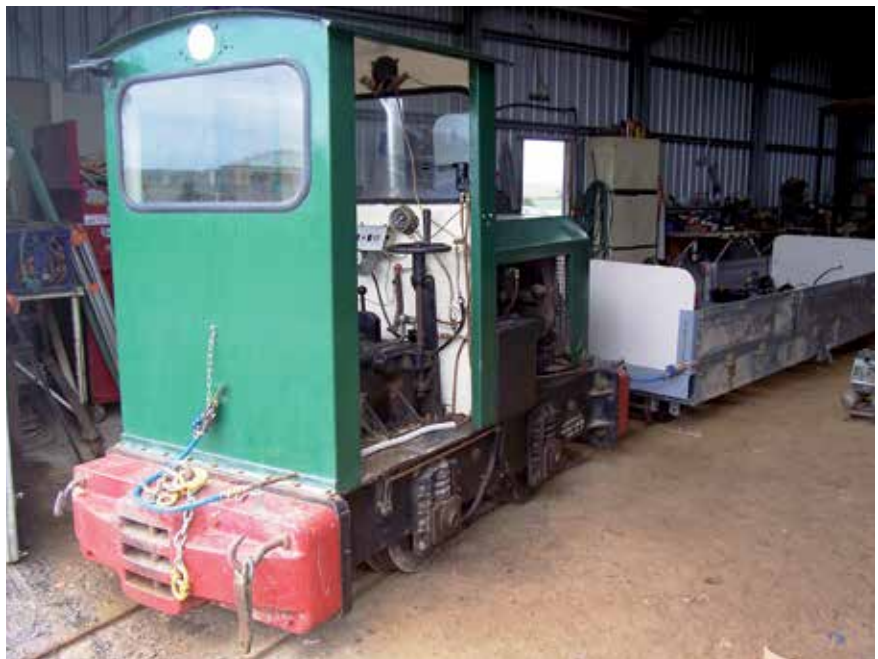
The photo shows the 610 mm gauge Tulloch locomotive Number 003 of 1959 'on shed' on the Glencoe Agricultural Tramway in front of a new bogie wagon, Feb 2014. The locomotive and wagon had just been fitted with a 'fail safe' air brake system using truck standard air brake parts reducing costs significantly. This was decided and designed by the owner, and was not a regulatory requirement. The locomotive is in regular use and is not a display item as can be observed by the red paintwork. Photo: Garry Barker
