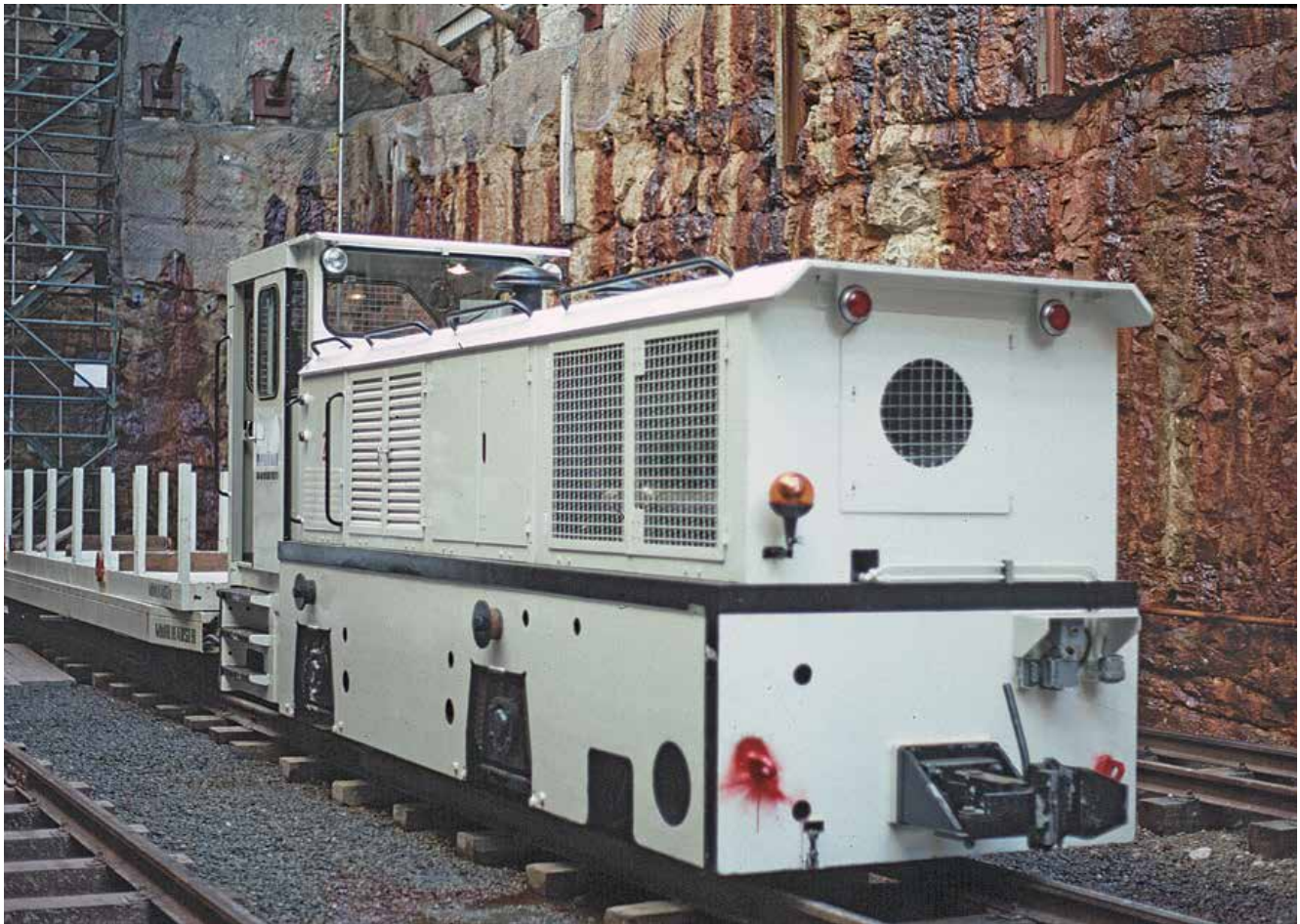
Exhibiting its third driving cabin incarnation, now with floor height almost at deck plate level, Schöma 4861 of 1985 is ready for work at the bottom of the Tempe Reserve launch shaft, on 22 March 1997. Photo: Ray Graf, LRRSA collection.
