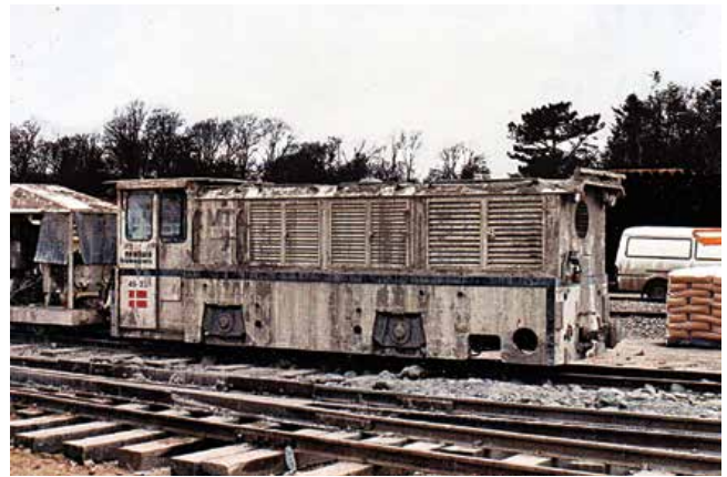
Onerous duties while on the Storebælt-Tunnel in Denmark with a liberal coating of muck. Note the height of the cab roof, and cabin floor level indicated by the bottom door rail. (4860 of 1985). Photo: Bent Hansen
