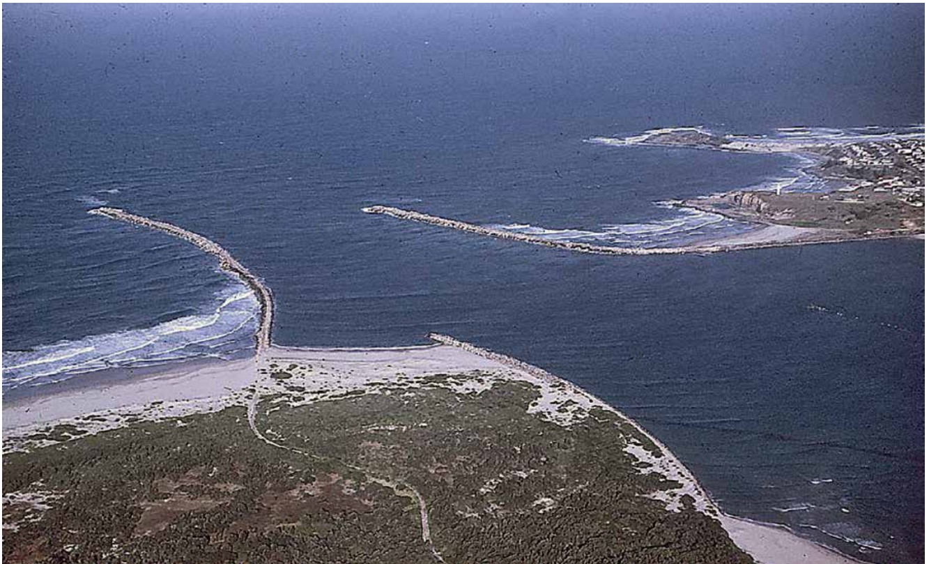
Contrasting aerial views of Clarence Heads in the 1940s (above) and in 1969 (below). The head of the Iluka Training Wall served as a de-facto northern breakwater for over 50 years until the North Breakwater was completed in 1969. Tide-borne sand was a continual problem for navigation inside the estuary. It was responsible for the formation of Hickey Island, which closed off steamer access to Yamba Bay. Photo: Norm Brown collection
