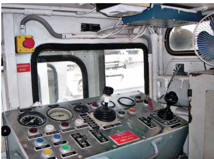
Above: The unusual lateral position of the control station on the right-hand side of the now cramped cab of Schöma 4860. Photo: Alain Ballmer
