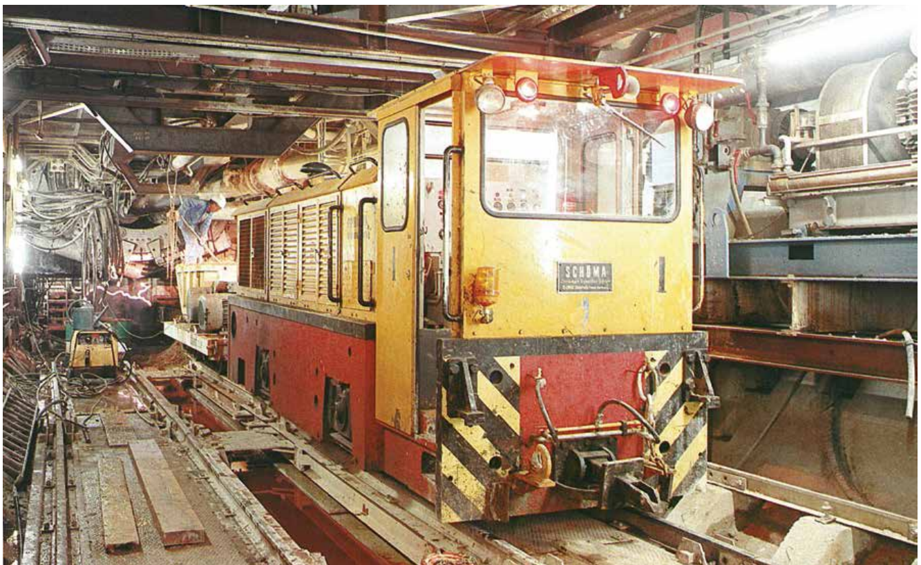
Schöma CFL200DCL 4858 in its original guise working as #1 on the TGV Atlantique Tunnel in France. Note the floor height inside the cabin just above the bottom door rail. Photo: Schöma Official
