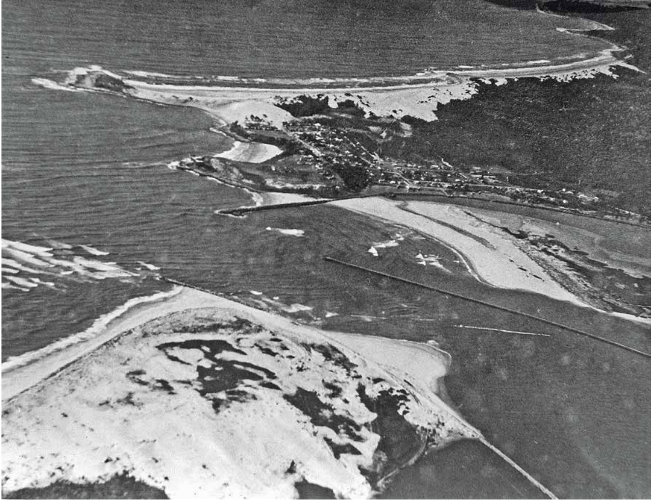
Contrasting aerial views of Clarence Heads in the 1940s (above) and in 1969 (below). The head of the Iluka Training Wall served as a de-facto northern breakwater for over 50 years until the North Breakwater was completed in 1969. Tide-borne sand was a continual problem for navigation inside the estuary. It was responsible for the formation of Hickey Island, which closed off steamer access to Yamba Bay. Photo: Norm Brown collection
