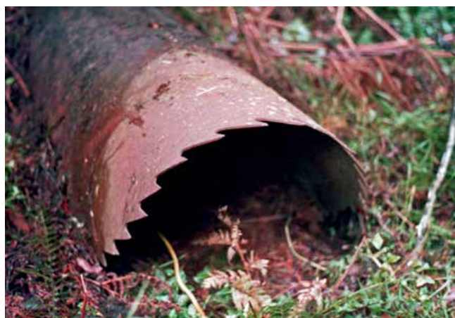
Above left: A drum saw (blade only) abandoned at the New Federal mill near Warburton. The Enterprise drum saw would no doubt have been similar to this. Photo: Peter Evans Above right: Raw staves and finished barrels at the MacRobertson chocolate factory in Fitzroy. Unknown photographer, State Library of Victoria image H2003.101/63.
