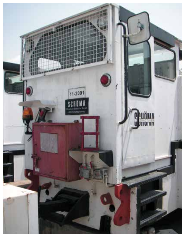
Below: The lowered roofline as altered from the Australian cab on 4859. Compare the cab door window and the cut-down cab side window position on the Hong Kong cab. Photo: Alain Ballmer
