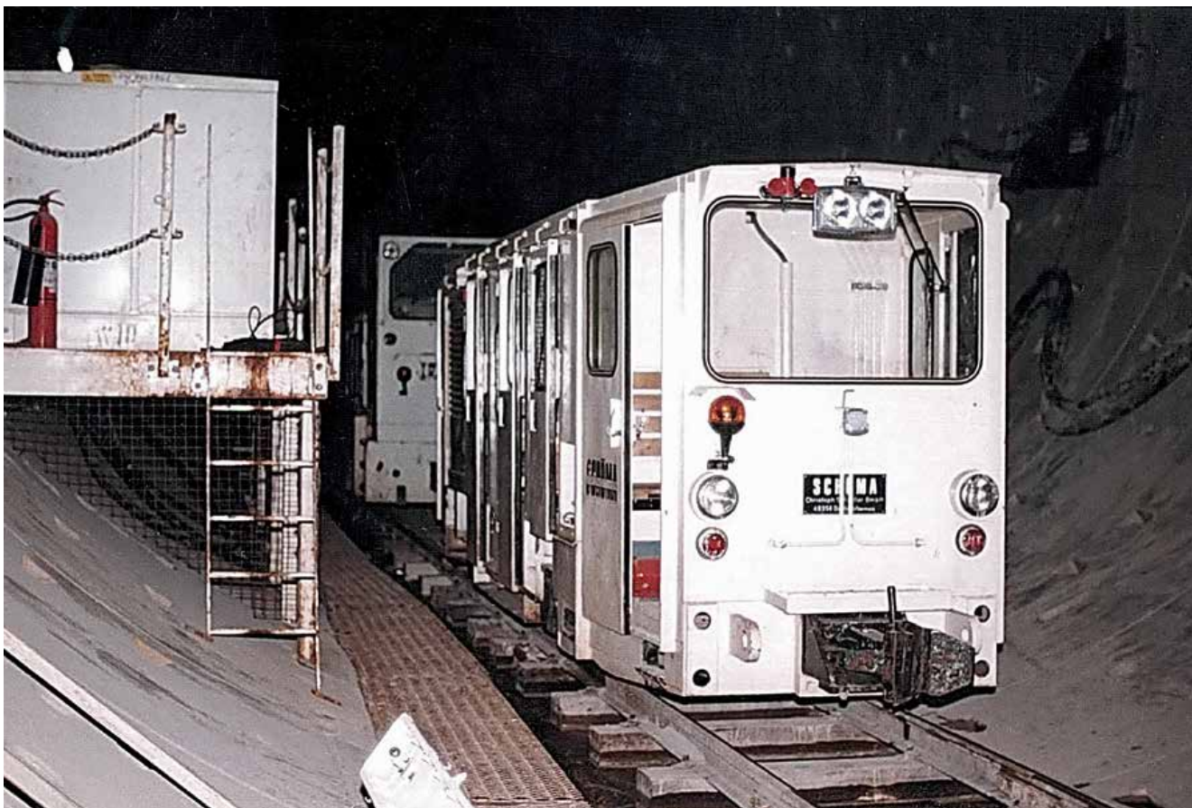
Below: Attending to man-riding duties for the Transfield/Bouygues JV, Schöma D60 (5024 of 1989) was already a veteran on its third tunnel project since its debut on the Channel Tunnel project between Great Britain and France. Photo: Kevin Waid
