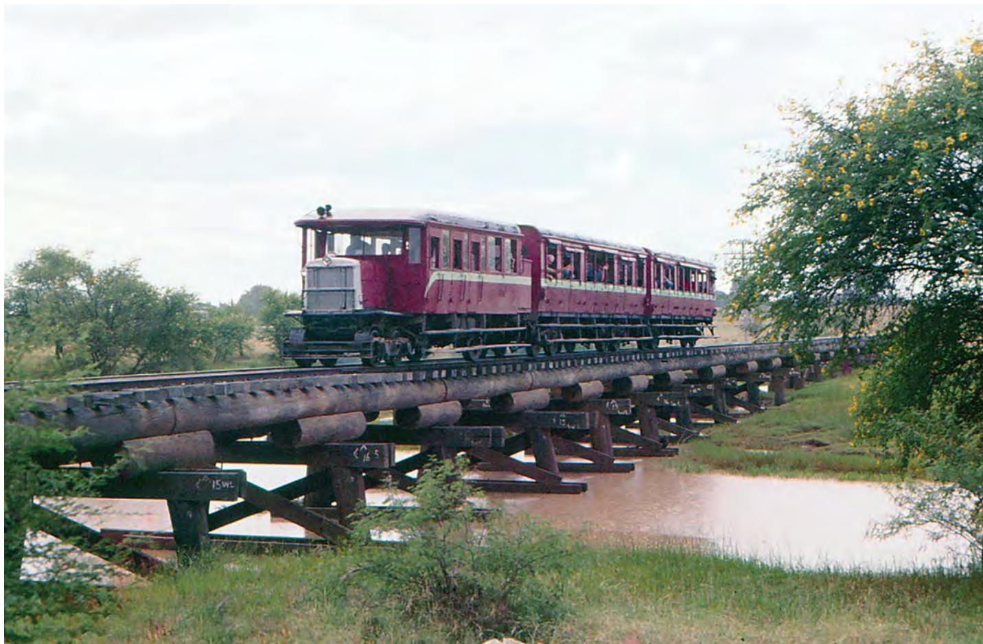
Aramac Creek bridge. Having reached Aramac, Aunt Emma has been turned and is now heading south, as the rain starts. RM28 was built at Ipswich Workshops and entered service with the QGR in 1928. Its original 45hp AEC petrol engine was replaced with a 50hp Gardner diesel in 1942. Restored by the QR Heritage Unit at Ipswich Workshops in 2003, RM28 is now preserved at the Aramac Tramway Museum. Photo: Ken Biggs, courtesy ARHS Qld
