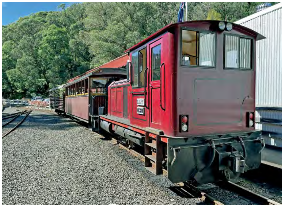
No.030, Kasey, a 4wDH built by E M Baldwin (b/n 3225.4.2.70 of 1970) had a varied career with the MMBW before finally ending up at the WGR in 1998. A rebuild by the Morwell engineering firm, Valicote Pty Ltd, saw the ex-tunnelling loco fitted with a neat cab to withstand the mountain rains – a rare event, of course! Photo: Phillip Milbourne
