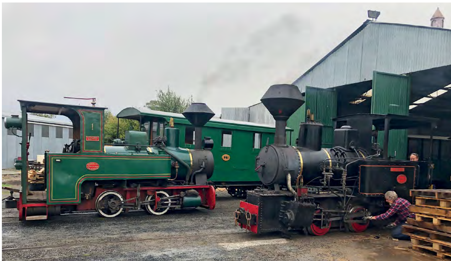
The Redwater Creek Krauss and the Fowler (Wee Georgie Wood) outside the Sheffield workshops on 5 March. The Fowler had to be turned to face the other way as during running tests the rear locomotive skid fouled on the turntable, which would have carried an unacceptable risk during the busy Steamfest operations. Photo: James Shugg
