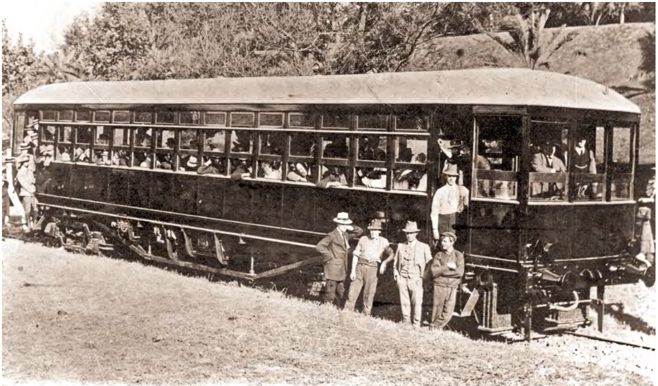
The Caldwell-Vale auto rail car photographed on the Adelaide Exhibition Line during a demonstration run, 1913. Whilst it was a fine-looking vehicle, thanks to the body work by Duncan & Fraser, underneath all was not well and mechanical problems brought about its demise including hot bearings, severe vibration and compressor troubles. Photo: Arnold Lockyer collection, courtesy NRM
