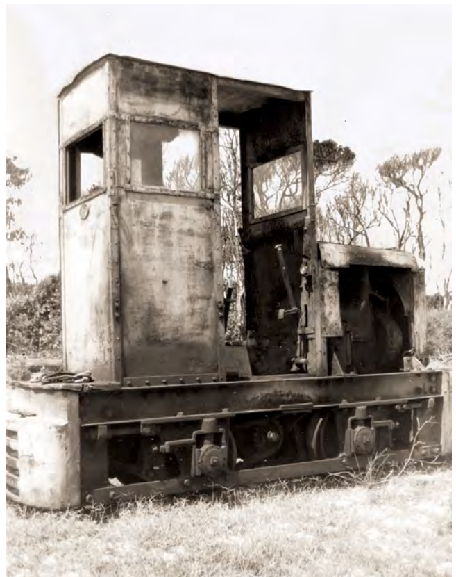
The Caldwell Engineering (Australia) locomotive out of use at Kingscliff. The John Fowler radiator and the oval builder's plate on the rear of the cab generated confusion among railway historians regarding the builder of this locomotive. Photo: Author's collection
