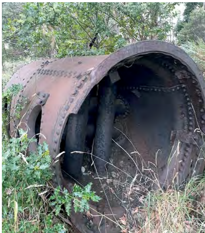
Above left: Boiler believed to be from a former vertical-boilered locomotive. Above right: Locomotive boiler converted to log-hauler and formerly mounted on a wooden frame. One wheelset survives underneath the boiler confirming the gauge as 1372 mm (4 ft 6 in). Photographs supplied by Tom Dearing
