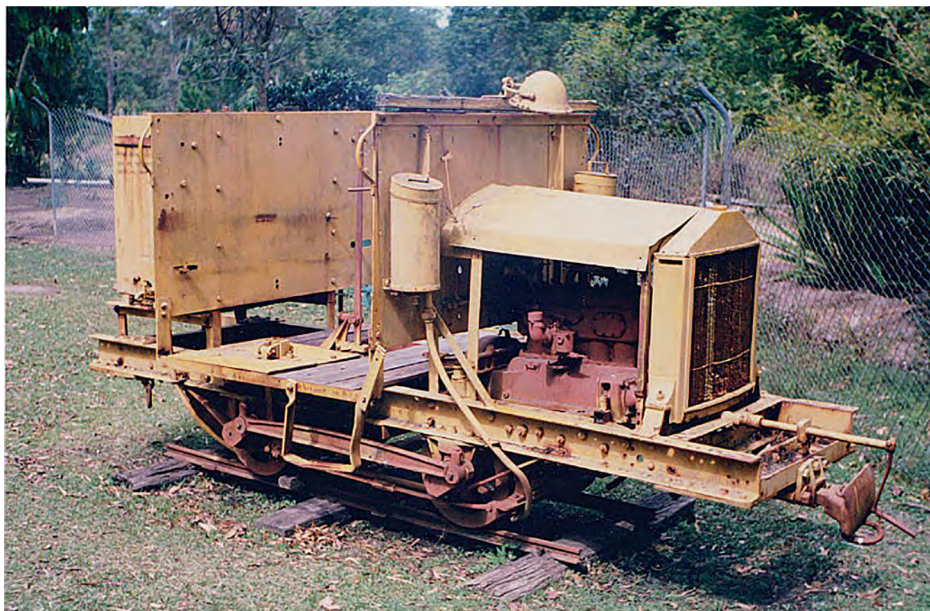
Remains of the 1913 Caldwell-Vale ex-Moreton Mill locomotive Vanguard, as saved by Graham Chapman in the 1990s. This loco, much altered though the chassis and wheels seem original, as well as the distinctive connecting rods, is now at the Kerosene Creek Tramway in the Blue Mountains, NSW. The headlight remains mounted centrally on the cabin firewall, while the cylindrical sand boxes are also prominent. Full details were covered in Part 1. Photo: Graham Chapman
