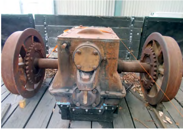
Undated view of the gearbox and driving wheelset of the Purcell at the West Ryde Water Pumping Station now at Valley Heights Locomotive Roundhouse Museum. Photo: Peter Stock
