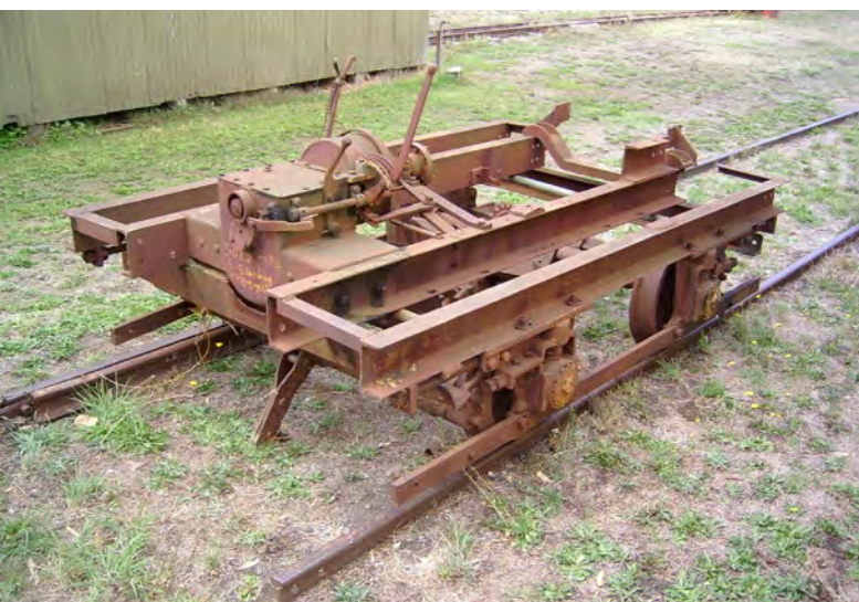
Undated view of the remains of Flora at the Alexandra Timber Tramway & Museum, showing how the frame was widened on both sides to accommodate the longer axles for the wider gauge. Photo: Peter Evans
