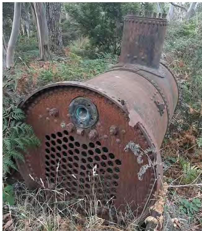
Above left: Boiler believed to be from a former vertical-boilered locomotive. Above right: Locomotive boiler converted to log-hauler and formerly mounted on a wooden frame. One wheelset survives underneath the boiler confirming the gauge as 1372 mm (4 ft 6 in). Photographs supplied by Tom Dearing
