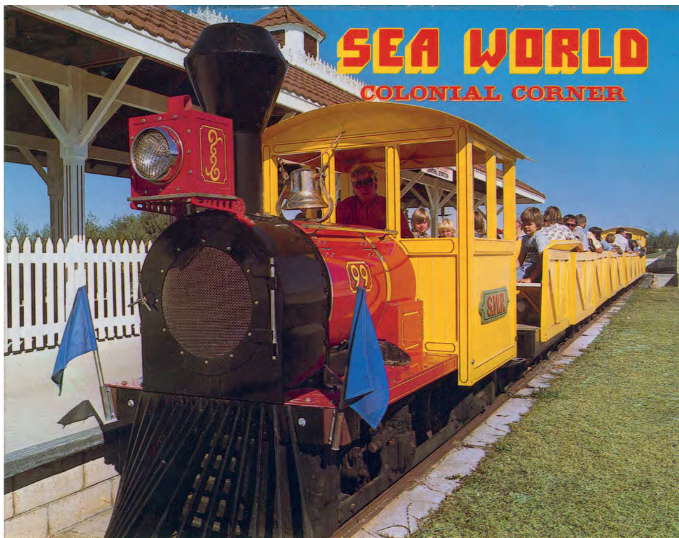
Steam outline internal combustion locomotive known as 'Old 99', built on a Caldwell Engineering (Australia) frame, on the railway at Seaworld, foldout postcard pack. Photo: G Fleming collection
