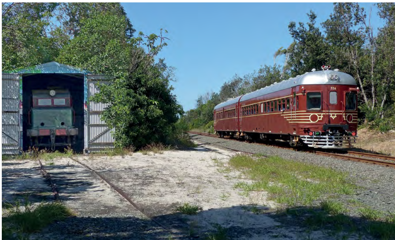
Byron Shire's Simplex locomotive peeking from its shed on 24 April 2021. Passing on the former NSWGR Murwillumbah line is the Byron Bay Railroad Co's beautifully restored 1949-built 600-class two-car rail motor set. The rail motor is solar powered, with panels on its roof, supplemented by solar panels on the BBRC depot roof at West Byron. (technical details at https://byronbaytrain.com.au/sustainability/ ) The out-of-use track parallel to the main line is the former jetty line, from the Byron Bay station yard to the long-gone 'new' jetty. Photo: Phil Rickard
