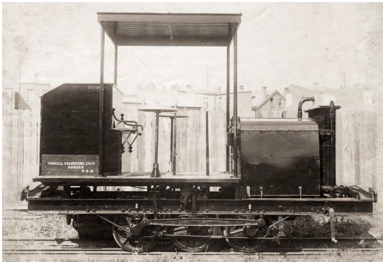
Builder's photograph of the four-ton, friction-drive locomotive delivered to Mannum in June 1921.
