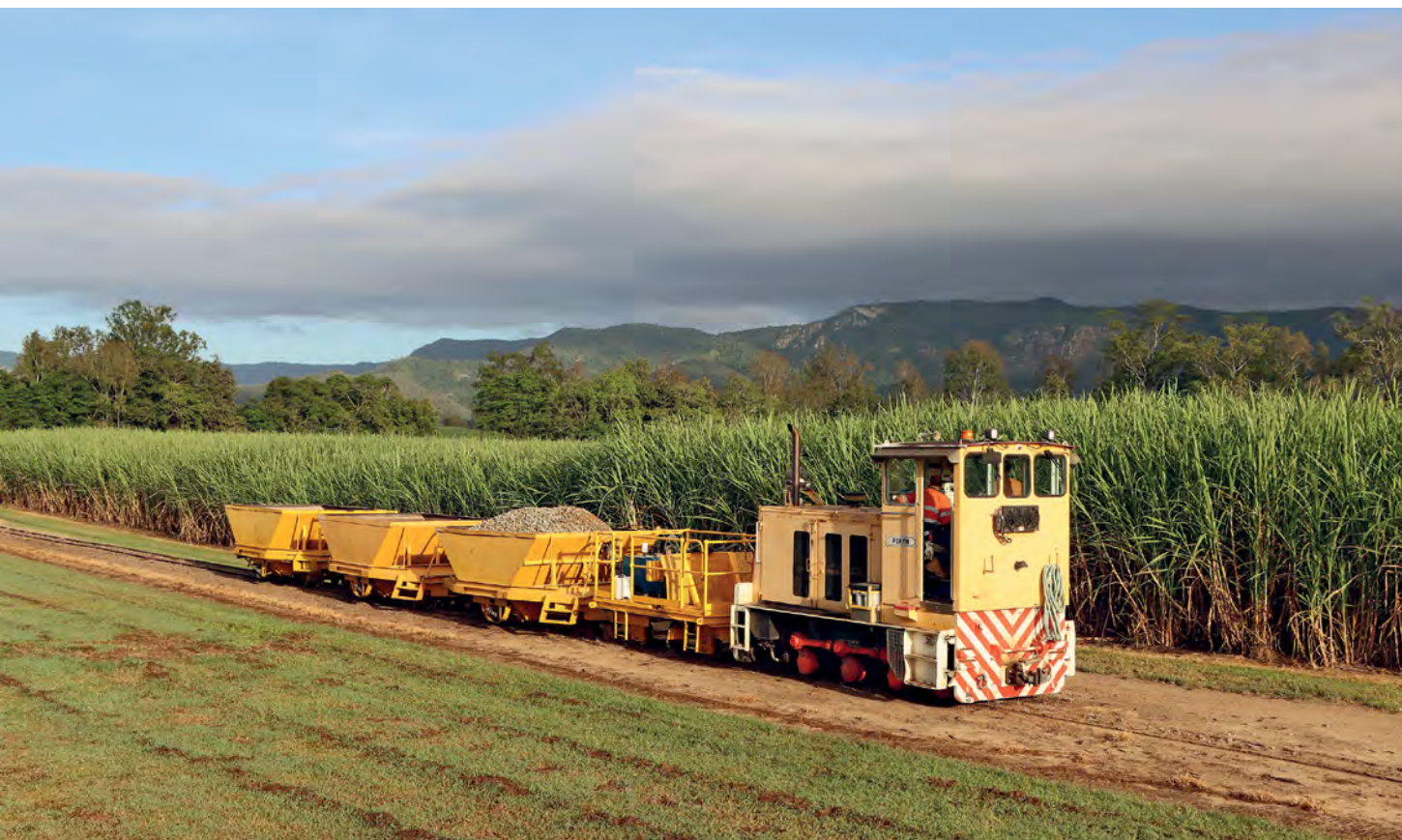
Above: Victoria Mill's Clyde 0-6-0DH Perth (69-682 of 1969) with a ballast train at Upper Stone on 22 May. In the consist is the ballast plough on loan from Proserpine Mill. Photo: Luke Horniblow
