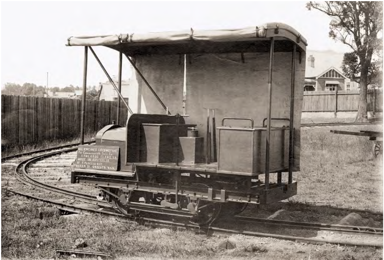
Builder's photo of the Purcell inspection truck for the Salt Lake to Muston tramway. Cheetham Salt Co records (1930) note this vehicle with a petrol engine, so the original oil engine must have been replaced. The builder's placard states "Builder: T.Purcell & Co." making its manufacturing date was prior to 1921, when Purcell Engineering Co Limited was floated. Seating is very basic though the roll-down blinds would have been appreciated on a wintery day when a south-westerly 'breeze' comes off the Southern Ocean!
