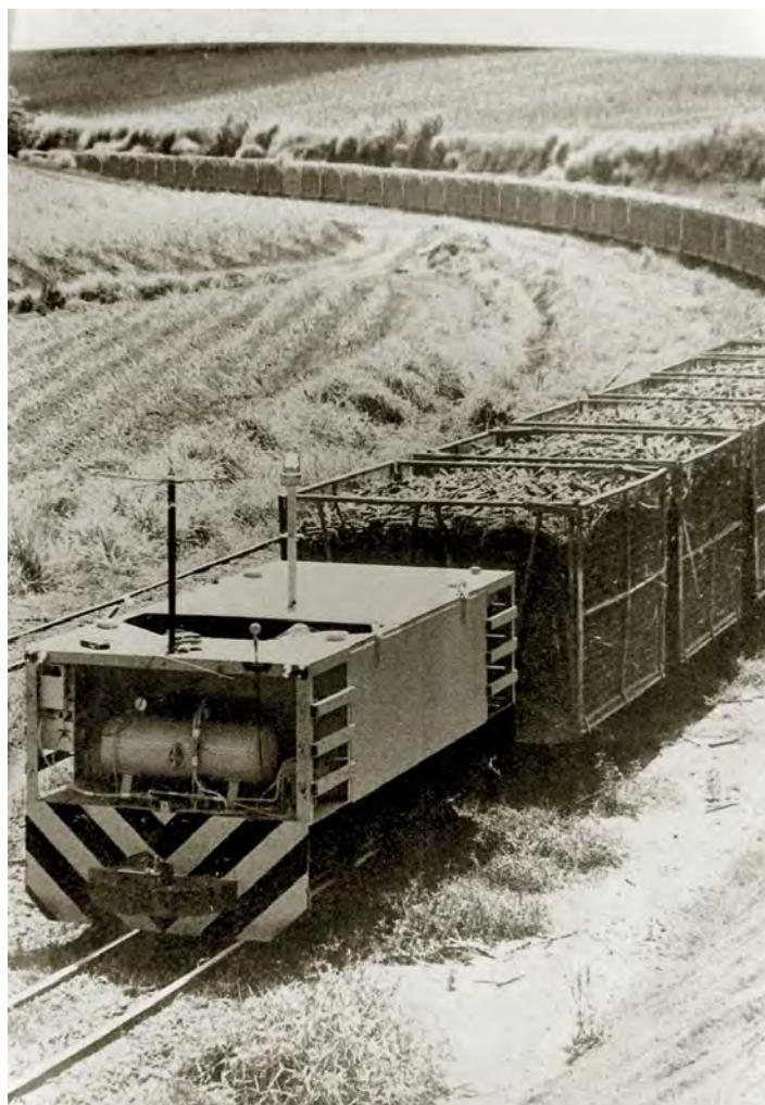
SRI developed a remote control system for cane railway brake wagons which could be controlled by the driver of the locomotive using radio control technology. This photograph taken in 1972 shows a Clyde Engineering-built brake wagon fitted with the SRI remote control equipment at the rear of a train consisting of 110 four-ton bins hauled by a single diesel-hydraulic 0-6-0 locomotive on the South Johnstone mill rail system. Photo: SRI via I.R.Crellin
