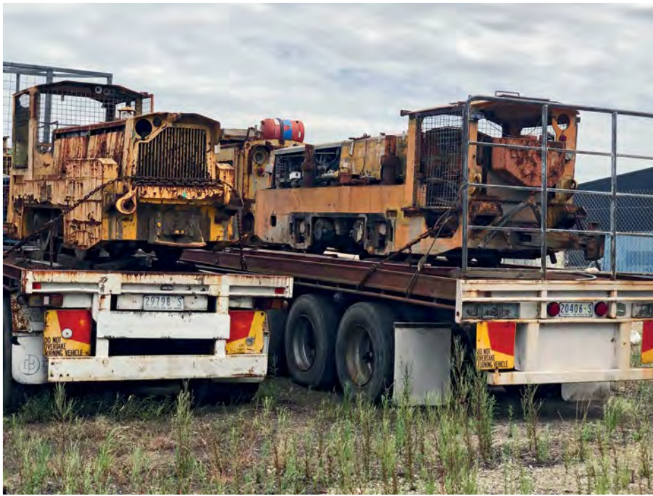
Above: Four 4wDH tunnelling locos stored on semi-trailers in the Traralgon area on 29 December. Two are FM Baldwin model 8T294 built in 1994, one is FM Baldwin model 12TRA295 built in 1995 and one is Clayton Equipment (UK) B1864E of 1979. Photo: Jack Daly Below: Goninan Bo-Bo DE 49 (013 of 1961) at Cockburn Cement in Parkeston on 11 August. Photo: Barry Trudgett
