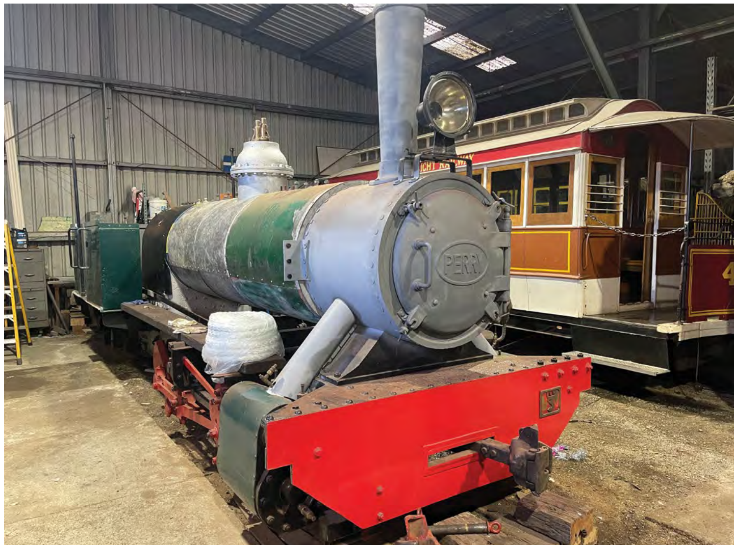
Work on the Perry locomotive showing its boiler in place in the workshops of the ILRMS at Albion Park, NSW. Photo: Brad Johns
