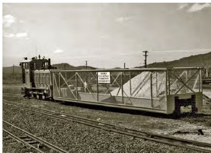
Above: The 20-tonne prototype wagon built by NQEA stands in the yard at Farleigh mill in 1988 prior to being filled with gravel to simulate a full load of chopped cane for running tests. Below: A drawing of the innovative wheelset arrangement for the Big Bin developed by NQEA and SRI. Photos: NQEA Australia
