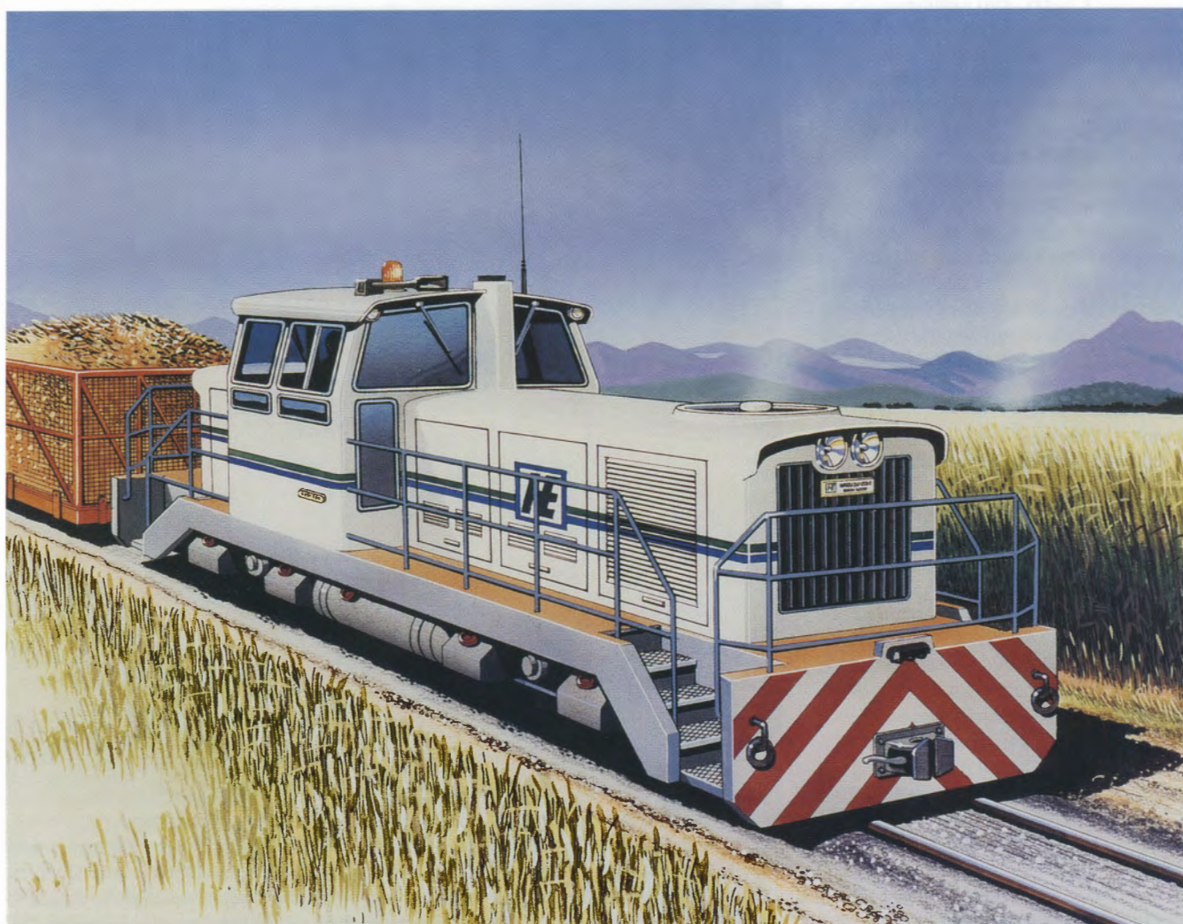
An artist's impression of the Hexham Engineering B-BDH 2ft gauge cane locomotive. This unit may well have seen the light of day in 1991 had Hexham still been in business by that time.
