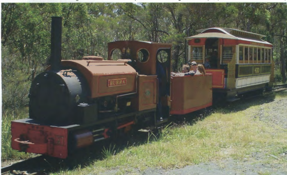
Former Corrimall Colliery 0-4-OST BURRA (Hawthorn Leslie 3574 of 1923) hauling the match truck and ex-Melbourne cable tram trailer 430, on the 'bay road run' at Albion Park on Sunday 9 November 2003. Photo: Brad Johns
