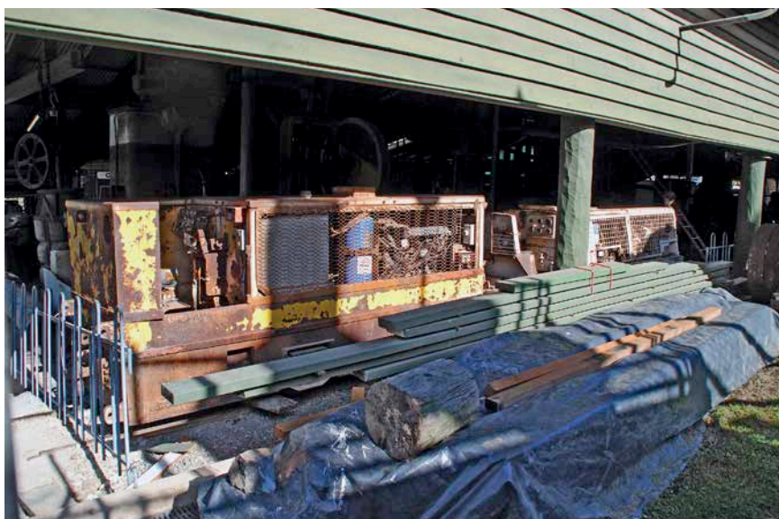
4wDH built by Bermagui Foundry in 2002, and 4 wDH built by E M Baldwin (B/No.4661.?.7.72) of 1972 at the Gympie Mining & Historical Museum, 22 May 2017. Photo: John Browning
