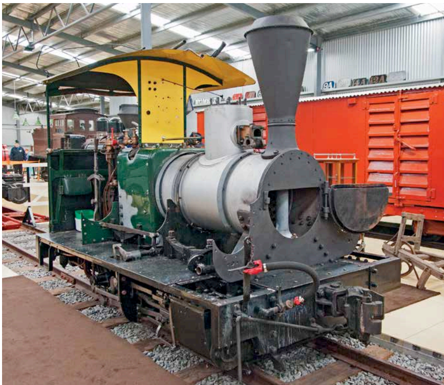
Ex-West Melbourne gasworks Carbon at the Puffing Billy Menzies Creek Museum, 2 June 2017. It is being prepared to re-enter service following the fitting of a new boiler. Photo: Frank Stamford
