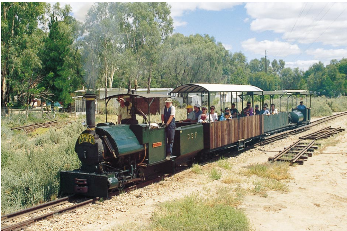
The Bagnall locomotive in action, with its four-wheel tender, the two bogie carriages, and the combination waggon in tow. Photo: Denis Wasley
