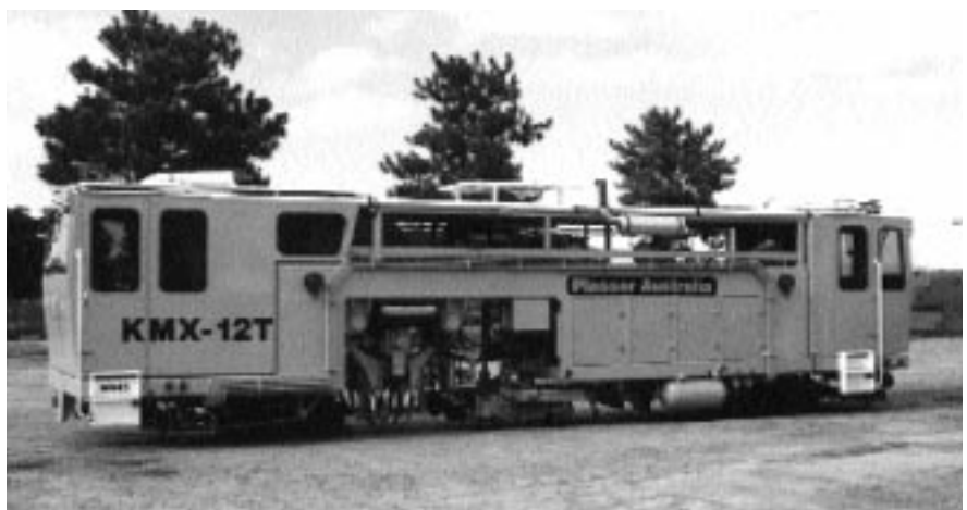
The newest Plasser KMX-12T, for CSR's Herbert River mills (445 of 1998) is indeed an impressive machine at 13m in length and weighing in at 22 tonnes. Photographed at the Victoria Mill navy depot, 30 November 1998. Photo: Chris Hart
