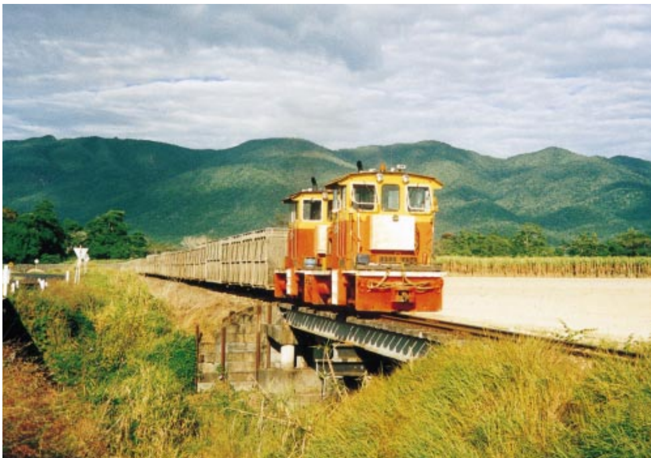
With a dark rainy sky as a backdrop, multi-paired Com-Eng 0-6-0DH locos Nos 15 & 12 (AK3574 of 1964 & AD1351 of 1961) work north over the Bookal Bookal Creek bridge just south of the junction to the Midgenoo branch with more empty bins from the mill in late 1996.
