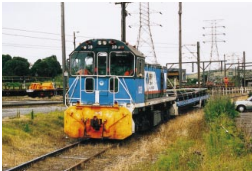
BHP's English Electric (Aust) Bo-Bo DE D39 (A.240 of 1972) passing National Rail's Port Kembla yard enroute for the CRM works, 3 December 1998.
