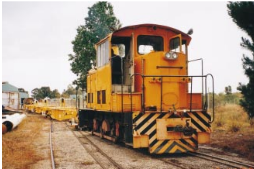
This Tulloch 0-6-0DE (062 of 1970) is used by Goninans for shunting their Basendean plant, seen here on 13 November 1998.
