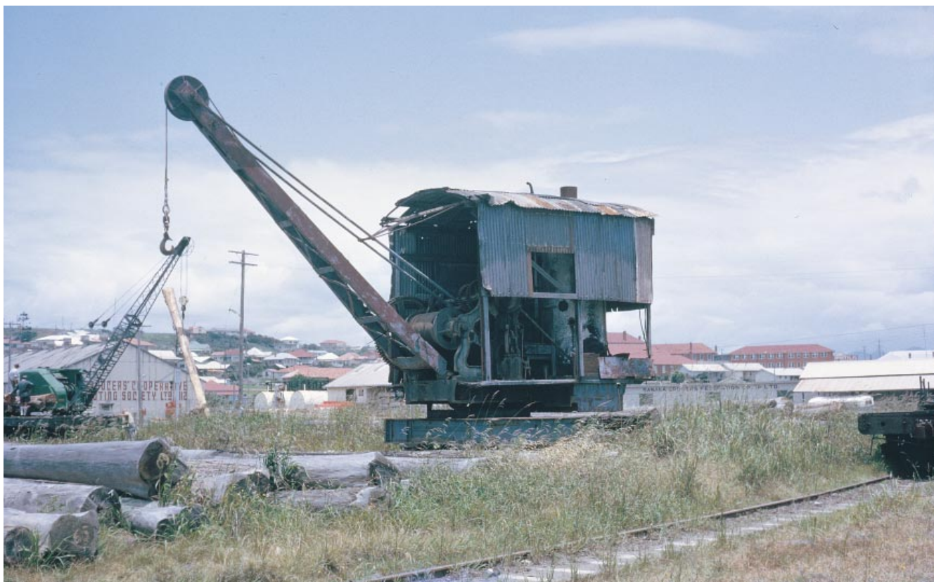
MSB Crane No.4 was a travelling steam crane built by Thomas Smith of Rodley, England, in 1912. In December, 1963, it was found sitting idle in its usual haunt, the area known as the Southern Timber Ramp. Photo: Bruce Belbin
