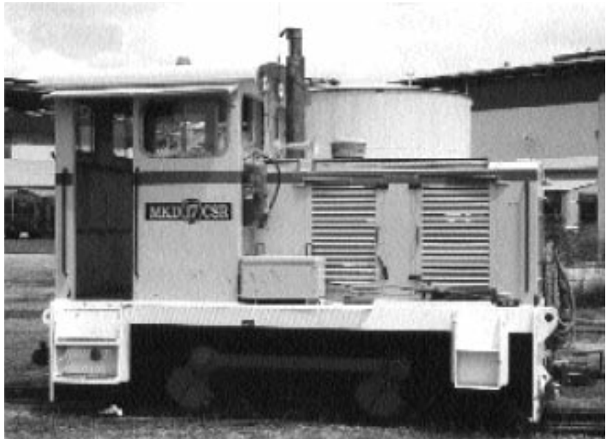
One of several ex-NSW locomotives on the CSR Herbert Valley's cane lines is Macknade Mill's E M Baldwin 0-4-ODH 17 (6-1446-1-9-65 of 1965), first delivered to Condong Mill, near Murwillumbah, as their number 2. As a spare loco, this small unit still sees some cane haulage each year.
