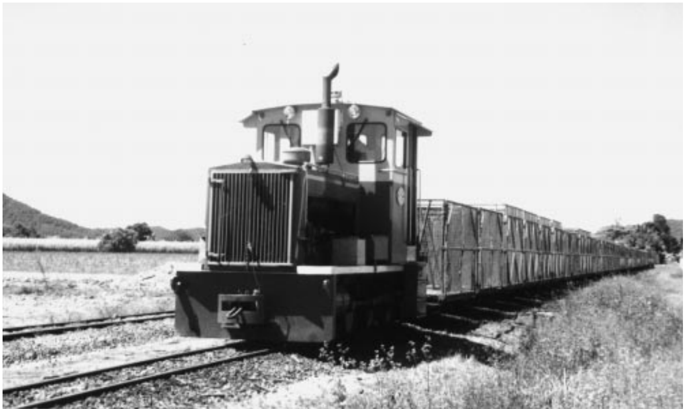
Standing at Midgenoo on 3 September 1996, Com-Eng 0-6-0DH No.11 waits to head back to the El Arish main line and the sugar mill with a load of chopped cane.
