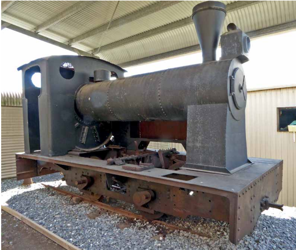
Remains of the Kerr Stuart locomotive B/N 685 of 1900 as displayed under cover at the Beaconsfield Mine Museum, 27 February 2018. Some detailing parts have been fitted. Fortunately, when viewed from the far side, the side tank disguises the incongruous absence of a fire box.
