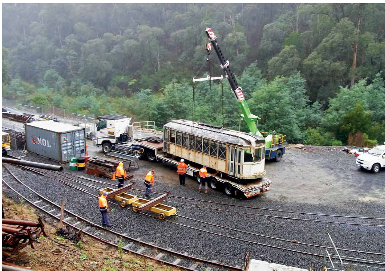
The X1 tram arriving in the yard at Thomson. Since arrival, the ends have been removed and the manufactured underframe and bogies have also arrived at Thomson. Photo: Rob Morton
