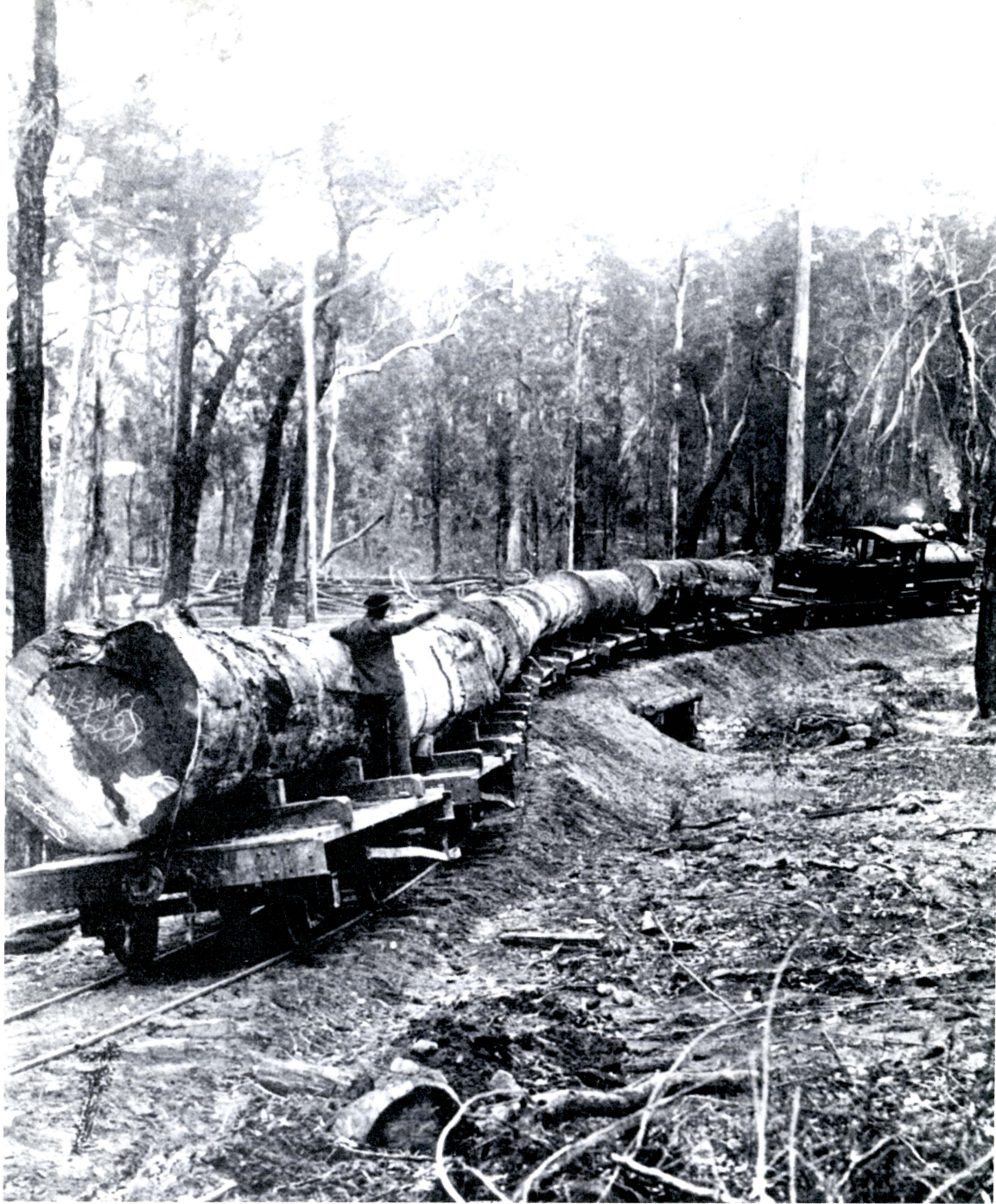
A train of karri logs totalling 34000 super feet of timber, in the Denmark Hills. This photograph was probably taken on the timber tramway running north out of Denmark. The locomotive is a Baldwin 2-4-2ST&T, the date — about 1896.
