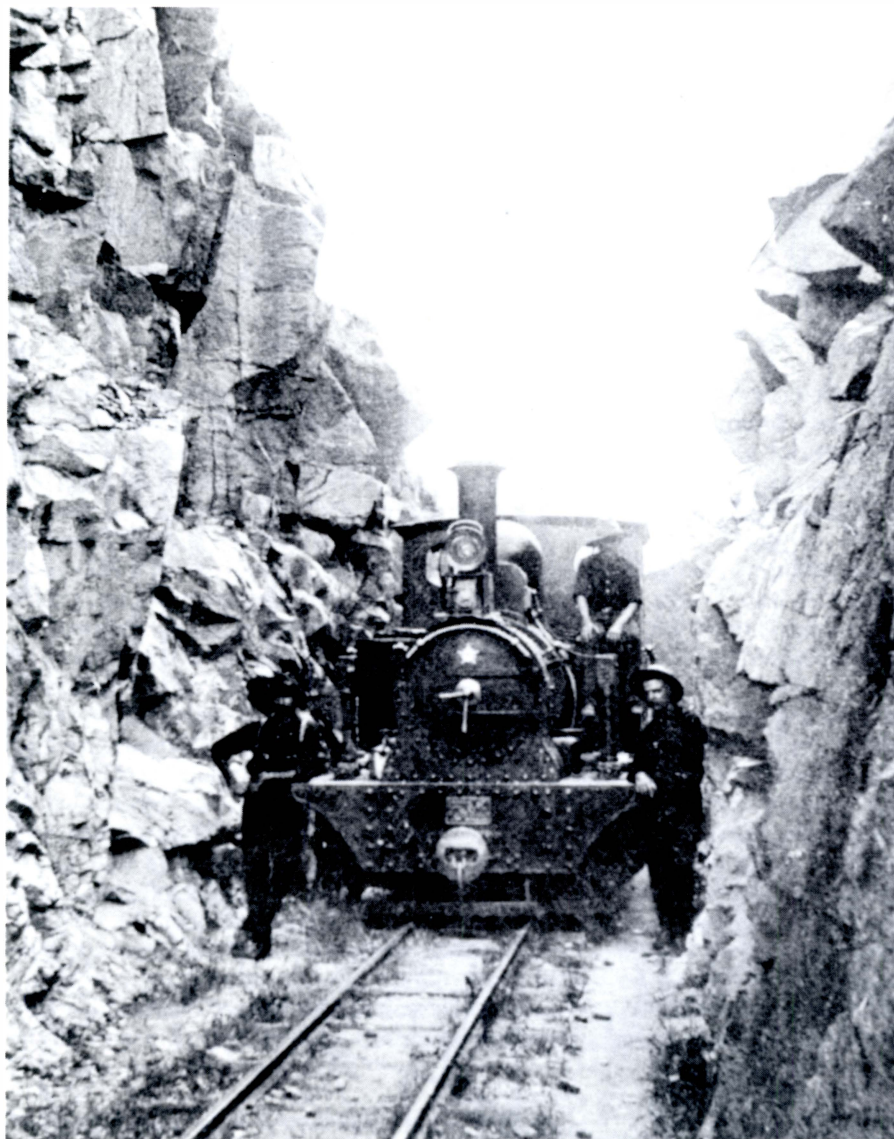
Irvinebank 2 foot gauge tramway locomotive No. 3 Old John , an Avonside 0-6-2T built in 1907.
