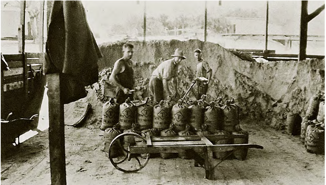
Black sand concentrates were air-dried in heaps on the treatment plant floor. The shed crew filled paper-lined jute bags with one hundredweight (50kg) of sand apiece. Filled bags were wheel-barrowed outside to the loading platform, ready to be taken by motor lorry to Maclean wharf. Bill Derrick collection
