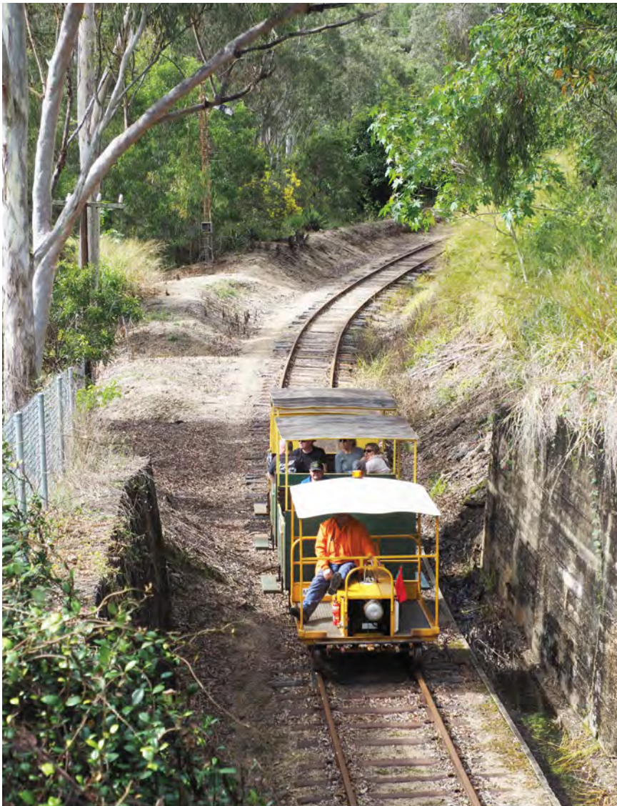
Top: The Atherton-Herberton Historic Railway offer rides on the “Tinlander”, consisting of a pair of section cars top-and-tailing two trolleys converted with seating for passengers. When the train is full, passengers sit on the seats in front of the driver and observer, facing backwards. The “Tinlander” is seen here departing Herberton on 17 July 22. Photo: John Dennis
