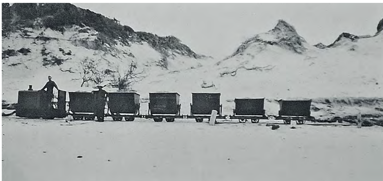
The small Deutz diesel locomotive (Bn 18306 of 1937) posed with six loaded side-tipping mine skips on Porter & Derrick's beach tramway on Pippi Beach in 1937. It faces a 2 km trip south along the beach to the treatment plant. There is no shelter for the driver. He, like the labourers wielding shovels on the beach, was expected to work in all weathers. Bill Derrick collection
