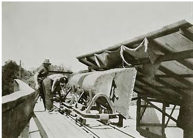
A pair of side-tipping tramway skips have just dumped their loads of raw black sand into the plant's feed hopper. A small belt elevator inside the hopper transferred sand into the plant to be separated by the Wilfley Tables. Bill Derrick collection
