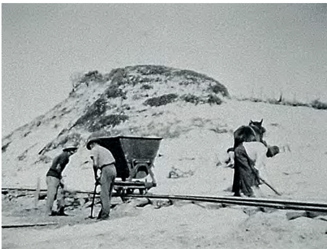
A horse scoop was used to clear beach sand off black sand deposits at Yamba, but all loading work was done by men wielding shovels. Bill Derrick collection
