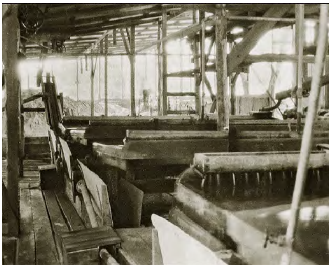
The treatment plant had four Wilfley Tables. Black sand concentrates were shaken off the near side of the tables into side troughs and sluiced down to the small elevator stacker visible in the background. A large pile of air-drying concentrates is visible behind the stacker. Bill Derrick collection
