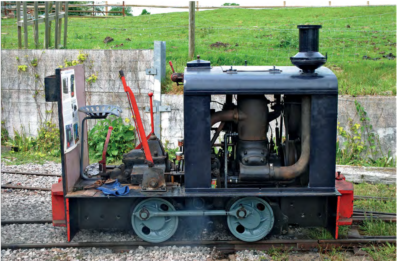
Deutz Bn 19531 of 1937 is preserved in running order at the Amerton Railway in Staffordshire, England. It is one of Deutz' Model OME117F diesel locomotives, the same as TAMCo's Bn 18306 of 1937, and it was also outshopped from the Cologne, Germany, works in March 1937. John Browning collection
