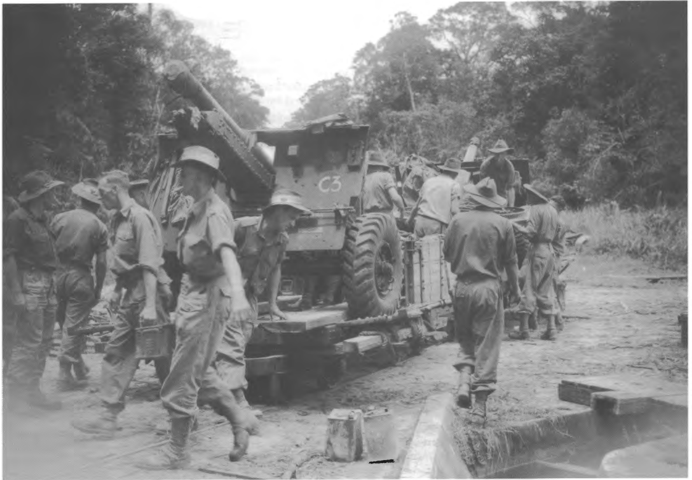
A train has arrived at Seria and the soldiers have begun to unload supplies. The modifications made to the bogie wagons to accommodate the 25-pounder field guns can be seen. Photo: Australian War Memorial No.111517
