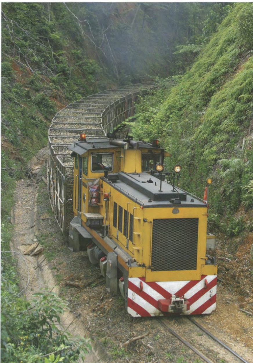
The magnificent sight of South Johnstone Mill's EM Baldwin B-B DH LIVERPOOL (10385.1 8.82 of 1982) powering its train up the Eight Mile Range from Japoon on 26 September 2006. Bundaberg Sugar paints the loco bonnet tops black to reduce reflected glare.
