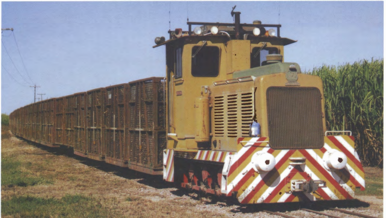
Pioneer Mill's 3ft 6ins gauge Clyde Model DHI-71 0-6-0DH locomotives are an interesting contrast to the narrower design running on 2ft gauge lines. Here MAIDVALE (63-287 of 1963) is pictured on dual gauge track at Klondyke Junction on 1 September 2006.
