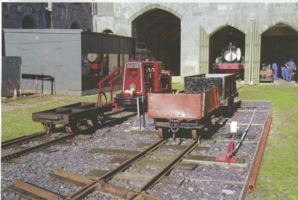
The slate quarry demonstration trackwork at the Penrhyn Castle Industrial Railway Museum with the restored Ruston & Hornsby 20DL 4wDM loco ACON and rolling stock.
