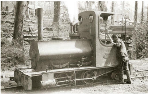
The Powelltown tramway had six steam locomotives. Little Yarra (Baldwin, USA No.37718 of 1912), pictured at left, and Powellite (Bagnall, England No.1965 of 1913), pictured at right, were mainly used between Yarra Junction and Powelltown. Both were bought new by the VPWPL.
