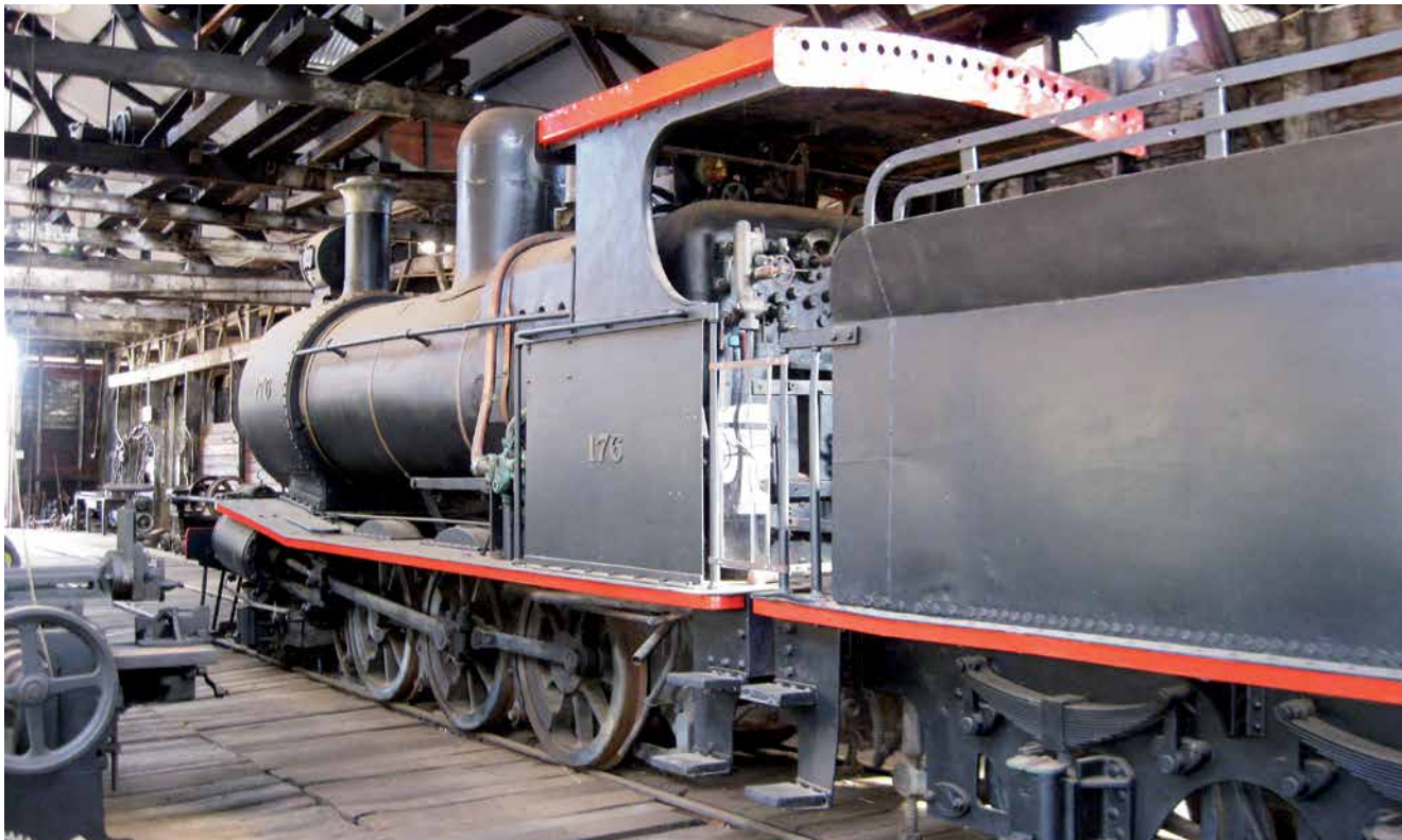
Former South Australian Railways 2-6-0 locomotive Yx 170 taking pride of place on the track amid heavy machines and equipment in the Main Workshop.
