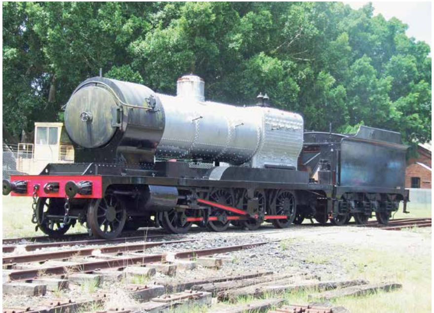
Richmond Vale Railway Museum's cosmetic restoration of ROD 23 continues, with the boiler back in place on the frames. Photo: Graham Black
