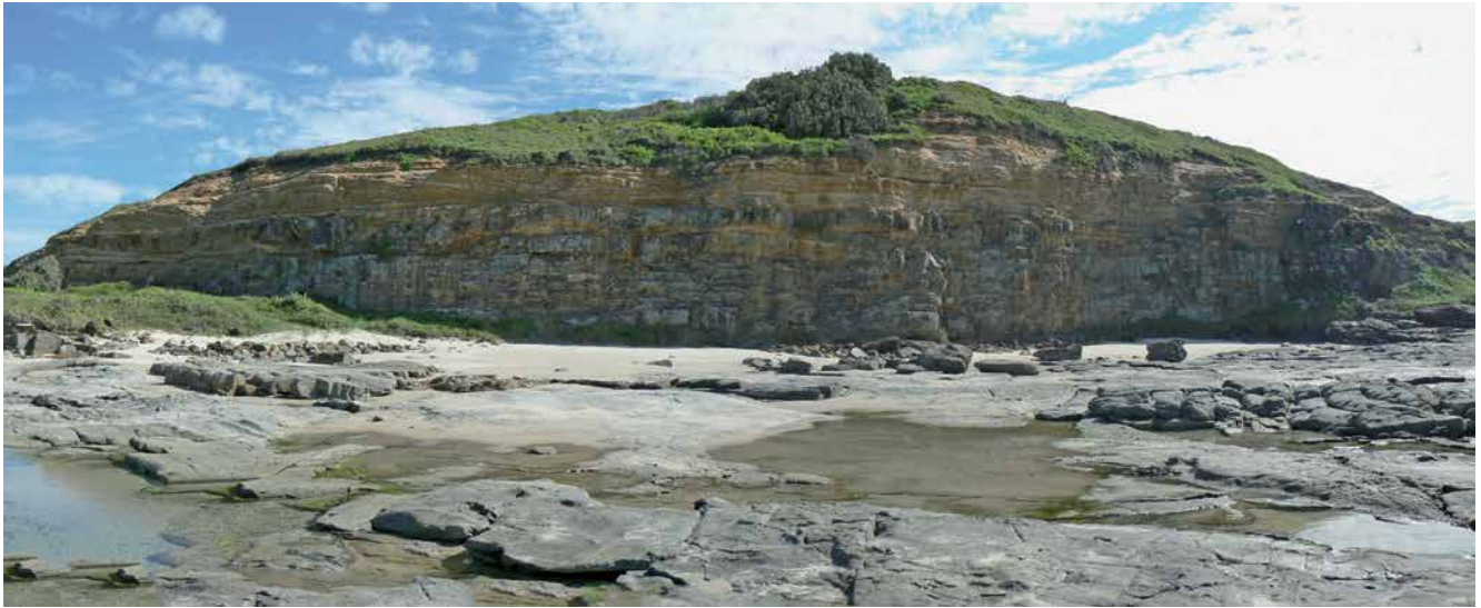
The imposing headland quarry face of the short-lived Iluka Bluff Quarry. Although there was a large quantity of hard blue sandstone available, it could not be quarried out in sizes large enough for breakwater construction. Photo: Ian McNeil
