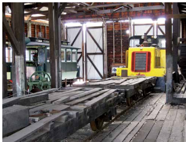
A scene inside the locomotive shed with the Clyde 0-6-0DH locomotive (B/N 61-241 of 1961) at the head of a rake of flat-top timber-carrying wagons on the right and the Baldwin steam tram replica built by Colin Fry to the left. Photo: Robert F McKillop
