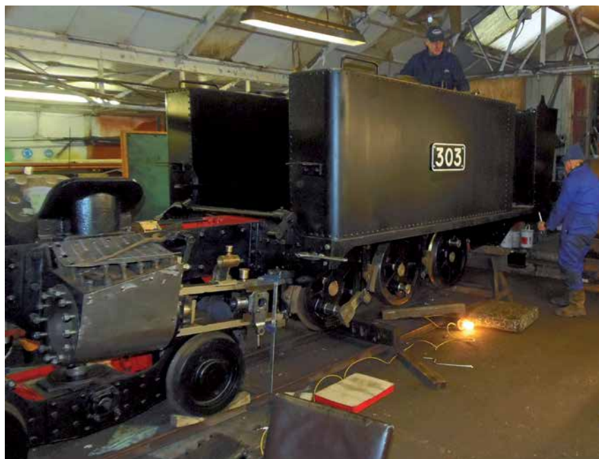
Carrying its service number plate, the left hand tank joins the frames as the jigsaw that is Hunslet 1215 comes together.
