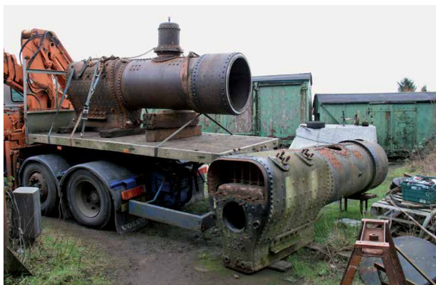
Out with the old, in with the new. The Bundaberg (on the ground) and newly constructed boiler for Hunslet 1215 of 1916 together as another restoration milestone is achieved.
