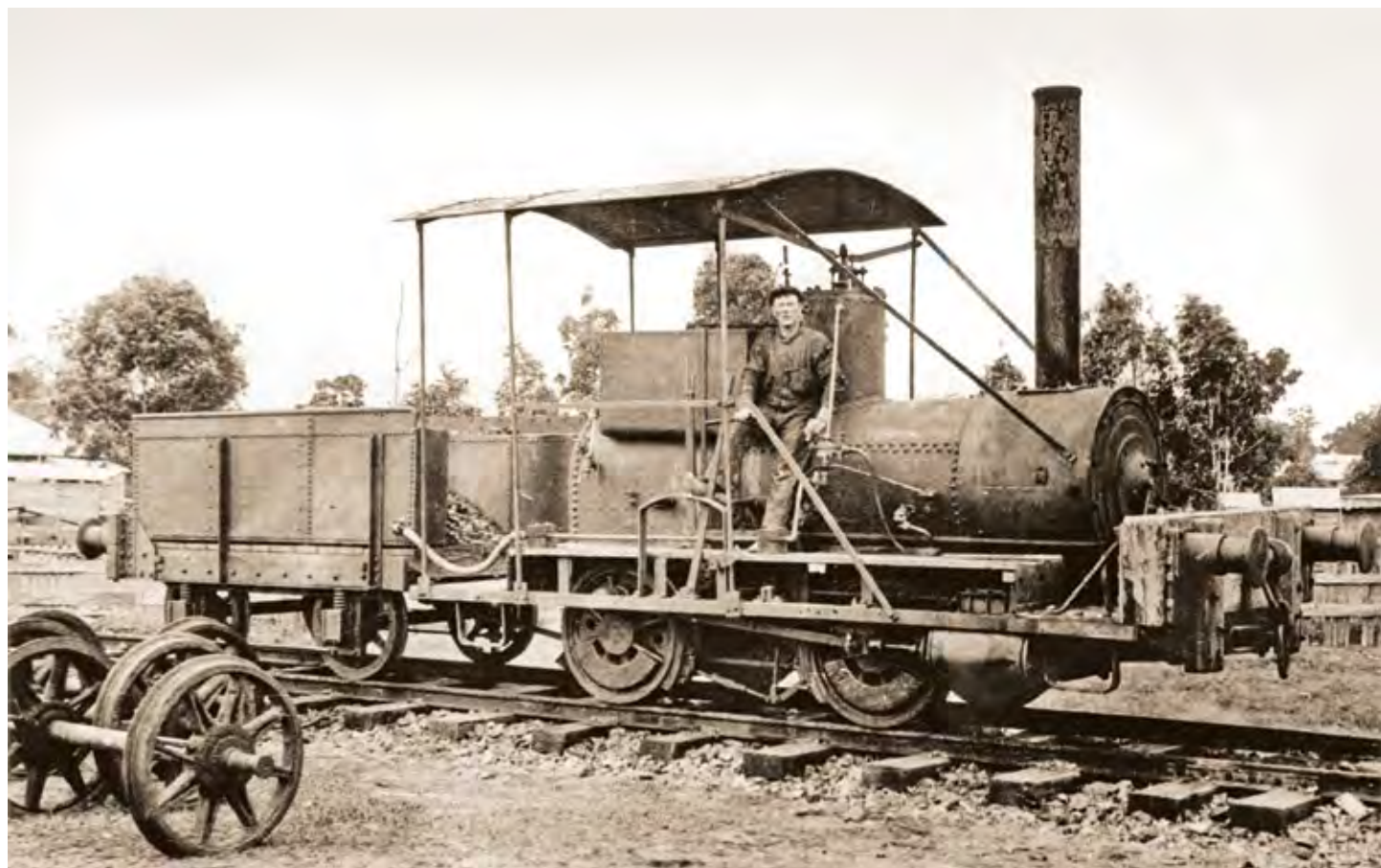
Above: Un-numbered and stripped-down ex-steam tram motor towing a 4-wheel tender working on the North Coast of NSW. The central driving position suggests it was of an early design. Photo: Unknown. Top: Australian Smelting Corporation Ltd locomotive, Andrew Barclay & Co, builder's number 790 of 1897, while on hire to the PWD near the eastern breakwater – date unknown. Photo: R T Horne collection.
