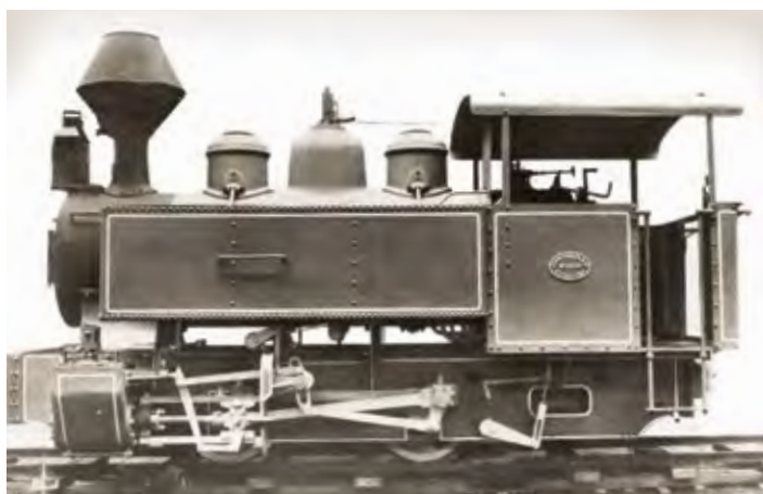
ONE OF THE FIVE-TON locomotives of the British Electric Vehicles Ltd., used to haul trucks of rock and earth from the tunnels driven through the hills for the outfall sewer.
