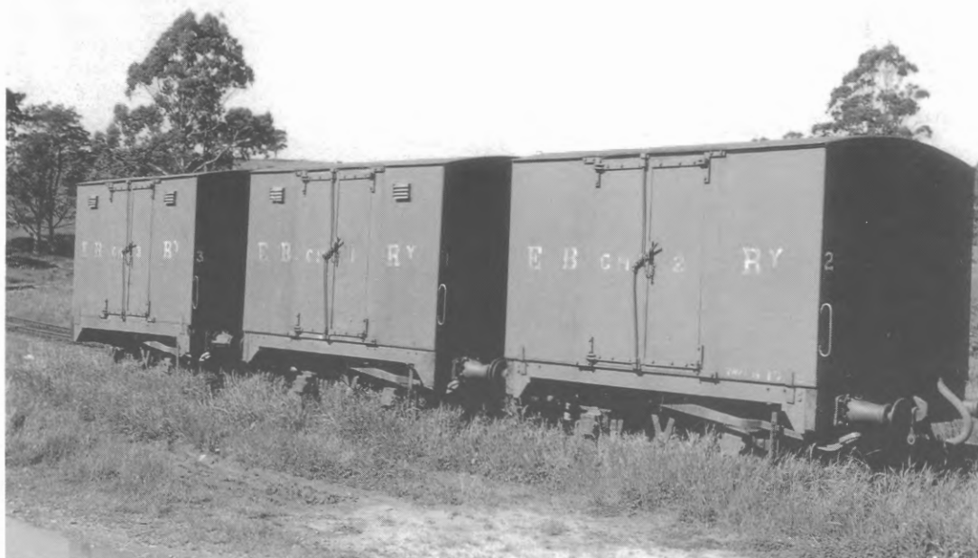
Emu Bay Railway 4-wheel steel goods vans Nos. 3, 2 and 1 built on the underframe of Hurst Nelson hopper wagons ex-NMLR. Photo: HJW Stokes
