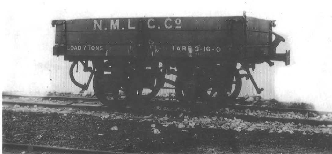
A 4-wheel open wagon built on the underframe of a Hurst Nelson hopper wagon c.1902. No record has so far been found of its class or running number. State Archives, courtesy Lou Rae
