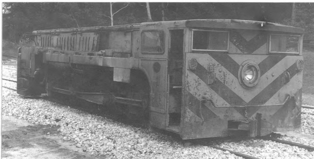
Malcolm Moore/Drewry 0-6-0DM underground locomotive at Clarence, 30 October 1987, shortly after delivery to the Zig Zag Railway Cooperative.
