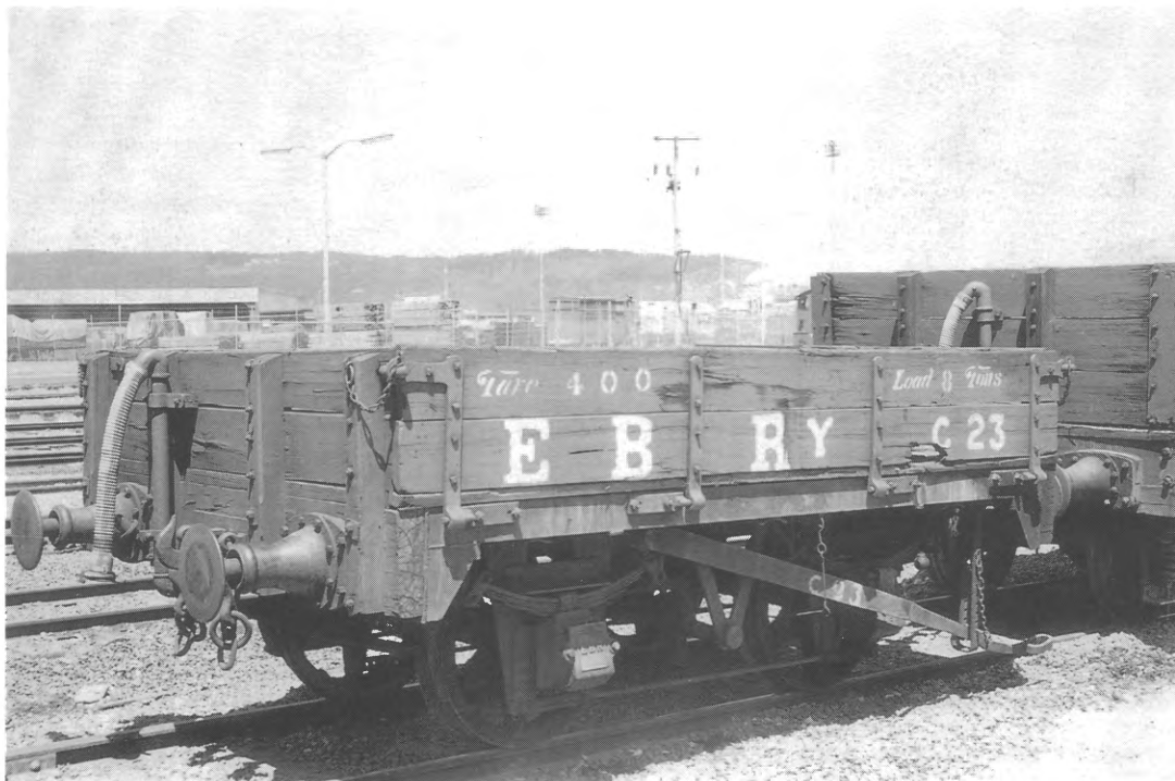
Emu Bay Railway 4-wheel wagon C23 was built on the underframe of a Hurst Nelson NMLR hopper wagon and looks much like the NMLR's own 4-wheel open wagon. Photo: HJW Stokes
