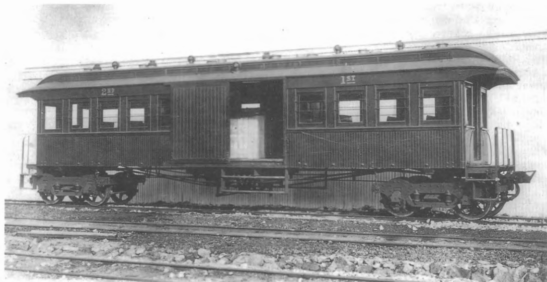
Brake composite passenger carriage as converted by the NMLR c.1903 from an ordinary composite vehicle. State Archives, courtesy JL Buckland
