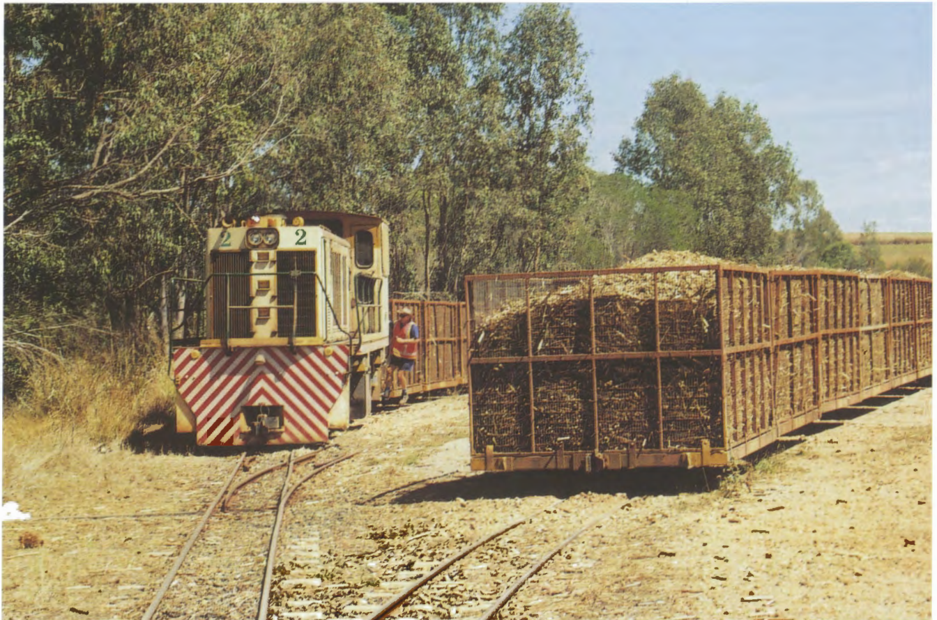
The main loading yard for road hauled bins from Booyal and beyond is Adie's, where Walkers B-B DH ISIS No.2 (598 of 1968 rebuilt Walkers 1994) was shunting in the spring of 2004.
