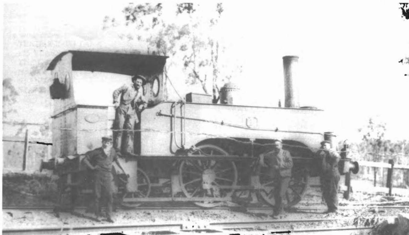
J&A Brown locomotive number 1 (R&W Hawthorn 947 of 1856) was one of two 0-4-2T machines originally purchased by John Eales to operate his Minmi to Hexham Railway. Photo: John Buckland Collection
