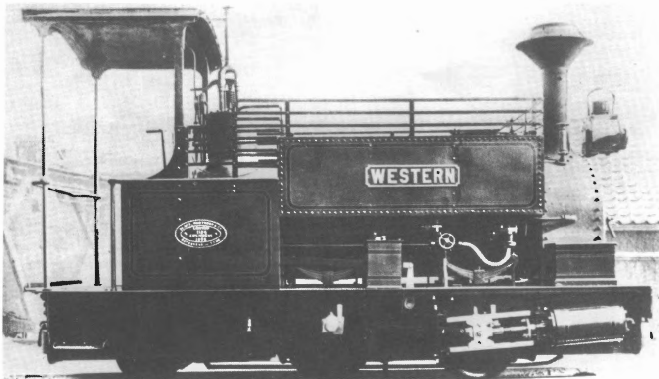
The builder's photograph of Black Hawthorn & Co. 0-4-2T 1134 of 1897, WESTERN .
