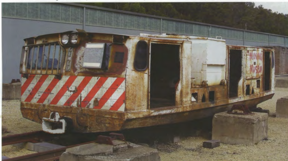
The Gemco miners' transport car displayed in its mine operating condition on 1067mm track laid near the State Mine Downcast Shaft in March 2007. Photo: Ray Christison
