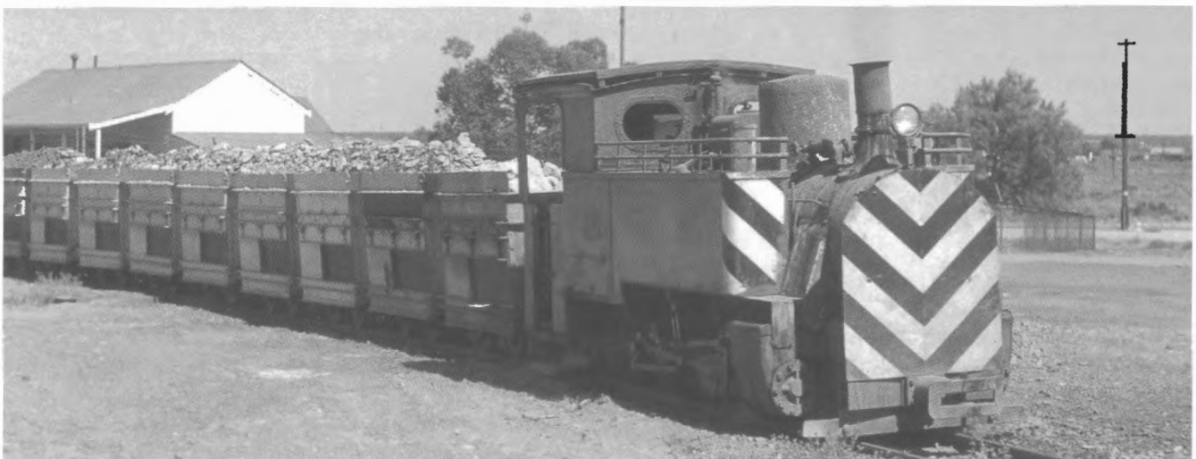
Ian Cutter took this photo of one of the Lake View & Star mine's Orenstein & Koppel 0-6-0T locomotives heading an ore train at Kalgoorlie on 1 March 1962. Can any reader provide further identification of this loco and the reason for the adornment on the smokebox and side tanks?
