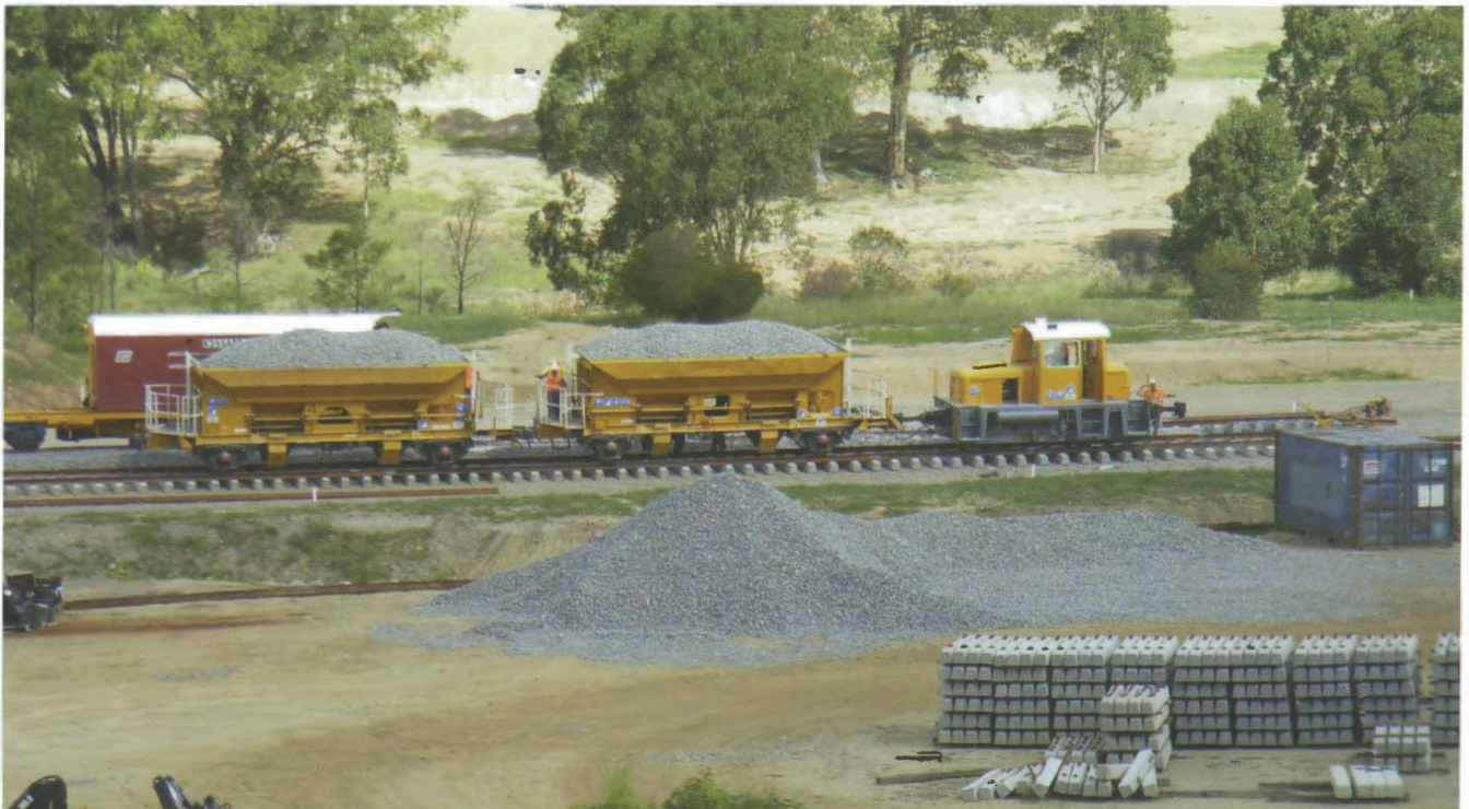
This small standard gauge 4wDH shunter of German manufacture has recently been imported to NSW from Hong Kong for use by the BT Contractors – iQR Alliance. It is seen at Drayton Junction on 21 March together with two ballast hoppers that are believed to have come from the same source. Photo: Ray Cross
