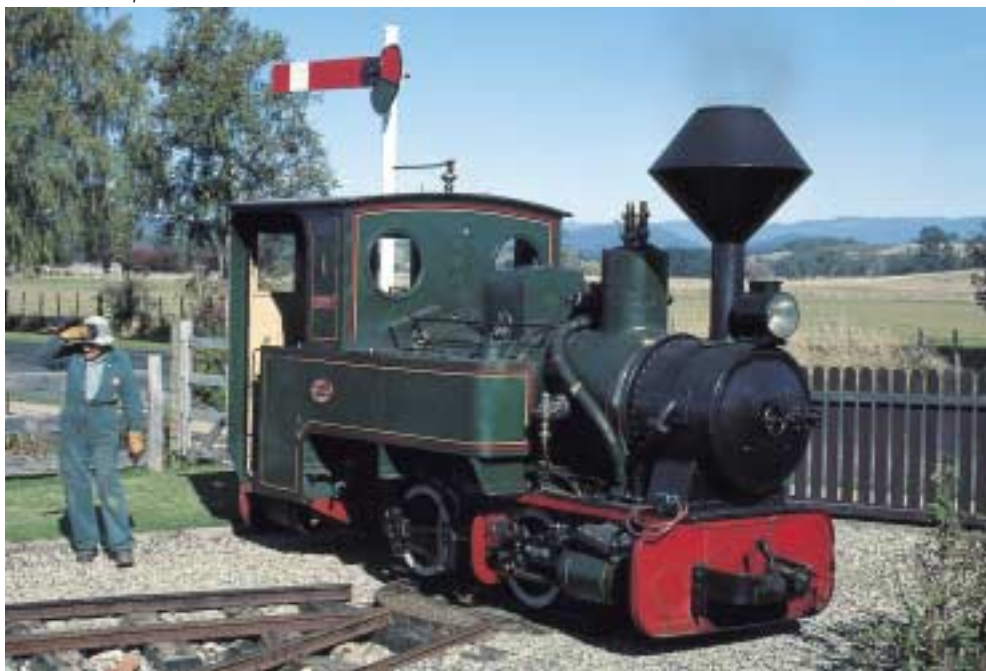
On Tasmania's Redwater Creek Railway, in April 2000, composite Krauss 0-4-0WT (5800/1907 & 5682/1906) makes use of the tiny turntable at the Sheffield end of the line. This locomotive will be out of action for about two months from June 2001, while its boiler is removed for a full inspection. Photo: Peter Charrett
