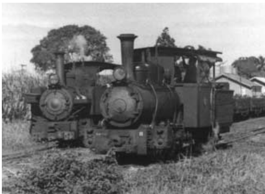
On the Innisfail Tramway, in September 1955, B9 1/2 class 0-6-2 number 11 (JF 17110/1926) waits in the loop near Mourilyan township as 6D8 1/2 class 0-6-0T number 8 (JF 15939/1923) passes with a train of empty 'H' wagons from Mourilyan Harbour.
