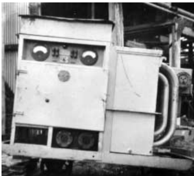
A 3ft 6in gauge wheel mounted underground transformer stored at the colliery in 1962. Photo: Brian Andrews
