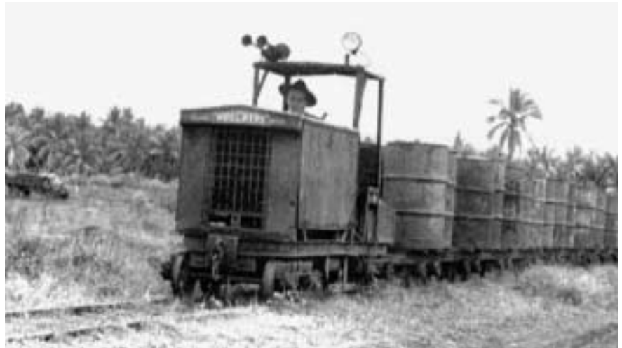
The unusual 4-2-0 internal combustion locomotive in action, hauling a load of 44 gallon drums on the Merauke airfield tramway. Photo: Australian War Memorial
