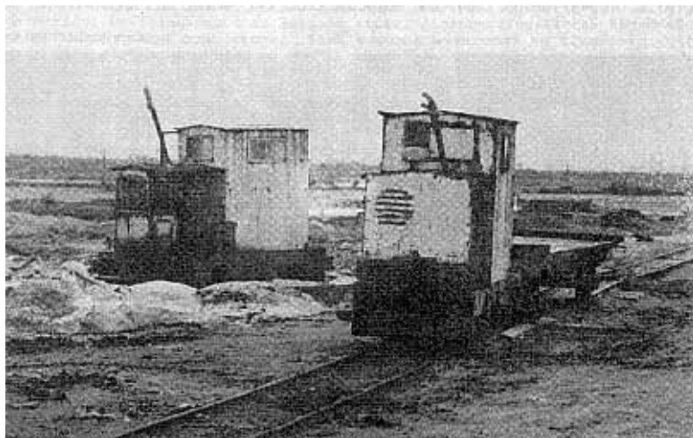
Ruston & Hornsby No.4, 320555 of 1951 (left) and No.1, 252805 of 1949 (right) at Cheetham Salt Limited's Laverton works on 21.8.88. (The gloves on the exhaust pipes are to keep water out of the exhaust manifolds and engine head.)
