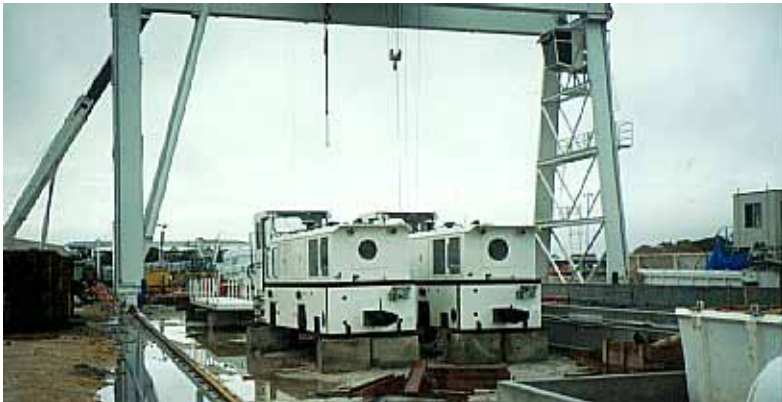
Two 900 mm gauge Schöma four-wheel diesels at the Airport Link tunnel construction site at Tempe, NSW. February 14th, 1997.
