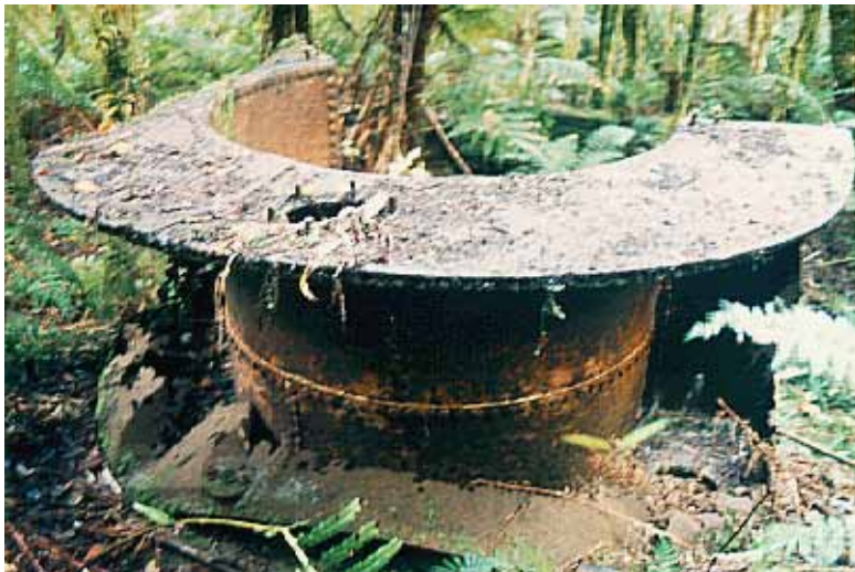
Water tank off one of Sanderson's vertical boilered loco/winches, Barramunga Creek Mill, June 1993.
