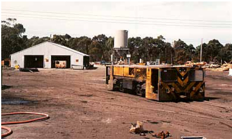
E.M. Baldwin 4wDH 25-tonne mining loco 10597-2 of 1984 on the surface at Chain Valley Colliery, while Titan battery electric personnel car EMT 1005 of 1979 looks on from the shed.
