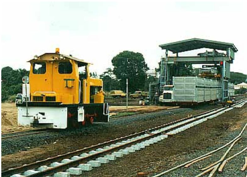
South Johnstone Mill's Com-Eng 0-6-0DH 19 (AH4688 of 1965) was shunting 14-tonne bin containers for Atherton Tableland cane at the new transfer gantry on 24 August 1995. Note the new main line track construction in progress on the adjacent line.
