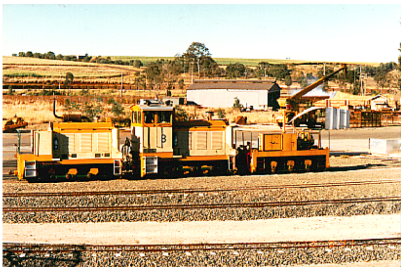
Coupled 0-6-0 Clyde units with cab removed from slave unit, and brakewagon at Isis Mill on 12/8/92.
