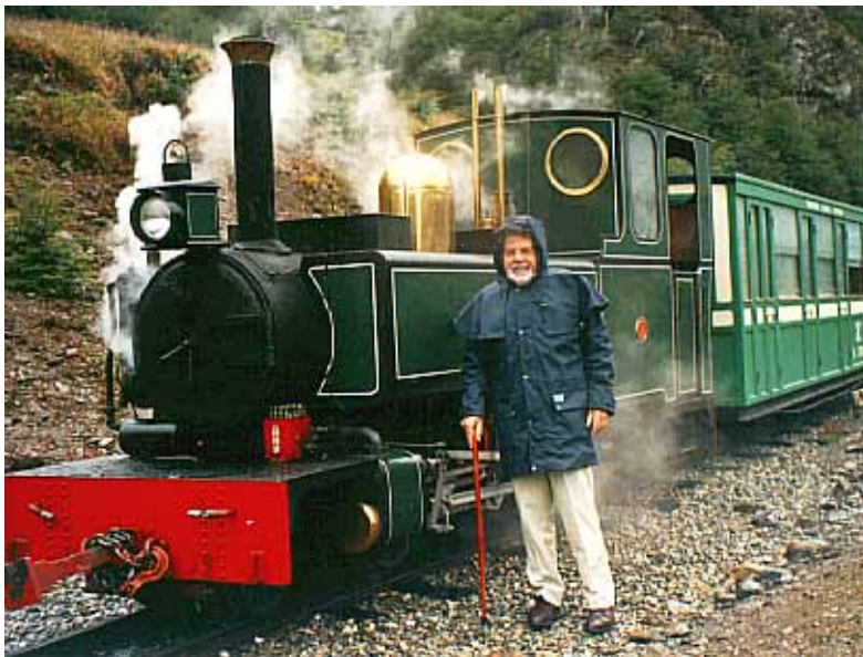
The Train to the end of the World, headed by 500 mm gauge Winson Engineering 2-6-2T CAMILA (15 of 1995), waits at a passing loop, January 1997.
