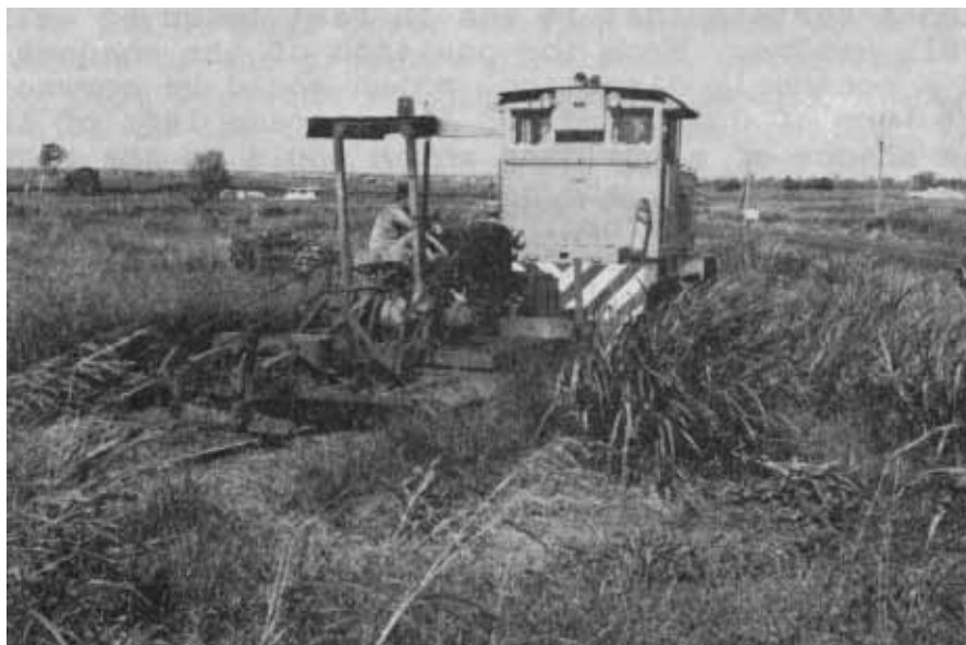
Millaquin Mill's 11903, E.M. Baldwin B-B DH 6456-1-11-75 of 1975, hauling the mill's grass cutter, a tractor mounted on a four-wheeled wagon chassis. 3 March 1978
