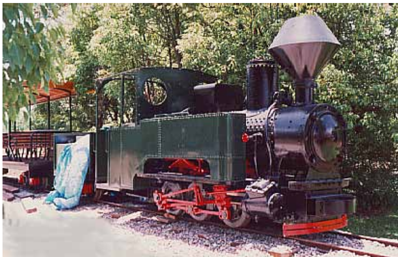
Krauss 0-6-0T Moreton (4679 of 1900) with carriage, prior to completion of the conversion of motive power.
