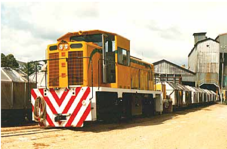
Ex QGR 2 ft gauge Walkers B-B DH 605 of 1969 with brake wagon and sugar boxes at Victoria Mill, August 1991.
