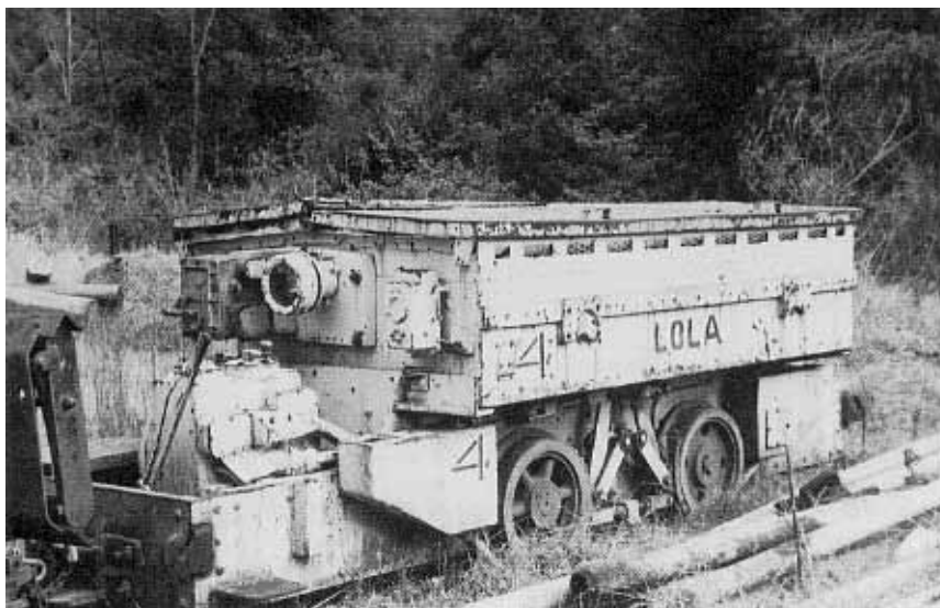
Lola, Atlas 10 ton four-wheel battery-electric locomotive, out of use.
