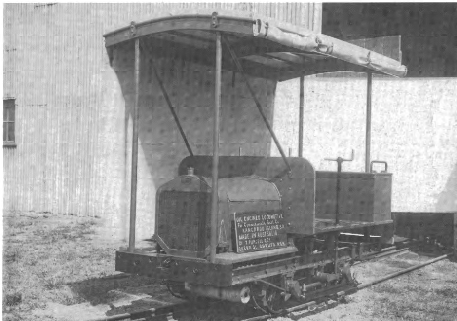
Below: Builders photograph of the Purcell inspection truck used on the Salt Lake to Muston tramway. Cheetham records show this unit to have had a petrol motor so the oil engine must have been replaced.
