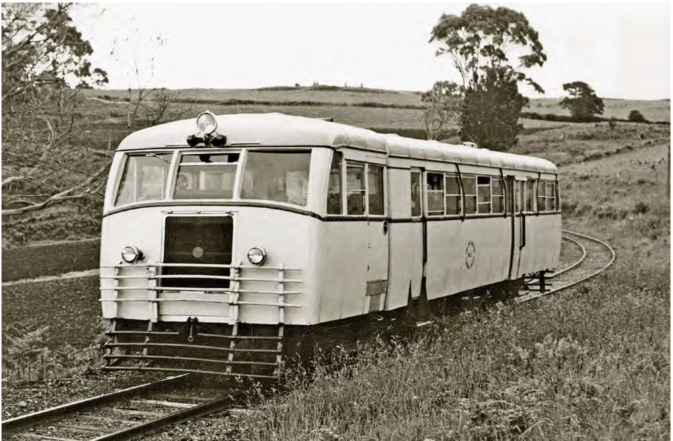
Below: The EBR's Walker rail motor, WG1, incorporated a 153hp Gardner diesel engine. The riding qualities were said to be the best of all the Emu Bay's rail motors, though that could be partly the result of better track standards by the time it was in service. With the more powerful motor, it had no difficulty in hauling the light trailer PT2 but not a heavier trailer with which it was originally tried. Included 2+3 seating at the front and 2+2 seating in the rear section. Intended for the growing West Coast tourist traffic of the late 1930s, its arrival at Burnie was delayed due to the outbreak of war in 1939. Photo: Ted Lidster colln, courtesy Trainiac, Flickr
