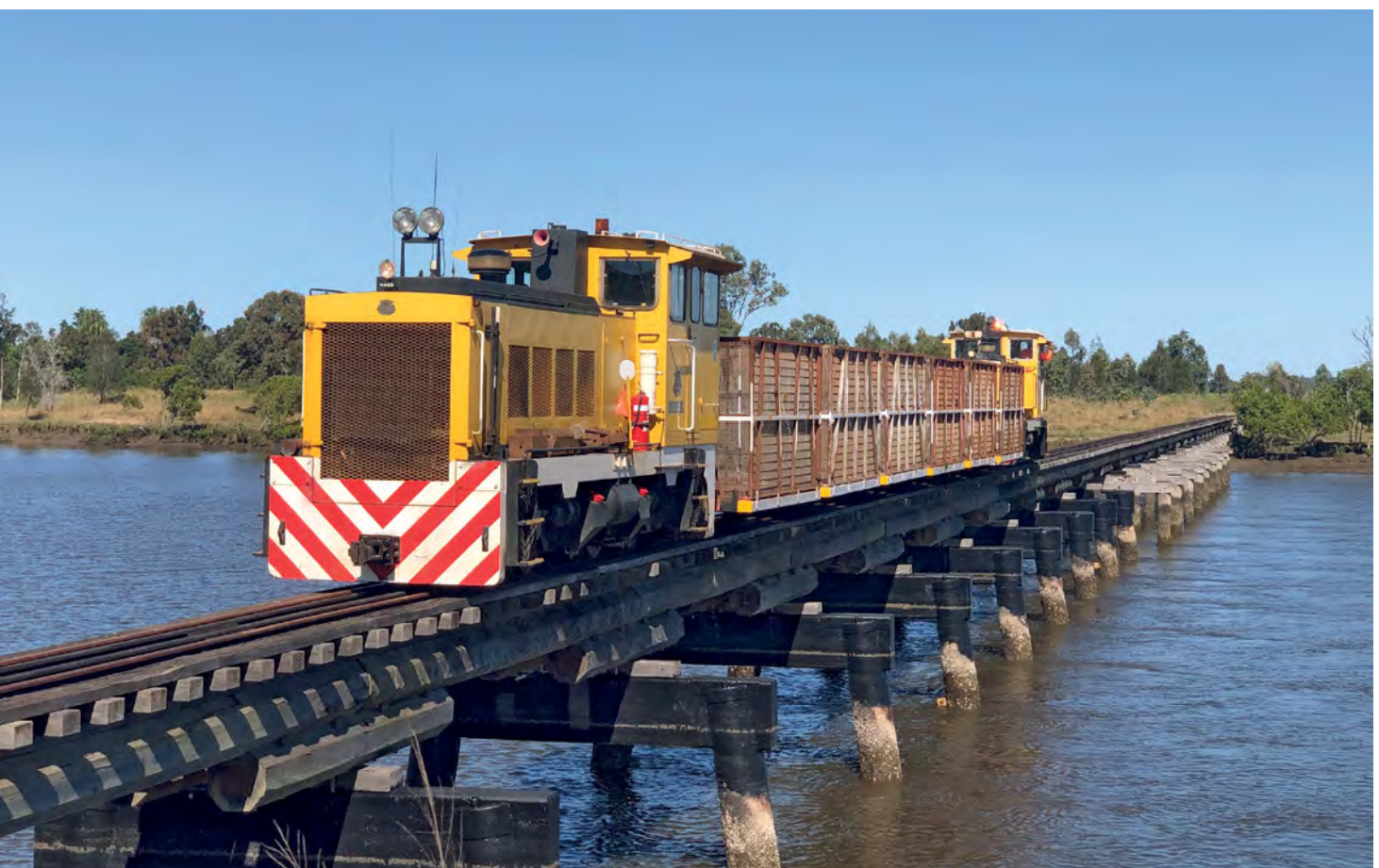
Millaquin Mill's EM Baldwin B-B DH locos Givelda (5800.2 6.75 of 1975) and Moorland (5565.1 10.74 of 1974) test the Booyan Bridge over the Kolan River on the Fairymead system's North Coast line to Avondale on 13 June. Photo: Mitch Zunker
