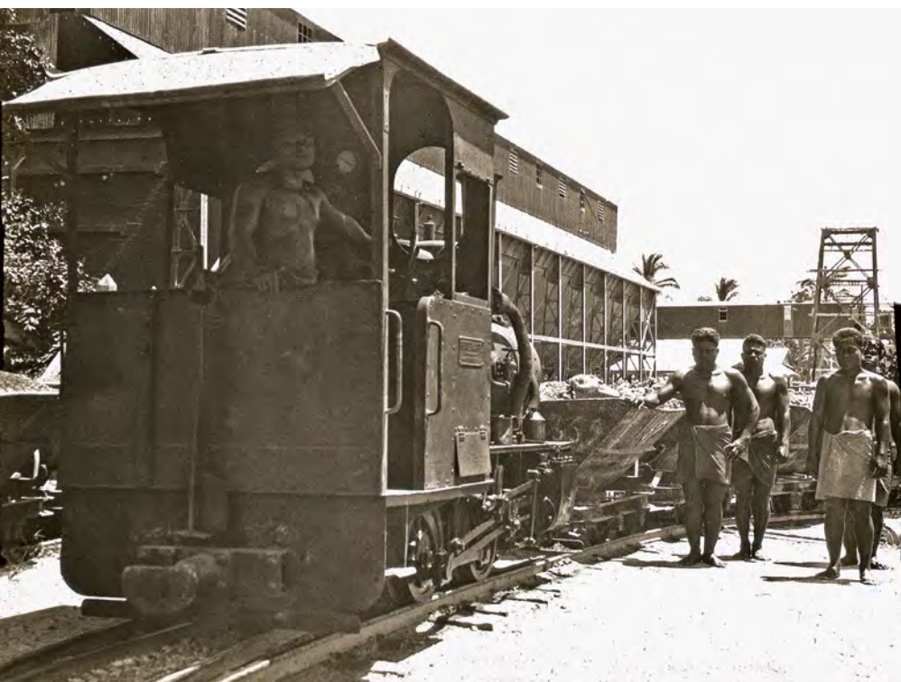
Orenstein & Koppel 20hp 0-4-0WT b/n 10474 of 1923 on Ocean Island. c.1930 Photo: courtesy CLN Archdeacon A N Williamson collection, Special Collections, Auchmuty Library, University of Newcastle ref a5051006
