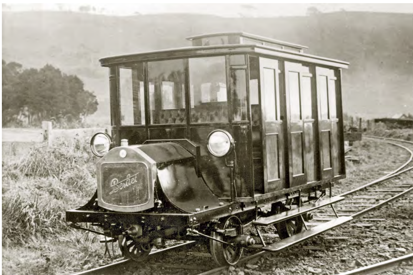
The Berliet-engined rail motor – said to be the second passenger rail motor built – on a trial run in 1916, posing for its photograph. The Burnie Advocate, of 3 October 1917 notes that it weighed two tons, will carry a dozen passengers and can climb a 1 in 16 grade at 15mph. It had a 15hp 4-cylinder engine. The body was made of Tasmanian timbers, the finish being in polished blackwood with sliding doors, the upholstery of American leather and had polished brass foot rests. It was sold to R J Howard at Zeehan in 1950 where it was scrapped and wrecked in the mid-1960s. Photo: Ted Lidster colln. courtesy Trainiac, Flickr
