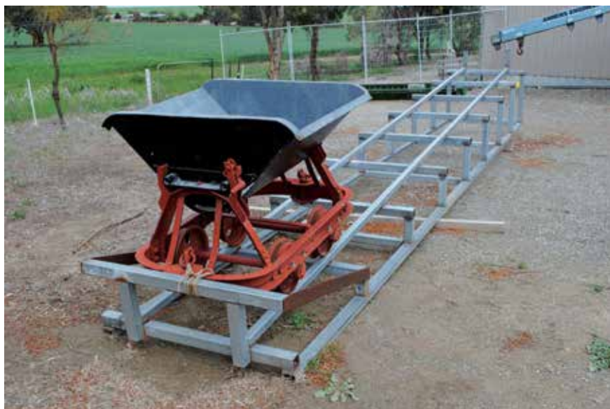
A restored tipper skip displayed outside the Sheoak Log museum building on 29 September. The incline construction, including the rails, is made of square section tubular steel. Photo: John Browning
