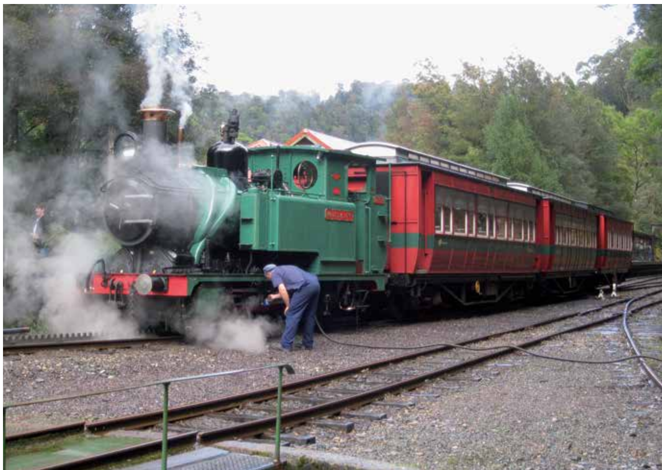
The driver of the 'Rescue Train' oils round MOUNT LYELL No.1 at Dubbil Barril amidst the gloom of the rainforest and overcast sky. The loco is taking water from the hose while the turntable is in the foreground. From this station the locomotive engages the Abt rack for the very steep climb of 1 in 20 up to Rinadeena which is the summit of the rack section.
