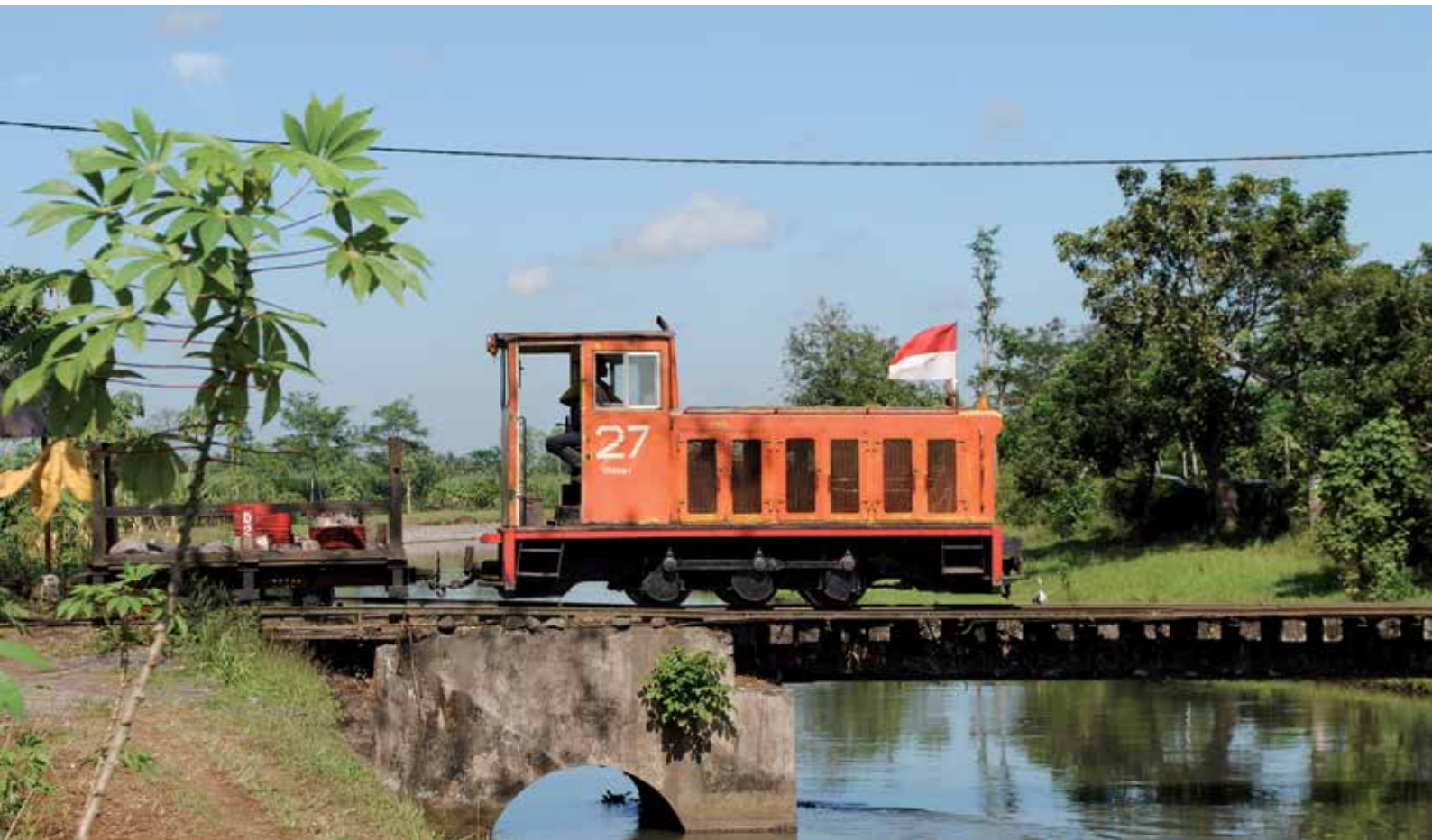
Jatiroto Mill's Hokuriku Juki Kogyo 0-6-0DH 27 (2420-09 of 1976), sporting the Indonesian flag, heads out to the canefields across an irrigation channel on the morning of 21 July. Each main line locomotive at Jatiroto and Semboro runs with a permanently-coupled 'tender'.
