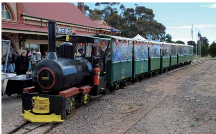
The Moonta Mines Tourist Railway train waits to depart from the old Moonta railway station on 29 September. 2ft gauge track is laid on top of the old 5ft 3in gauge lines. Photo: John Browning
