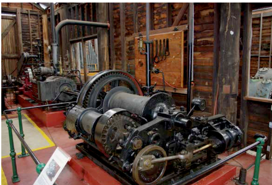
In the once beautifully maintained machinery display room at the Yarloop Workshops, this Clarke Chapman (UK) winch was used for log haulage in the bush, bringing cut timber to the tram lines for transport back to timber mills. Photo: Stuart Thyer
