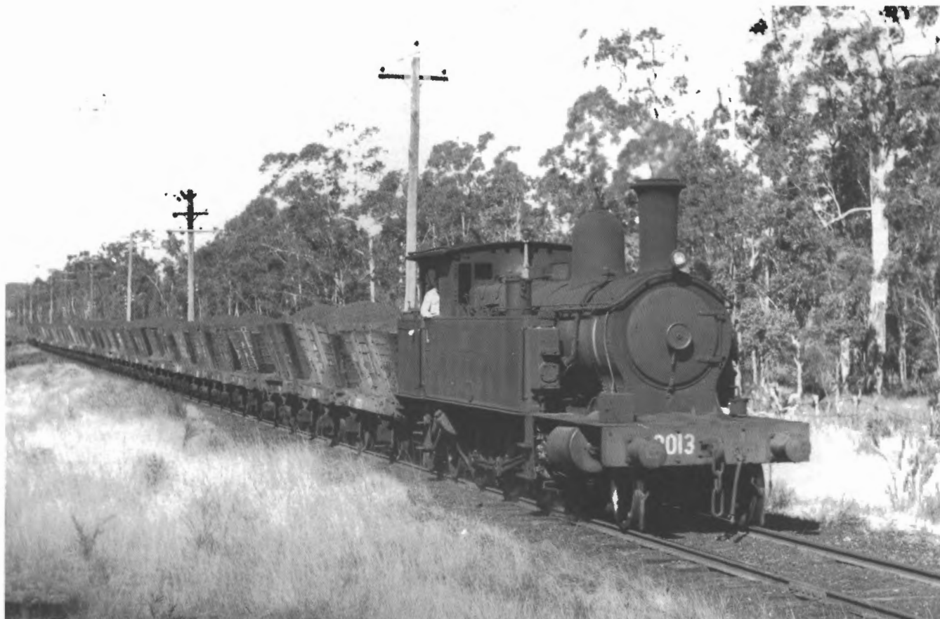
Ex-government 4-6-4T suburban tank engine 3013 (Beyer Peacock 4456 of 1903) was acquired to operate the colliery line following an accident to number 1 in 1967. In its early days on the line, it operated in as-delivered condition, the extra brake cylinders, salvaged from number 1, being fitted later. A rake of non-air hoppers is rolled down the 1 in 89 grade towards Hebburn Dam in 1967. Photo: Ron Preston
