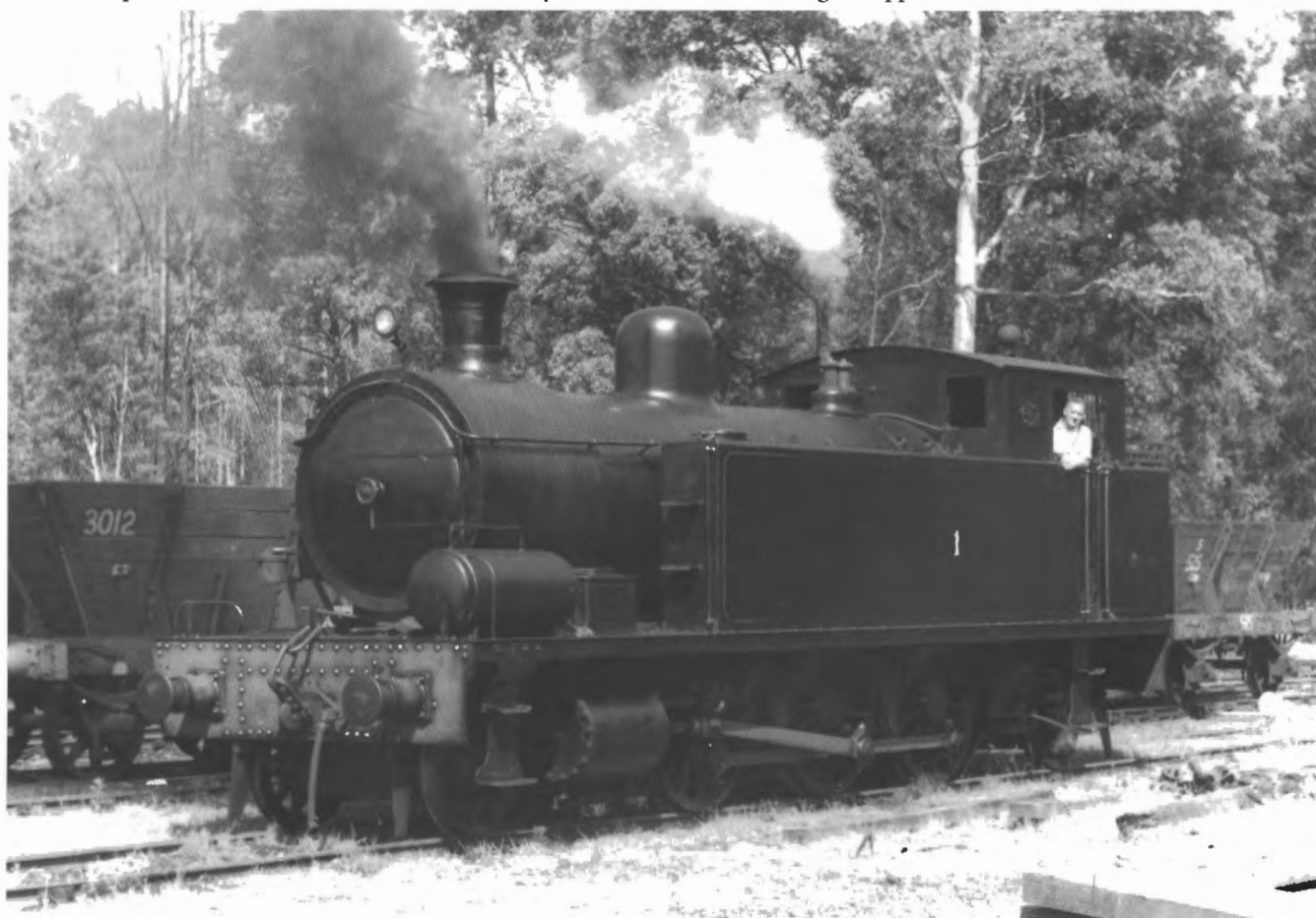
With a design extending back to 1885, Hebburn 2-6-2T number 1 was built by Robert Stephenson and Hawthorn (E7841) and entered service in July 1955. The large air reservoir on the front footplate was part of the braking system.
