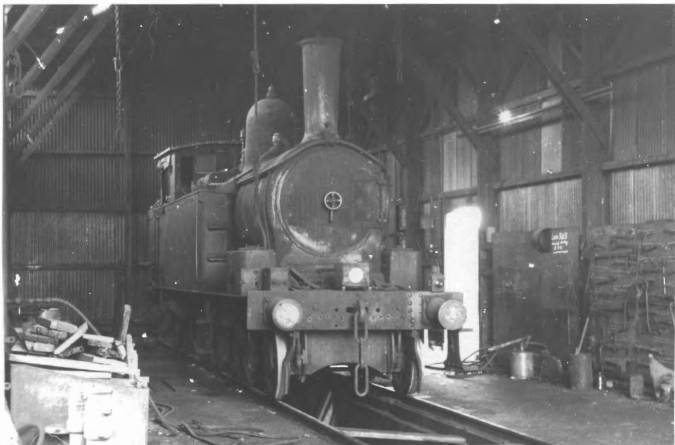
While facilities within Hebburn's engine shed were not extensive, the staff maintained a relatively wide range of locomotives using the spanners, grease guns, jacks and other basics on offer. In 1967, J&A Brown number 26 (Beyer Peacock 2567 of 1890) stands over the shed's pit while 3013 does duty on the line. Photo: Ron Preston
