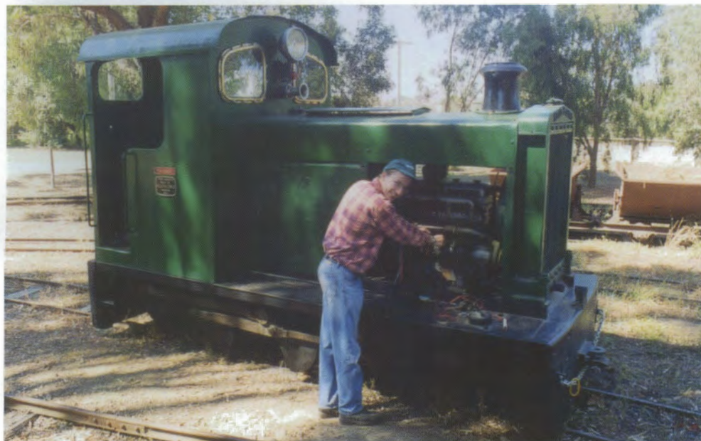
Long standing problems with the generator of the Alexandra Timber Tramway & Museum's ex-Rubicon 0-6-ODM (Kelly & Lewis 4271 of 1935) have finally been remedied by volunteer Carl Hopkins. Photo: Peter Evans
