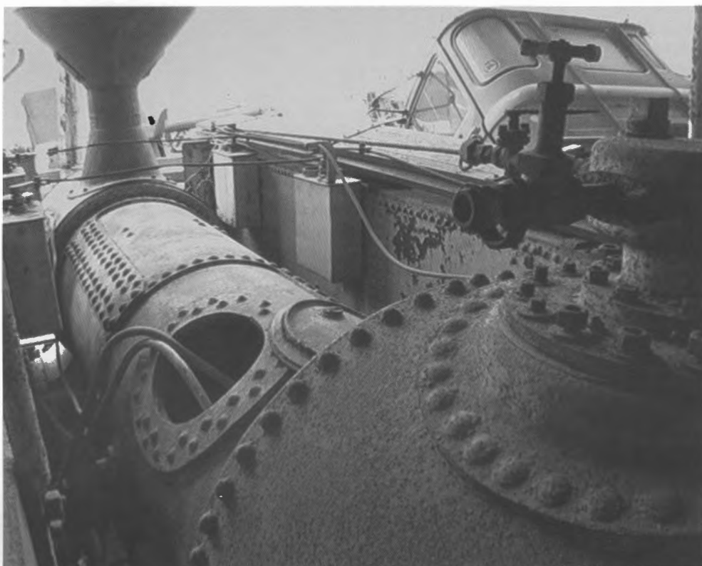
John Fowler 0-6-0T 7607 of 1896 (Ex-Isis Central Mill No.4) was recently advertised for sale. (See News Item p.25). Its riveted water tanks and original style of boiler are well illustrated in this view, taken at its current (May 2004) storage site.
