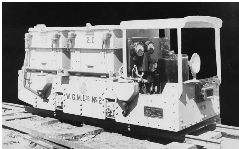
English Electric battery locomotive W.G.M.LTD. No.2, (770 of 1930) ordered by Consolidated Goldfields, for Wiluna Gold Mines.
