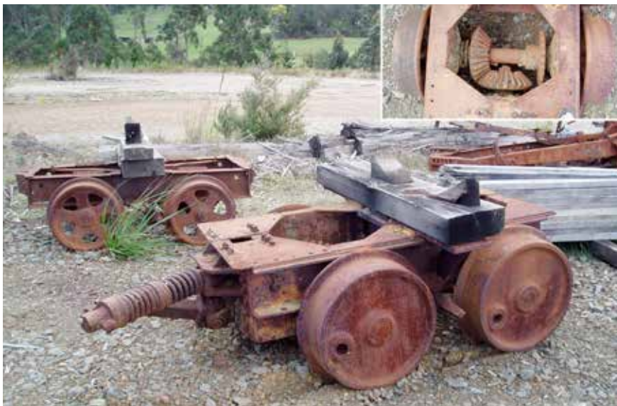
This composite photograph appeared on page 23 of LR 211, and shows one of the original Byers bogies reconfigured as the powered log bogie used behind the Caterpillar . The rod linkages had been removed, but the former holes are evident. The bogie was, for a time, displayed under the front of a log outside Clennett's Dover Mill, but the photo was taken after it had all been taken into the mill site. The bogie in the background was that at the rear of the display, and its wheels appear identical to those in the bogies shown behind the Caterpillar . Photos: JS Clennett, August 2006
