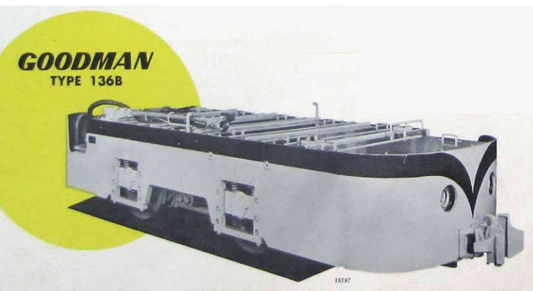
Trolley pole equipped version of the Goodman Type 136B locomotive. Photo: Ross Mainwaring collection.
