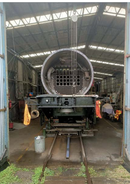
Above: A side view of ASG 33 showing the rear engine unit and boiler cradle under restoration in the Queenscliff workshop of the Bellarine Railway.
