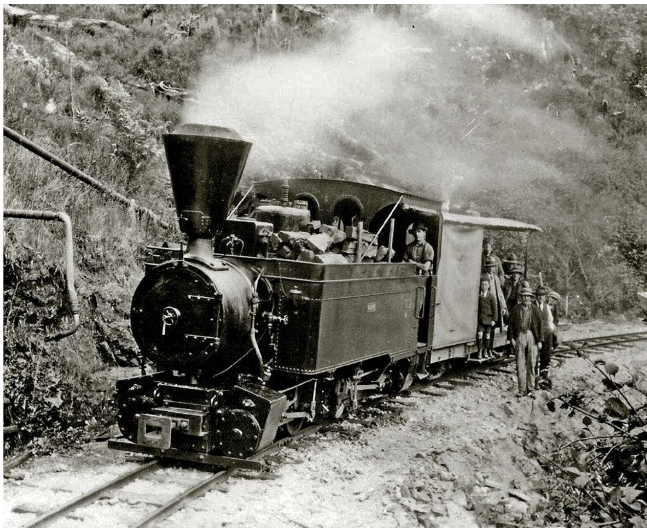
Of all the photographs of the Magnet Tramway's two Mallet tank locomotives, the majority are at this spot, a watering and fuelling location near the Arthur River, and most show the locomotives facing Magnet Junction, attesting to the lack of turning facilities. This photo of Magnet No.3 (O&K 2609 of 1907) is thought to date from the line's later years as suggested by the dress of the people. In our picture, watering has been completed and everyone is paying attention to Jackie Robinson, the well-known photographer from Waratah. Photo: J H (Jackie) Robinson, Wikipedia 28070064140
