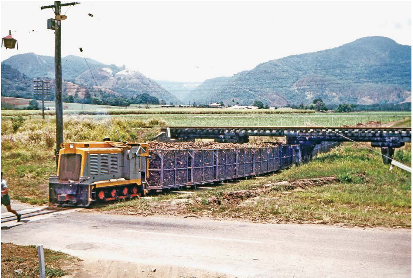
Number 6, one of the five Clyde 0-6-0 diesel-hydraulics built with a fold-down cab, coming under the QR's bridge that carries the Kuranda railway, and crossing Kamerunga Road. Note one of the crew, his head and hat just visible above the cab – he would be standing outside the loco on the cab steps. Red Peak at the right background. The Kuranda railway, after crossing the low-level bridge, will wind its way into the mountains at left and head into the Barron River gorge, just left of middle background. Photo courtesy: www.westonlangford.com/images/photo/108385
