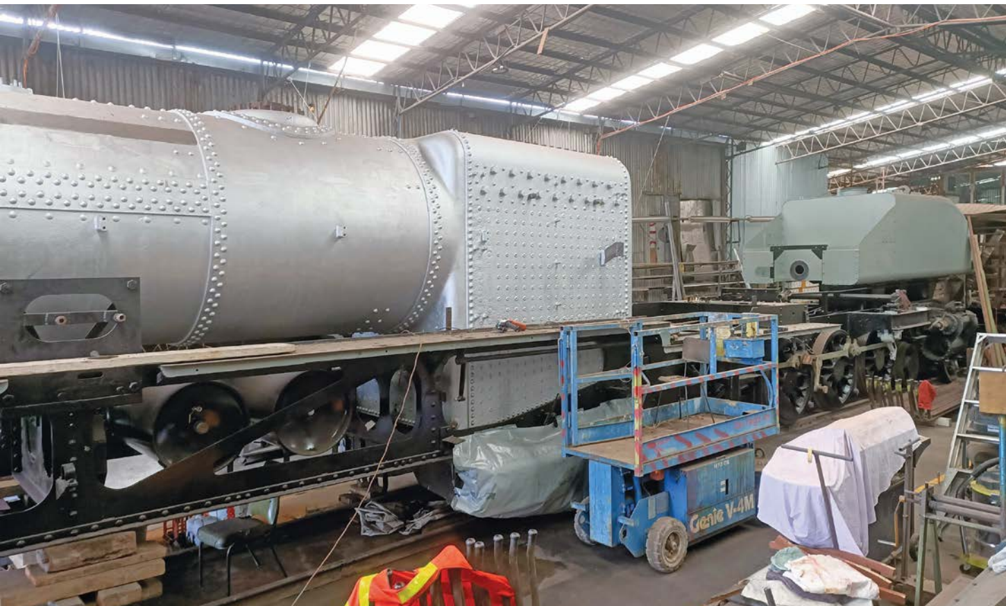
Above: A side view of ASG 33 showing the rear engine unit and boiler cradle under restoration in the Queenscliff workshop of the Bellarine Railway.
