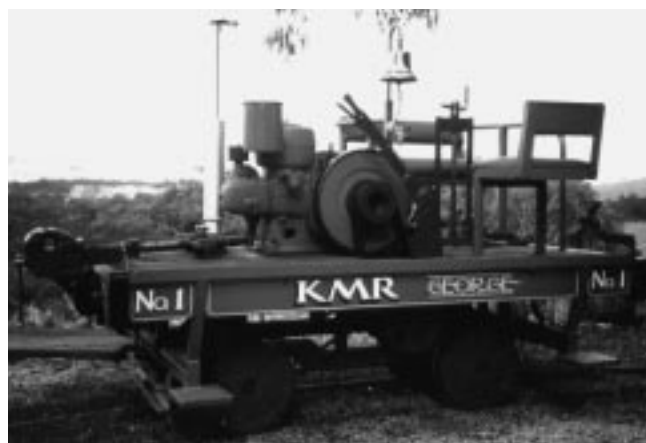
Kerrisdale Mountain Railway - No.1 GEORGE 4wDM built at the railway for construction duties. Photo: Andrew Forbes
