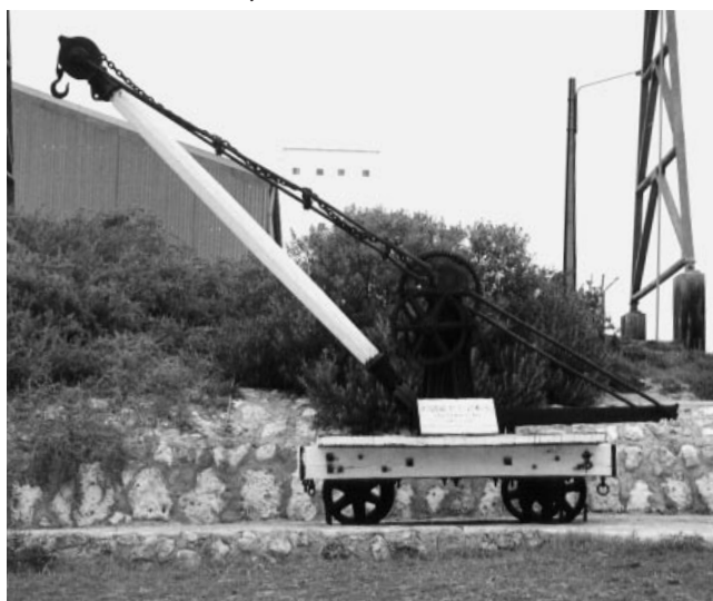
At Thevenard, ships are now loaded by conveyor belt, but this three-ton crane is preserved near the jetty. Until 1969, the crane was in use at Denial Bay.
