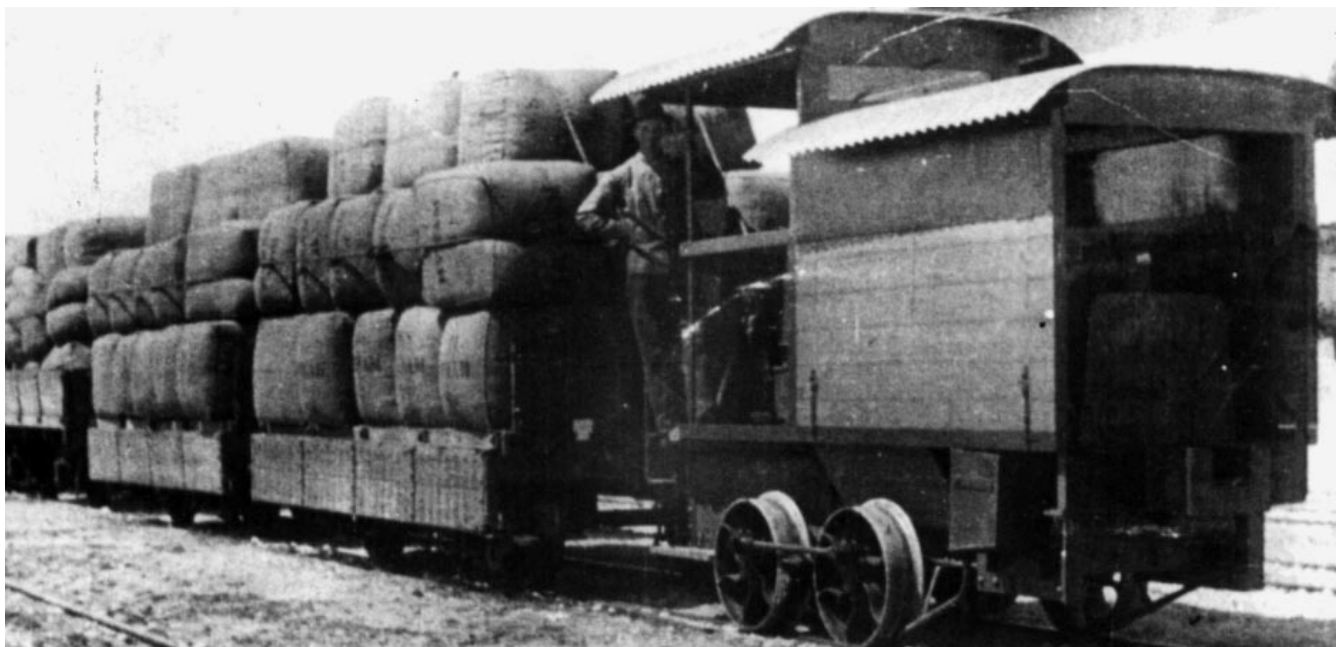
Internal Combustion Locomotive, built by A.H. McDonald & Co. Engineers of Richmond, Victoria (Imperial Engine Works). In 1914 purchased by Dalgety & Co. Ltd for use on the jetty at Kingston SE. Driver on the footplate is Syd Pincher and the trucks are South Australian Railways, with wool brought to Kingston from Hynam to be shipped overseas. Photo: K.Neal McDonald, from A.D. Lockyer collection
