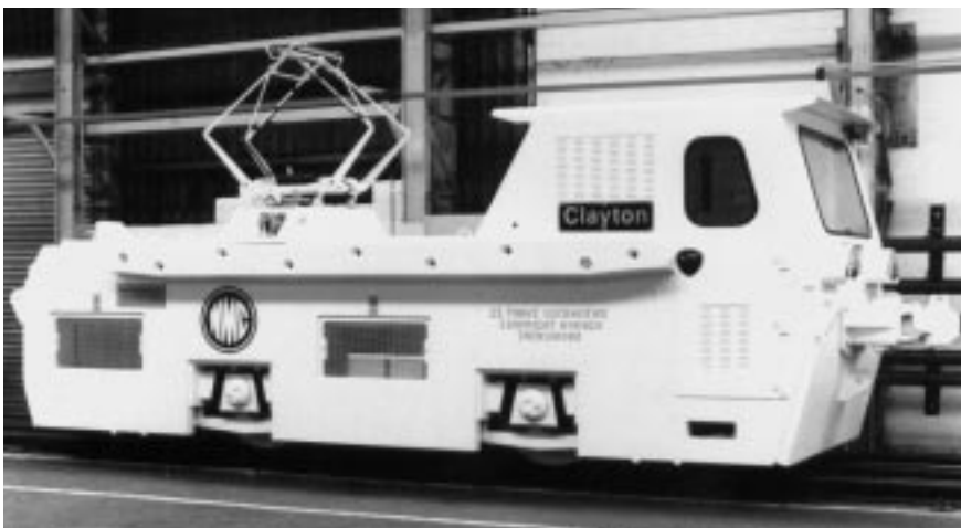
Clayton Equipment 914mm gauge 4wWE 2820LM1002 (B4231B of 1998) for Western Mining Corporation, Olympic Dam project, photographed at the builder's works.
