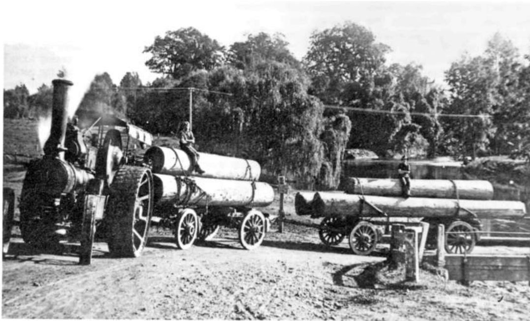
A Fowler 10hp steam traction engine hauling pine logs from Glenniffer in the early 1920s. The driver is Wal Wilkinson. Photo: Mrs Toms, per VA Lovell
