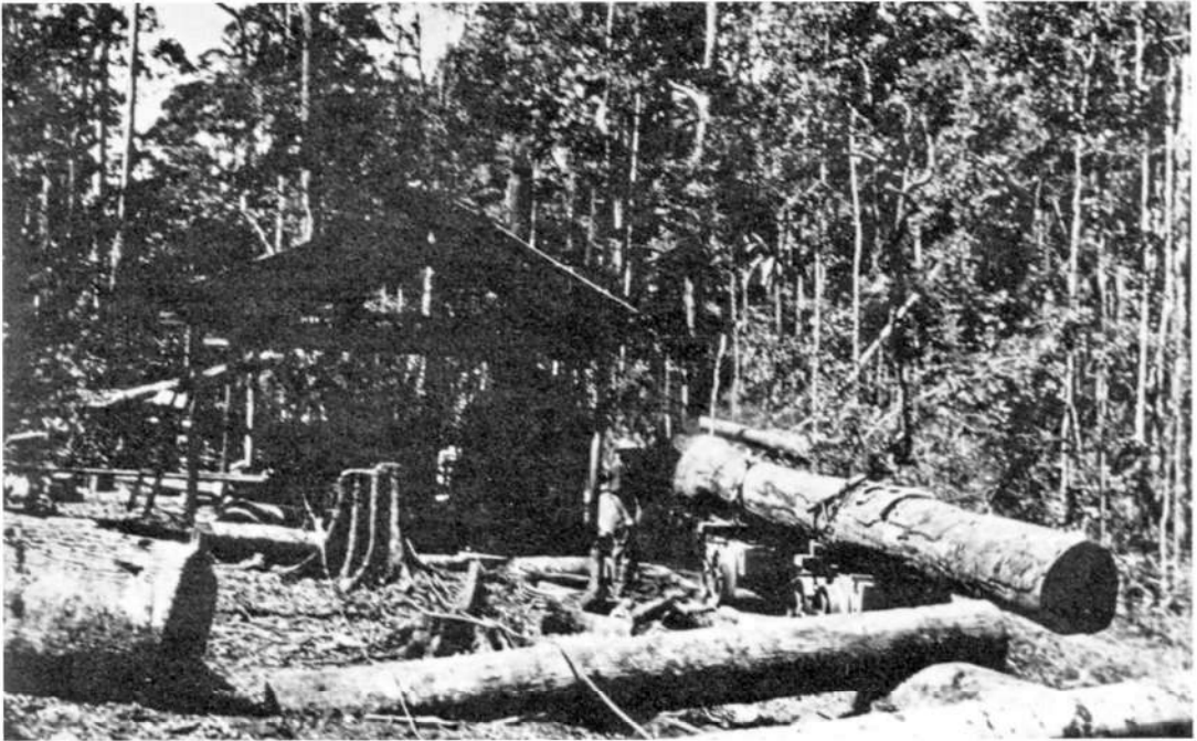
Steam hauler on Eades & Co tramway, September 1930. A brush box log is on the truck for horse haulage to the mill. Photo: FM Bailey, per Forestry Commission of NSW
