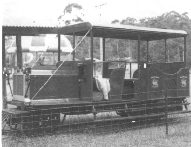
Bob Gough's photo of the Holden-engined 2ft gauge railcar at Tanawha World on the Queensland Sunshine Coast.
