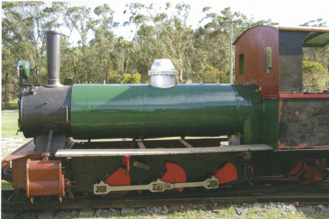
...and a Lick of Paint. Well, actually, three coats of multi-part epoxy provide an acceptable finish to the boiler cladding. The cab is back and the side rods again in place. Photo: Grahame Swanson
