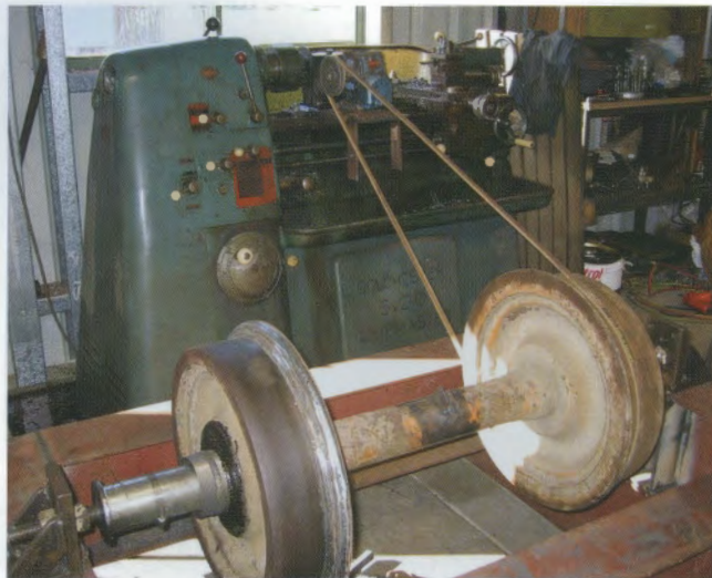
Improvisation - the name of the game when undertaking such a large project in a home workshop. Here the Colchester lathe drives the pony truck wheels while the flanges are reconstructed. Note the reduction gearbox to provide extra slow speed for metal deposition. Photo: Grahame Swanson
