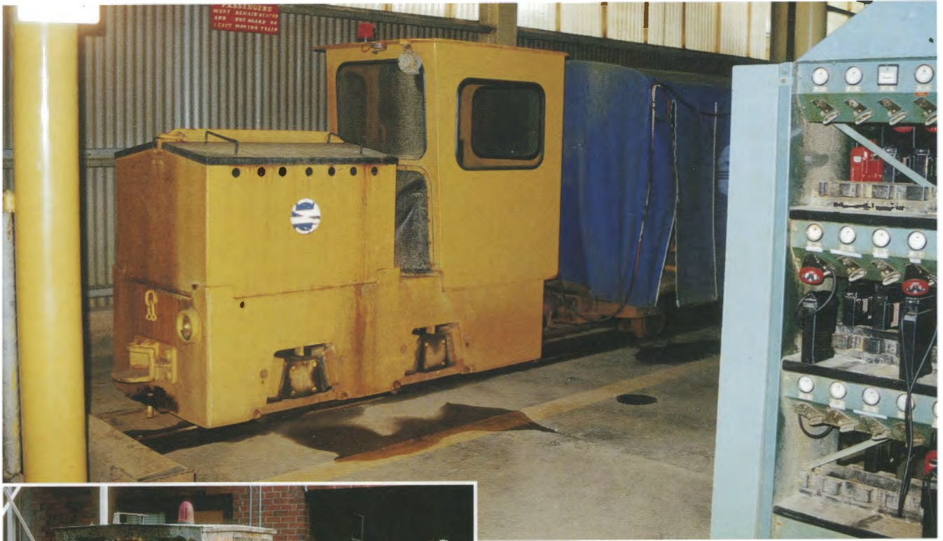
Gemco 5.5-tonne loco charging its batteries on the charge house road while attached to the transport train. Much smaller batteries, those for the miner's lamps, are in their charging racks on the right. 17 September 2002. Photo: Author □ A very work-stained 10-ton Gemco stands outside the charge house on 7 Level in 1980. The open truck behind the loco was probably to match couplings. Granby Willisons were higher than the couplers on the transport cars. Photo courtesy M Dix □ Right angle crossing on the 7 Level main line with building covering the transfer pass down to 8 Level on the right, 1988. Photo courtesy M Dix
