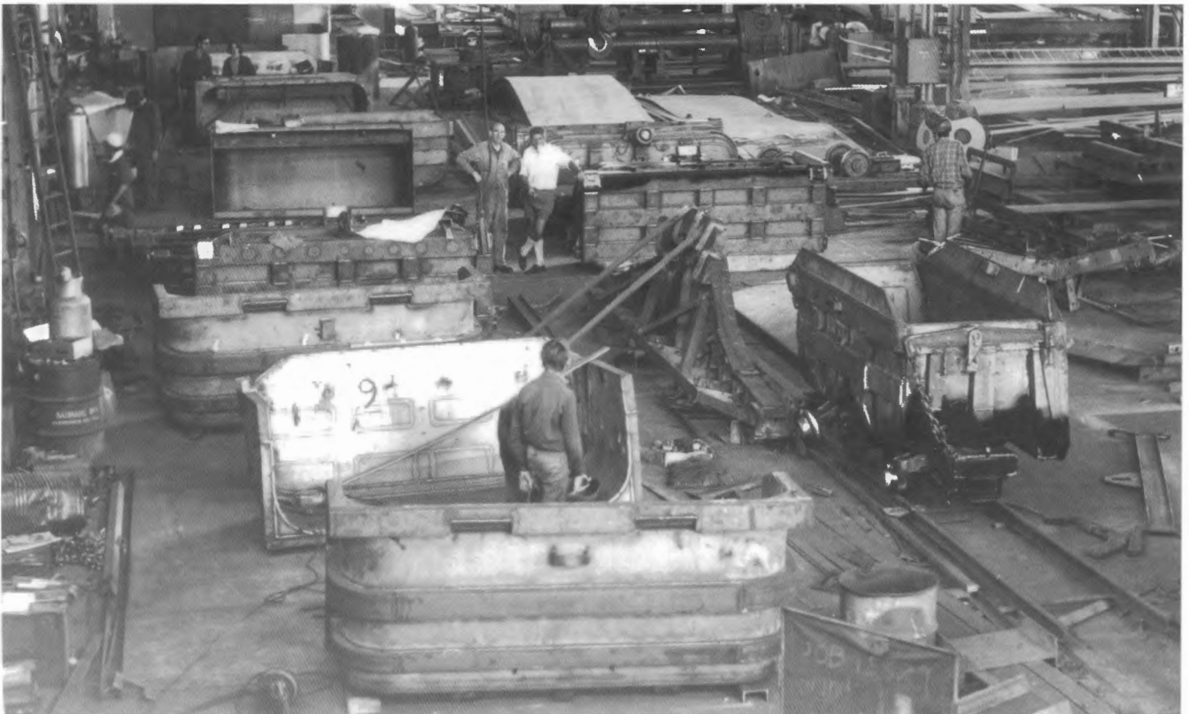
Rosebery's Granby cars under construction at Phoenix Foundry, Launceston. Note the Granby tipping ramp for trial purposes behind the completed car on right. Photo: L Johnson Collection
