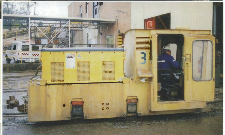
Gravel bin on 7 Level with Granbys in the siding. Cutting through the trees on the right is the route of the aerial ropeway to Williamsford. 1988. Photo courtesy M Dix □ No.3 outside the charging room in 1995. Note the Willison coupler arrangement to match the Granbys. The cab has now been extended and fitted with sliding doors on each side. Photo: L Johnson Collection □ 10-ton Gemco No.1 as rebuilt, shunting fuel tank trucks on 7 Level. Photo: L Johnson Collection
