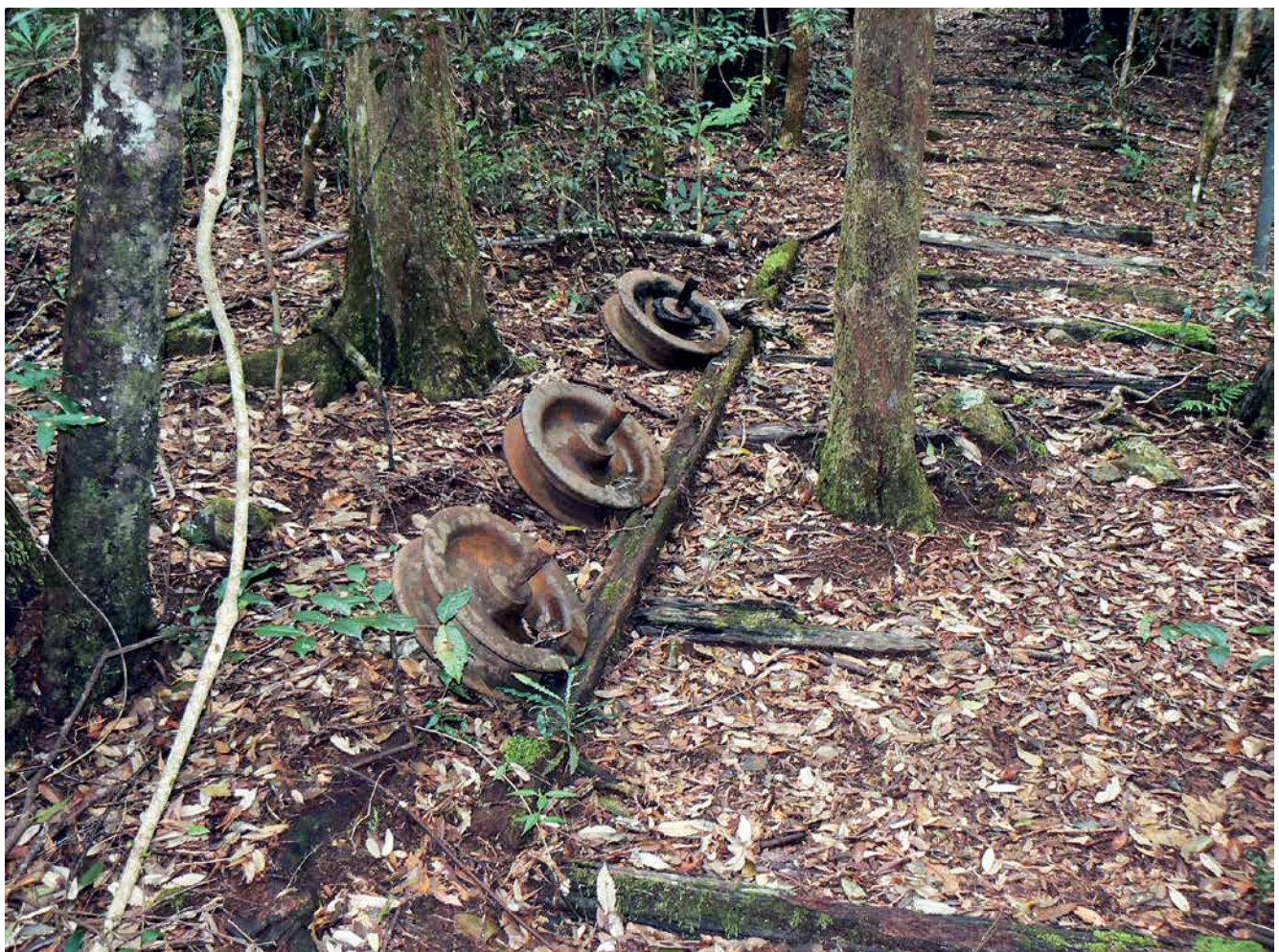
380mm diameter cast iron pulley wheels posed on remnant brush-box rail on the upper section of the Gleniffer Incline Tramway. These pulley wheels were attached to convenient tree trunks and posts beside the tramway to guide the return wire to the steam winch. Photo: Ian McNeil
