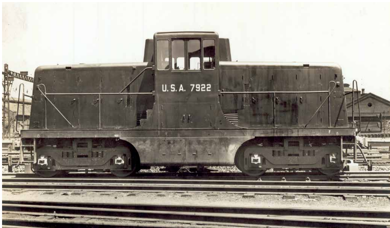
General Electric 44-ton locomotive no.7922, photographed on 17 January 1944. It is still in original condition. The cab did not fit within the New South Wales Railways rolling stock gauge and had to be modified. It is also fitted with automatic couplers, which were replaced by hook and buffers by the New South Wales Railways, but automatic couplers were again fitted by the Commonwealth Railways.
