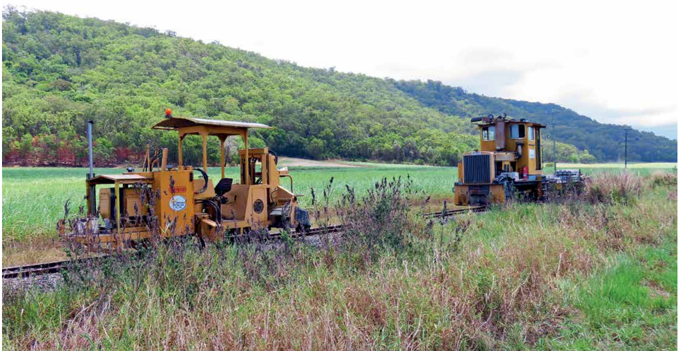
Mossman Mill's Com-Eng 0-6-0DH Mossman (B1719 of 1957) and the Gemco sleeper renewer (R854 of 1987) on re-sleeper duties alongside the Cook Highway on 1 November. Photo: Gregorio Bortolussi
