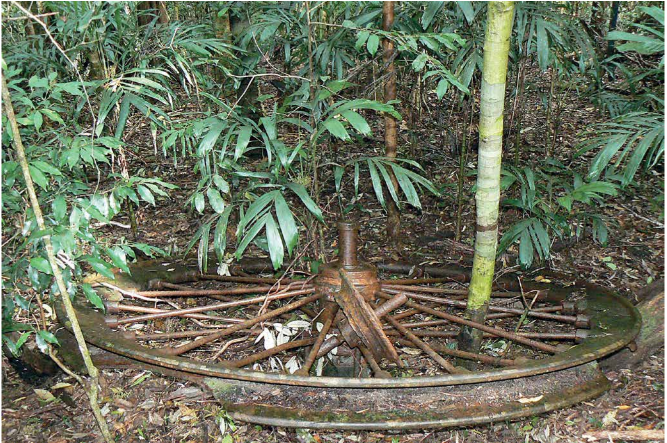
The cracked remains of the old 7ft diameter bull wheel are still in situ at the upper terminus of the incline tramway. The wheel originally graced the poppet-head of a colliery, and features twin hubs each mounting twelve one-inch diameter spokes.
