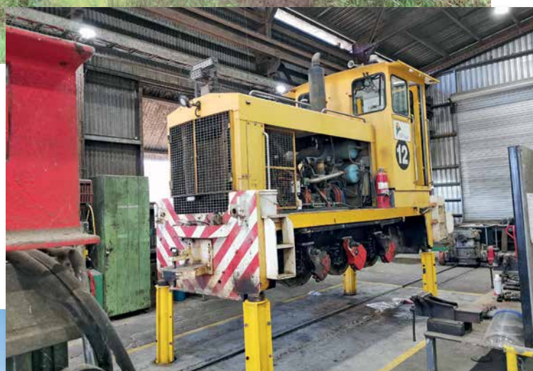
Above: On 23 October, Mossman Mill Com-Eng 0-6-ODH multi-unit locos Ivy (AL4181 of 1965) and Cook (AL3372 of 1964) at Cassowary Creek with the last rake of fulls from Killaloe for the 2019 crushing season. Photo: Gregorio Bortolussi Right: South Johnstone Mill's Clyde 0-6-ODH 12 (55-60 of 1955) jacked up in the loco shed with its final drive removed on 12 November. Photo: Jason Sou Below: Mulgrave Mill's Com-Eng 0-6-ODH 26 Meringa (AK3675 of 1964) prepares to pull fulls out of a siding along Parry Road on 19 November while Clyde 0-6-ODH 19 Redlynch (65-435 of 1965) hovers in the background and the harvester cuts cane in the adjacent paddock. Photo: Gregorio Bortolussi
