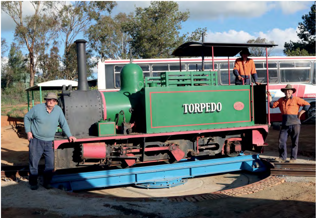
Hunslet Torpedo 1187/1915 on the newly constructed turntable. Peter Neve is standing at the front of the locomotive while Josh (in cab) and his father, Phil Burke who were responsible for the design and construction of the turntable and pit stand at the rear on 5 September 2020. Photo: Peter Neve Collection
