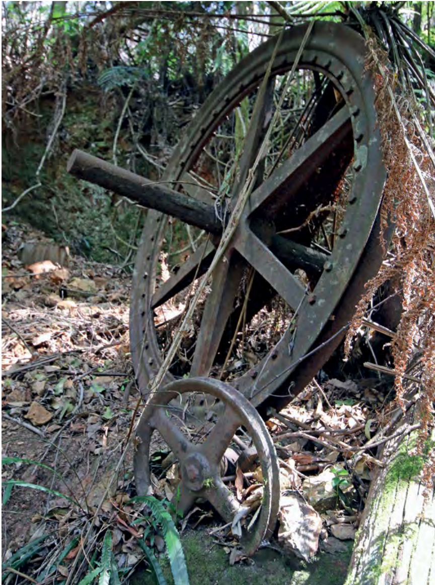
Terminating wheel and idler wheel at the Bumbo Creek battery site. Both show signs of rope wear. Photo: Phil Cleaver
