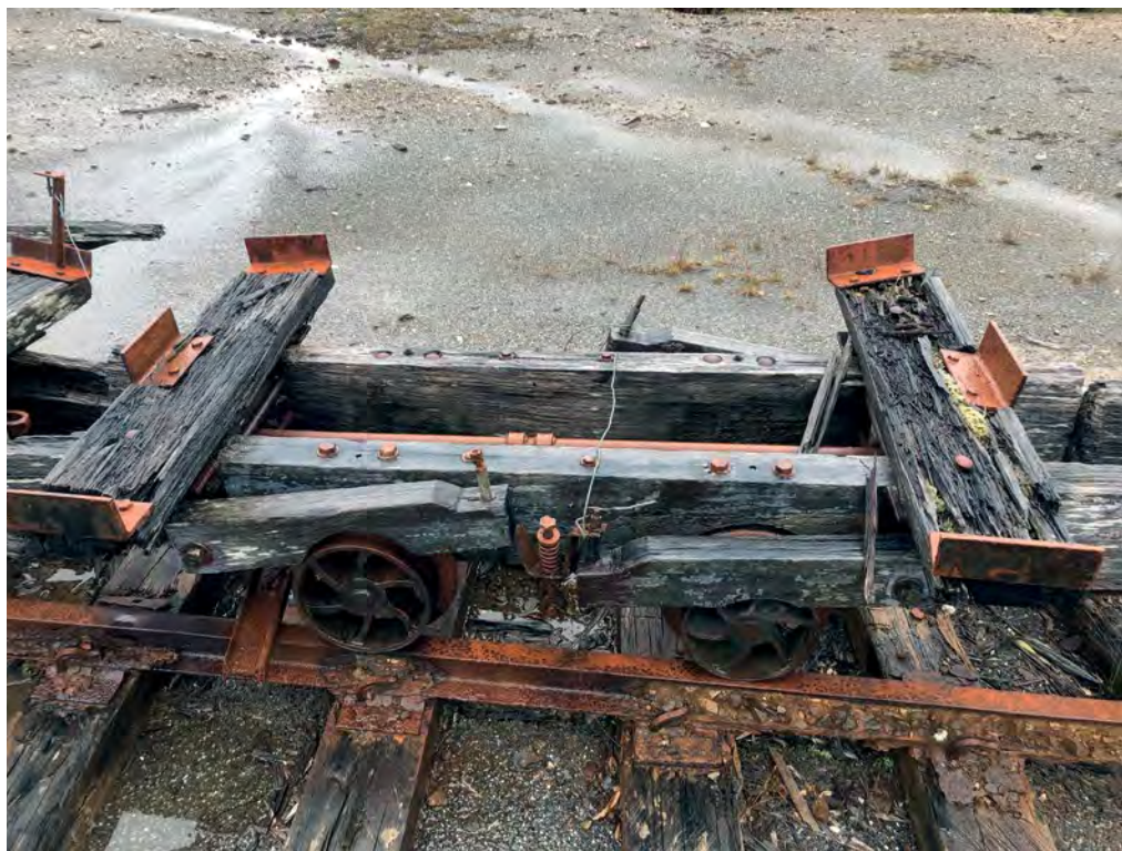
Also at Tullah on 4 October were three limestone trolleys from the Ida Bay Railway, perhaps the only intact examples left anywhere of these wagons, which feature a unique inertia braking system. Photo: James Shugg
