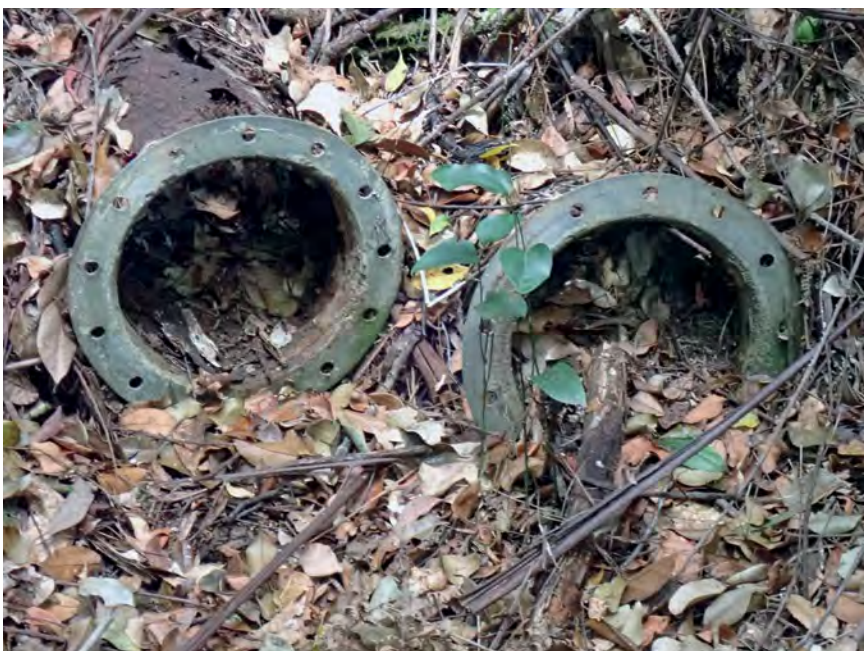
Flanged piping at the battery site hinting at the use of water power to drive the ore processing machinery. Photo: Rob Lees
