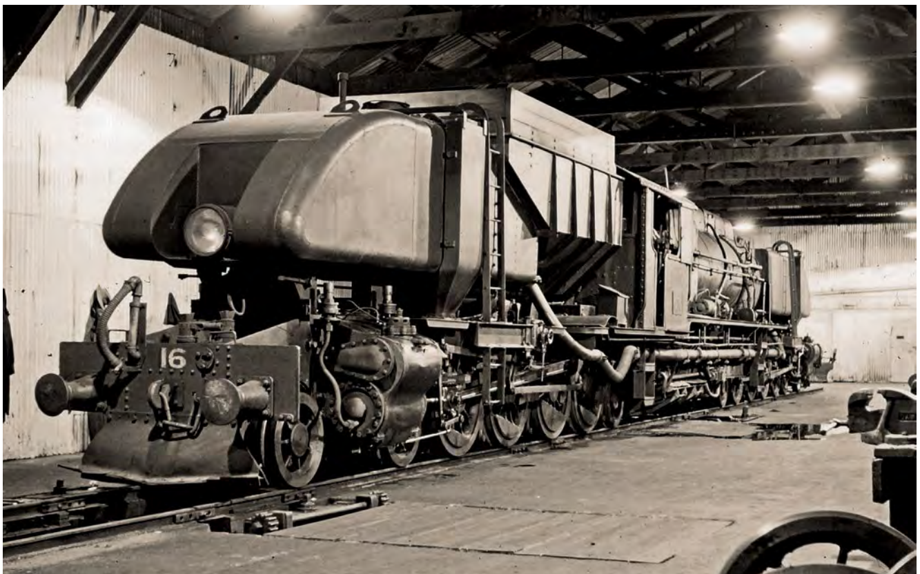
Stylish from all angles. EBR No.16 Burnie locomotive shed 28 January 1963 – a wonderful photograph inside a very clean shed at night. The ASG was designed in Melbourne by the Commonwealth Land Transport Board under lead designer Frederick Mills, the WAGR CME on secondment. The first rolled out of the shops just twelve months after design work started – a major achievement considering the more than 100 separate sub-contractors involved. The actual locomotives were assembled in WA, SA, Victoria and NSW. No.16 had been assembled at the SAR's Islington Workshops in Adelaide in August 1944. It quickly entered service with the Queensland Railways only to be withdrawn in September 1945, when the war ended. The EBR, sensing a bargain (and being cash-strapped) obtained G16 in 1950, did the necessary modifications and put No.16 to work in mid-1952. Photo: Weston Langford www.westonlangford.com/images/photo/102483 (Colour changed to B&W)
