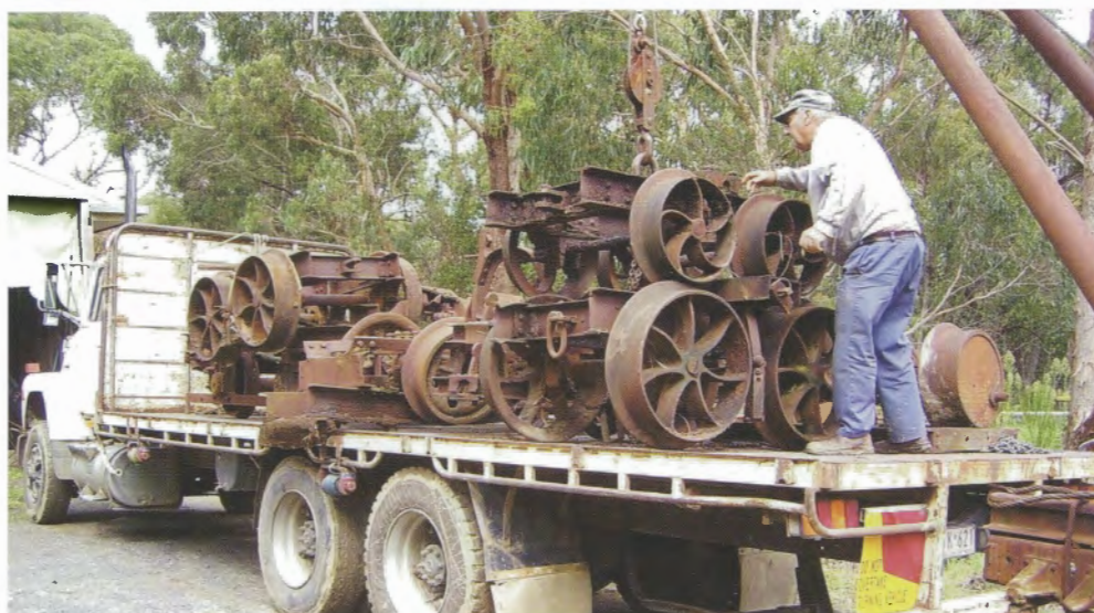
Loading the 3ft gauge steel frames log bogies at Belgrave South on 8 April 2006 for transport to the Alexandra Timber Tramway & Museum.
