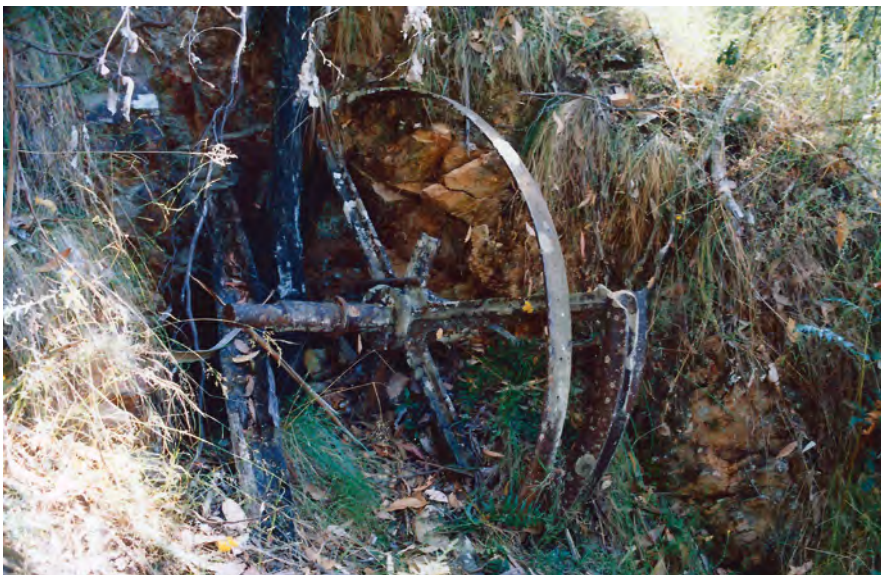
Above: Lowering gear brake band, No.3 level lowering gear site. From the numerous drilled holes and remnant fastenings it can be assumed that the brake band was lined with segmented material, probably wood. Photo: Peter Evans
