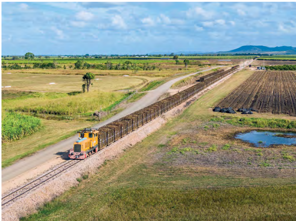
Below: Pioneer Mill's Clyde 0-6-0DH Colevale (65-438 of 1965) passes by Payards 2 with a load of fulls from Sexton Road on 31 July. Photo: John Kirk
